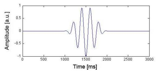
Figure A.2: Source pulse employed to excite surface waves inside our cavity.
