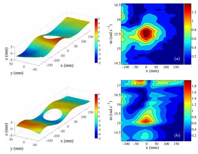
Fig. 2: Typical instantaneous fields of the surface elevation  $h_T(x, y, t)$ , here for a/d = 0.50, kd = 1.32. The scale of the colorbar is in mm.
