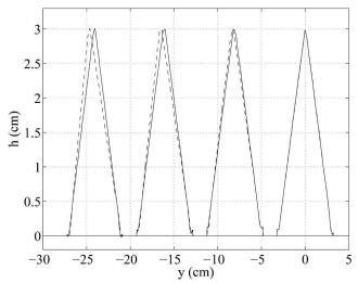
Fig. 10. Height reconstruction h(y) for various  $y_0$  values. Solid curves correspond to our phase-to-height relation and dashed curves correspond to Takeda's phase-to-height relation. The experimental configuration is the same as in Fig. 9.
