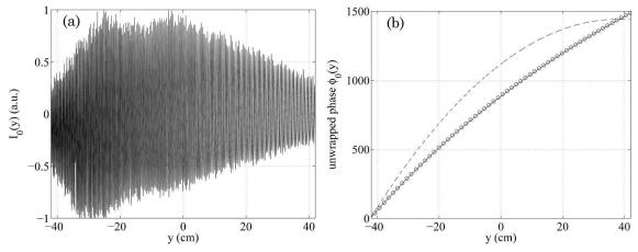
Fig. 8. (a) Intensity variations  $I_0(y)$  for fringe projection onto the reference plane in the absence of the triangular prism and (b) the corresponding unwrapped phase  $\varphi_0(y)$  (see [23]). Experiments correspond to  $\theta = 33.9^\circ$  with L = 105.2 cm. The points are the experimental data (only one point of each 150 points is indicated for visibility), the solid curve corresponds to our Eq. (2.12) and the dashed curve corresponds to Eq. 2.13 from [12,13,20].
