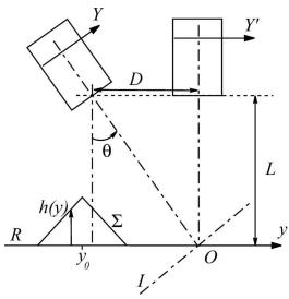
Fig. 5. Experimental configuration:  $\Sigma$  is at distance h(y) from the reference plane R with  $h(0 < y - y_0 \le -3 \, \mathrm{cm}) = y$ ,  $h(0 < y - y_0 \le 3 \, \mathrm{cm}) = -y$  zero, otherwise. I is the image plane of the projector. In the experiments,  $L = 105.2 \, \mathrm{cm}$  and  $\theta$  can vary, and for  $\theta = 0^{\circ}$  (parallel-optical-axes geometry),  $D = 18 \, \mathrm{cm}$ .
