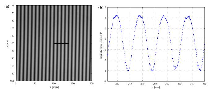
Fig. 3 a Sample image of the fringes projected onto an undeformed liquid surface as registered by the camera. b Intensity profile along the horizontal segment shown in *black* over the image a
