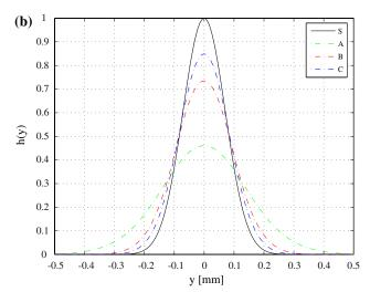
$s/p = 10^{-1}$  over each curve in the **a**, compared to the original gaussian profile (shown in *black*). *Color* correspondence between curves in both panels has been conserved for reference purposes. Note that **b** shows a bad-case scenario to illustrate the influence of the filter width on the quality of the reconstruction; however, in practice, a set of parameters ensuring an error less than  $10^{-4}$  % was used
