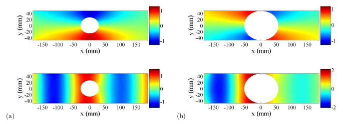
Fig. 4: Experimental patterns of the two trapped modes, and the associated even parts. (a) even and odd fields of the linear field  $h_1(x, y)$ , for a/d = 0.40 and kd = 1.46. The even part exhibits the form of the trapped mode localized in the vicinity of the cylinder. (b) Same representation for a/d = 0.95 and kd = 1.51. The scale of the colorbar is in mm.
