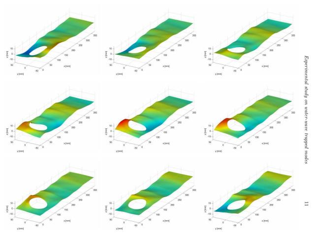
Figure 4: Experimental measurements of the instantaneous total free-surface deformation fields. The figure shows a time-sequence of the evolution of the free surface deformation fields for a particular case of the aspect ratio explored, namely a/d=0.5. The wave's incident frequency corresponds to f=2.5 Hz. Frames are separated by  $\Delta t=0.04$  s.
