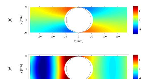
Figure 11: Experimental patterns of a second kind of trapped modes and their associated symmetric part. Panels (a-b): symmetric and antisymmetric fields of  $h_1(x, y, t)$  for a/d = 0.95 and kd = 1.51 (f = 2.62 Hz). The position of the obstacle is indicated by the black circle. The scale of the colorbar is in mm.
