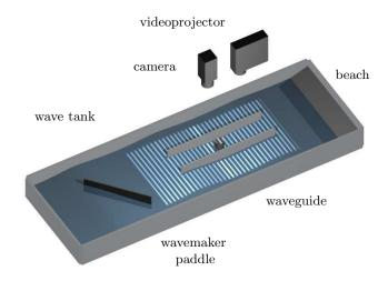
(a) scheme of the complete experimental setup
