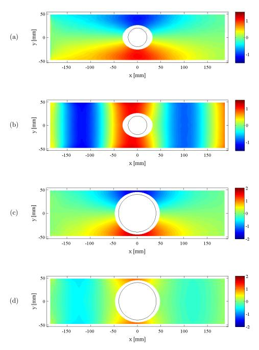
Figure 10: Experimental patterns of the trapped modes and their associated symmetric parts. Panels (a-b): Symmetric and antisymmetric fields of  $h_1(x, y, t)$  for a/d = 0.4 and kd = 1.46,  $(f = 2.50 \, \text{Hz})$ . Panels (c-d): Same representation for a/d = 0.80 and kd = 1.33  $(f = 2.40 \, \text{Hz})$ . The position of the obstacle is indicated by the black circle. The scale of the colorbar is in mm.
