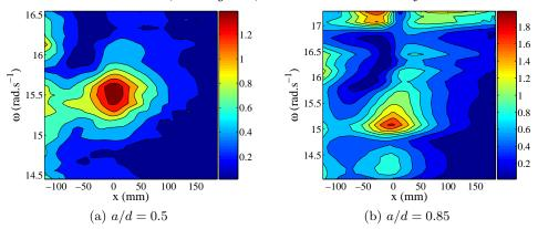
Figure 5: Experimental evidence of the trapped mode resonance:  $^{1}/_{2} \cdot [h_{T}(x, y, t) - h_{T}(x, -y, t)]$  for some fixed (y, t) is displayed in color scale as a function of x and  $\omega$ . (a) For a/d = 0.5, one resonance is visible near the cylinder, (b) for a/d = 0.85 in addition to the first resonance a second maximum near the cut-off frequency can be seen. The cylinder lays at x = 0 mm (configuration I). The scale of the color bar is in mm.
