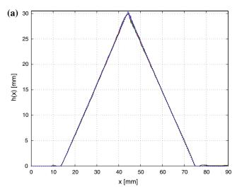
**Fig. 5 a** Several height profiles measured for the triangular prism used for laboratory testing. **b** Zoom over a portion of the reconstructed profiles showing the precision of the method. In both cases, *dots* indicate the object's profile measured by a 25- $\mu$ m resolution (point) laser displacement sensor, whereas continuous lines
