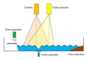
Fig. 2 Complete experimental setup
