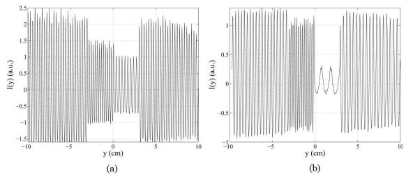
Fig. 7. Intensity variations I(y) in (a) the parallel- and (b) the crossed-optical-axes geometries. The curves correspond to the averages over the x direction of the 3D plot in Fig. 6.
