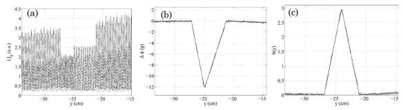
Fig. 9. (a) Signals  $I_0(y)$  and I(y) for fringe projections on the reference plane R and on the  $\Sigma$  plane. (b) Unwrapped phase difference  $\Delta \varphi(y)$  and (c) reconstructed height h(y) using Eqs. (2.9) and (2.11). The experiment is conducted in the parallel-optical-axes geometry with  $L=105.2\,\mathrm{cm},\,D=18\,\mathrm{cm},\,\mathrm{and}\,y_0=-24\,\mathrm{cm}.$
