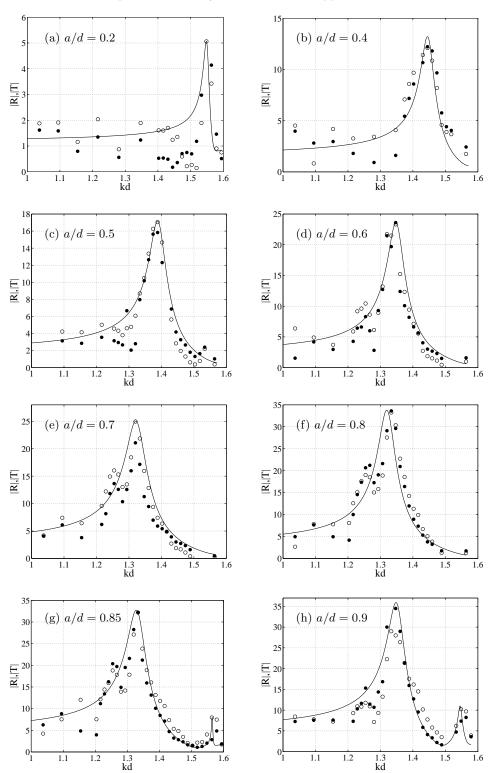
Figure 15: Resonance curves for several values of the aspect ratio a/d considered in this study. Full circles: reflection coefficient R; open circles: transmission coefficient. The continuous line represents the fit of the experimental data (see text for details).
