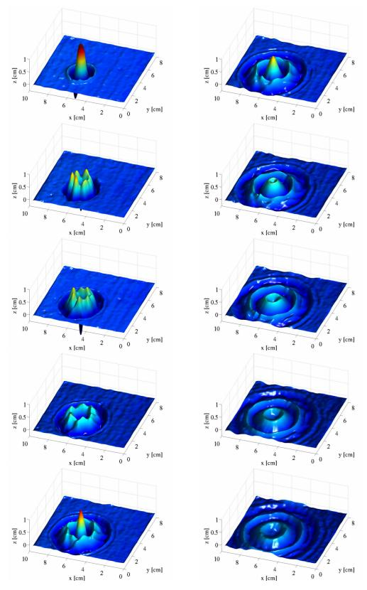
Figure A.4: Experimental measurements of a drop impact onto a thin liquid film of the same fluid. In this series of snapshots, time evolves columnwise from top to bottom and from left to right. The liquid surface shown in these figures is sampled at a resolution of  $800 \times 1000 \, \mathrm{px}^2$ , using a high speed camera. [See text for further details.]
