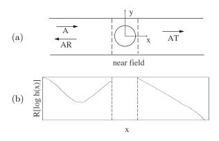
Fig. 5: Top: The problem reduces to a 1D problem along the x-axis, by projecting the odd field onto the first transverse mode in  $\sin \pi y/2d$  outside the near field region. Bottom: Typical variation of the measured h(x) along the x-axis: real part of  $\log[h(x)]$  as a function of x (a.u.) (the curve has been obtained for a/d = 0.4, kd = 1.47).
