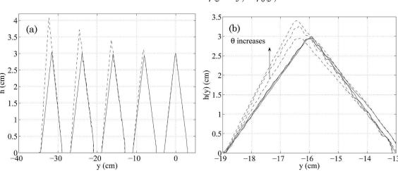
Fig. 11. Reconstructed height h(y) in the crossed-optical-axes geometry (a) for  $\theta = 33.9^{\circ}$  and varying the  $y_0$  position of the triangle and (b) for  $y_0 = -16$  cm and varying  $\theta = 0$ , 18.1 and 41°. Solid curves correspond to our height reconstruction from Eq. (3.3) with Eq. (1.2). Dashed curves are the height reconstructed using Takeda's relation Eq. (1.1).
