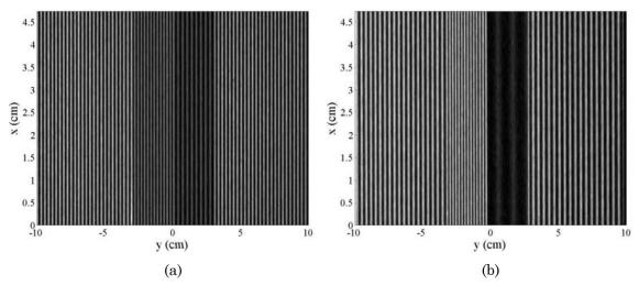
Fig. 6. Experimental intensity variations I(x,y) captured by the camera (a) in the parallel-optical-axes geometry with  $D=18\,\mathrm{cm}$  and  $L=105.2\,\mathrm{cm}$  and (b) in the crossed-optical-axes geometry with  $D=70.7\,\mathrm{cm}$  ( $\theta=33.9^\circ$ ),  $L=105.2\,\mathrm{cm}$ , and  $y_0=0$ .
