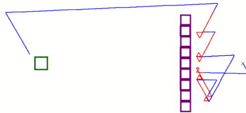
Figure 7.12: Example of obstacle avoidance. The cross is the start point of the robot, the violet squares are obstacles, and the green square is the target. The red trajectory is where the CNN orbit is controlled inside of eight-dimensional (12345678), while the blue trajectory is inside of the four-dimensional invariant subspace whose corresponding moving range covers the target direction. Modulus 4 is used for external input period.
