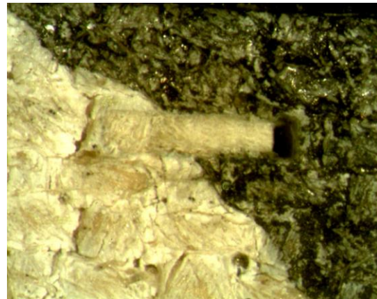
Figure 84 : élimination de PVAc, \lambda=248 nm, \tau = 10 ns
