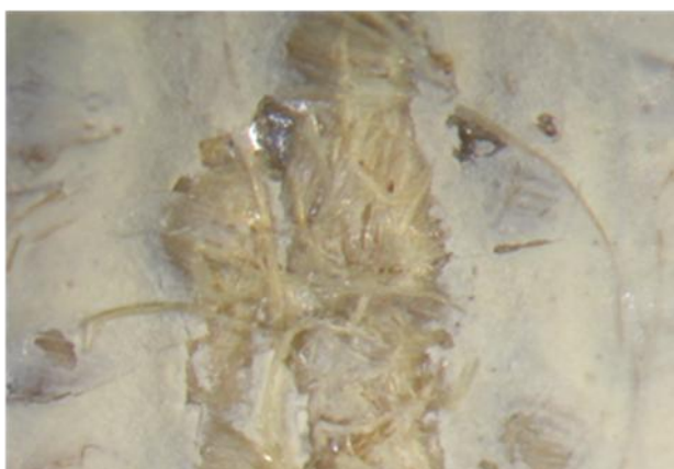
Figure 130 : élimination de la cêruse, \lambda : 532 nm, F = 1,87 J/cm 2 .5 pulses, Ablation +++
