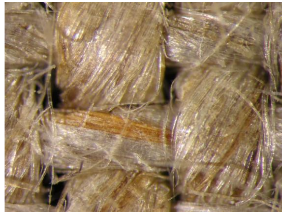
Figure 73 : Nd:YAG; Q=258 mJ; \lambda=532 \text{ nm} , \varnothing=7 \text{ mm} , H=25 cm, \tau 8\text{ns}
