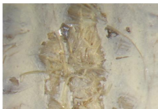
Figure 130 : élimination de la cêruse, \lambda : 532 nm, F = 1,87 J/cm².5 pulses, Ablation +++
