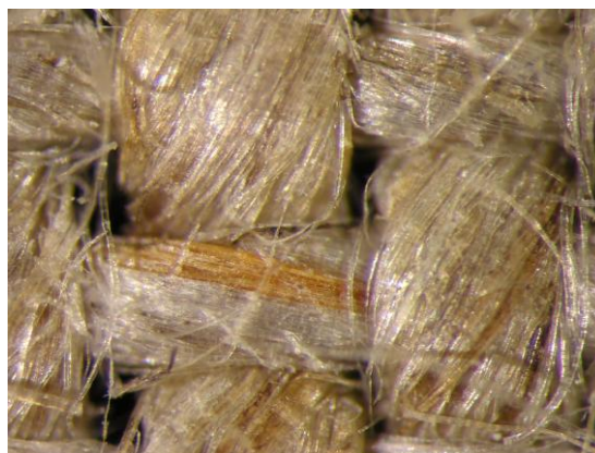
Figure 73 : Nd:YAG; Q=258 mJ; \lambda=532 nm, \varnothing=7 mm, H=25 cm, \tau 8ns
