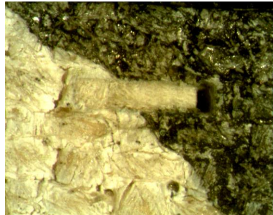
Figure 84 : élimination de PVAc, \lambda=248 nm, \tau = 10 ns
