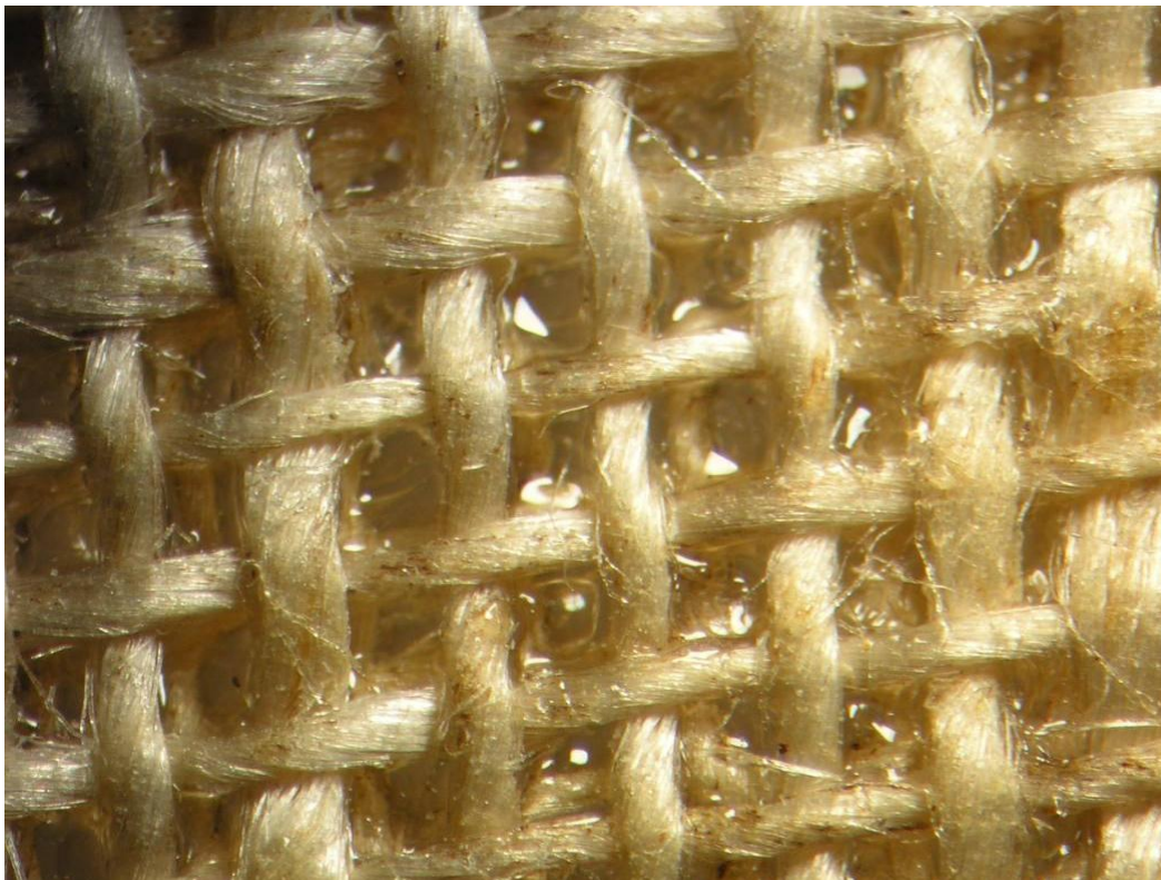
Figure 146 : élimination de la Mowilith® DMC2, \lambda : 248 nm, F = 1,12 \text{ J/cm}^2 .40 pulses, Ablation +++
