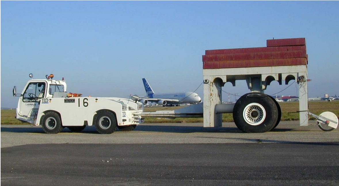
**Fig. 0-13** STAC's A<sub>340</sub> two-wheel landing gear loaded at 25 tons (250 kN) per wheel here trailed by the Airbus truck on the HTPT test facility (Photograph by D. Guédon, Toulouse LRPC)
