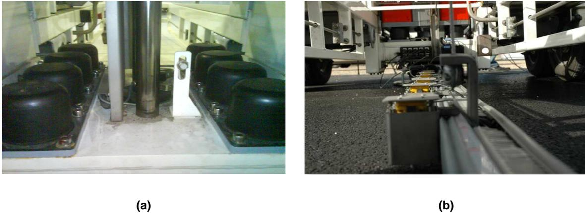
**Fig. 1-2 a- The HWD buffer system, b- The geophones**
