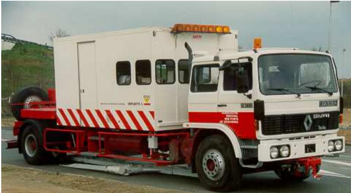
Fig. 0-15 The Lacroix Deflectograph (source: LCPC's database)
