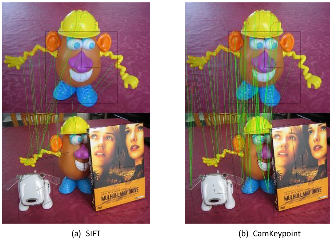
Figure 2-15: Comparisons between SIFT and CamKeypoints: note that the number of points matched between the interest points of two images extracted by SIFT is relatively small compared to the number of points extracted by CamKeypoints. We try to detect the same number in both cases by changing the threshold.
