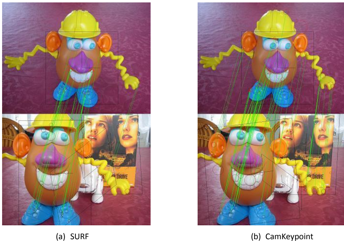
Figure 2-16: Comparisons between SURF and CamKeypoints we note that the number of points that match between the interest points which extracted by SURF is relatively small compared to the number of points extracted by the CamKeypoints. We try to detect the same number in both cases by changing the threshold.
