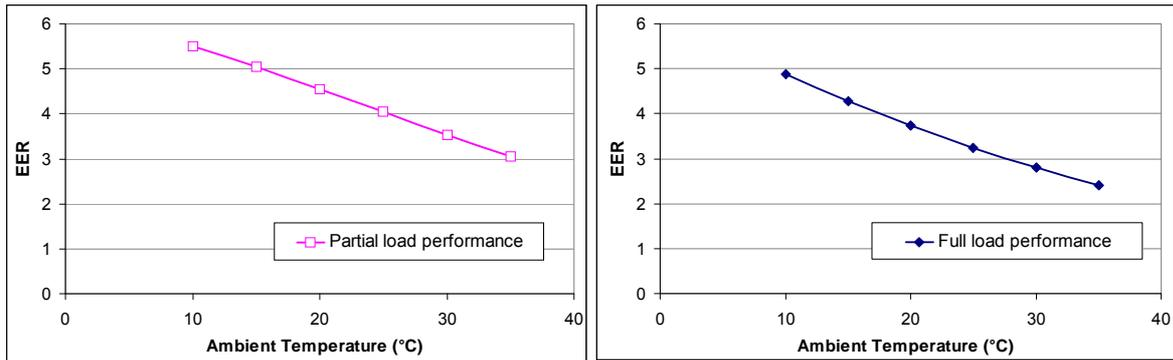
Figure 12: Cooling mode performance at partial load (left) and full load (right)
