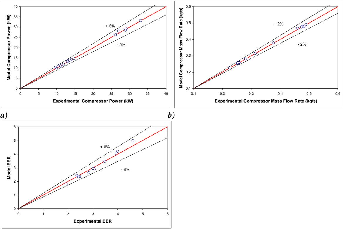
c) *Figure 10: Comparison between model and experiments results in cooling mode*
