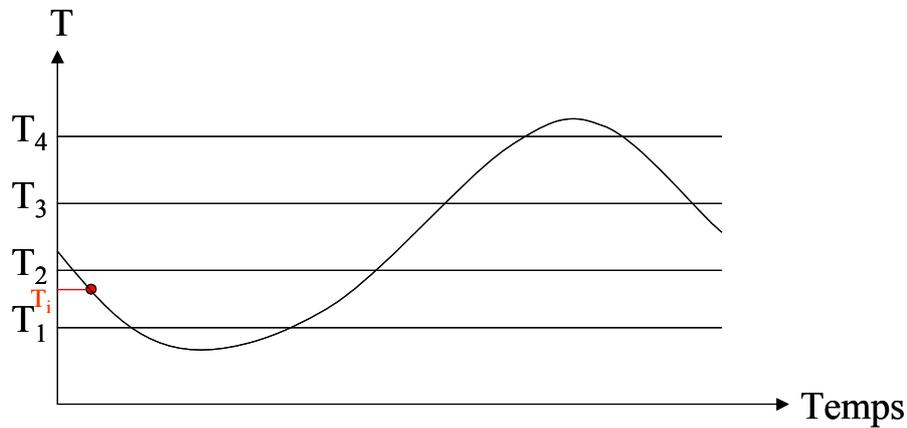
$$\begin{aligned} d_i^2 &= \frac{T_i - T_1}{T_2 - T_1} \\ d_i^1 &= \frac{T_2 - T_i}{T_2 - T_1} \end{aligned}$$
