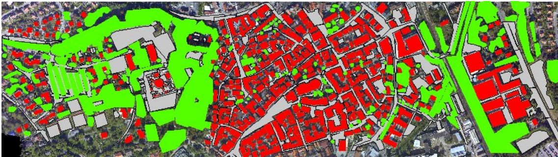
(a) Defining the ground truth with manually selected 2D polygons (full area of Biberach).
