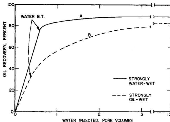
Figure 1.9: Typical waterflood performance in water-wet and oil-wet sandstone cores at moderate oil/water viscosity ratios [107].
