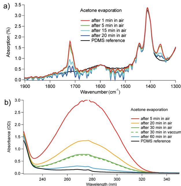
**Figure 4.** (a) FTIR-ATR spectra around the acetone absorption band ( $1715 \text{ cm}^{-1}$ ) showing an acetone-imbibed PDMS sample and acetone evaporated from the surface layer over time. (b) UV absorption spectra of an acetone-imbibed PDMS sample showing vanishing acetone concentration from bulk PDMS over time.
