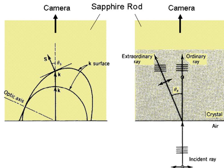
Figure C.28: Double refraction at normal incidence [229].
