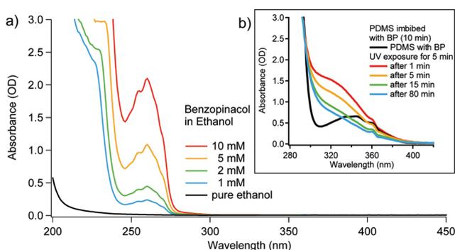
**Figure 8.** (a) UV absorption spectra of benzopinacol dissolved in ethanol. (b) UV absorption spectra of PDMS imbibed with BP before and after UV treatment. The spectral series shows the appearance and evolution over time of the intermediate species In with characteristic absorption at around 320 nm.
