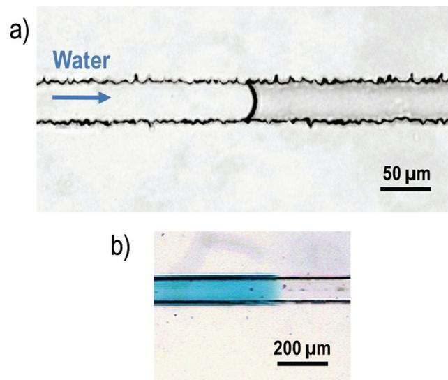
Figure 2.9: PDMS microchannels. (a) Water is injected in a  $40 \times 40 \mu\text{m}^2$  channel in a PDMS chip with ‘rough’ walls. (b)  $100 \times 100 \mu\text{m}^2$  channel with partial hydrophilic surface treatment (blue).
