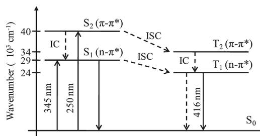
**Figure 2.** Simplified Jablonski diagram of BP ground state ( $S_0$ ) as well as first and second excited singlet ( $S_1$ ,  $S_2$ ) and triplet ( $T_1$ ,  $T_2$ ) states. Excited state energies are indicated in terms of their wavenumber as approximate values. Solid lines indicate radiative transitions, while dashed lines indicate nonradiative transitions. IC and ISC processes are labeled as well.
