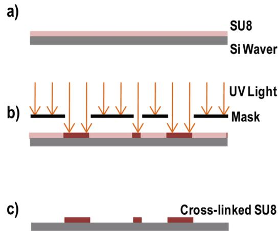
Figure 2.2: Silicon master fabrication process. (a) SU8 photoresist is spun onto a silicon wafer at a desired thickness. (b) Microstructures are transferred to the photoresist by UV exposure through a mask. (c) Developed photoresist provides the microfluidic structures on the silicon master.
