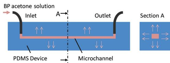
**Figure 6.** Schematic of a simple PDMS device containing a single microchannel. Acetone and BP diffusion into the PDMS matrix during injection is indicated.
