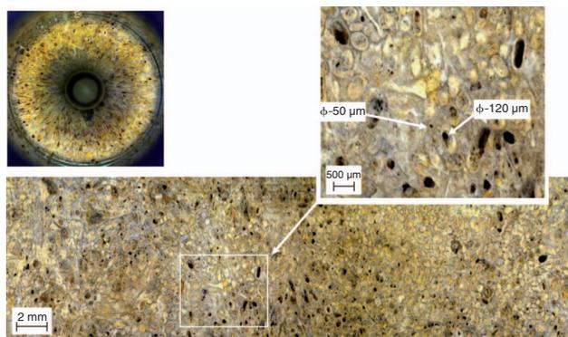
Figure 6. Example of a “digital core” obtained from a rock sample with a strongly heterogeneous pore structure covering about 400 mm<sup>2</sup> of rock surface. One of the raw images as obtained during the digital core-imaging process is shown in the upper left corner. A magnification of a selected area is given in the upper right corner showing grain and pore features as small as a few tenths of microns.
