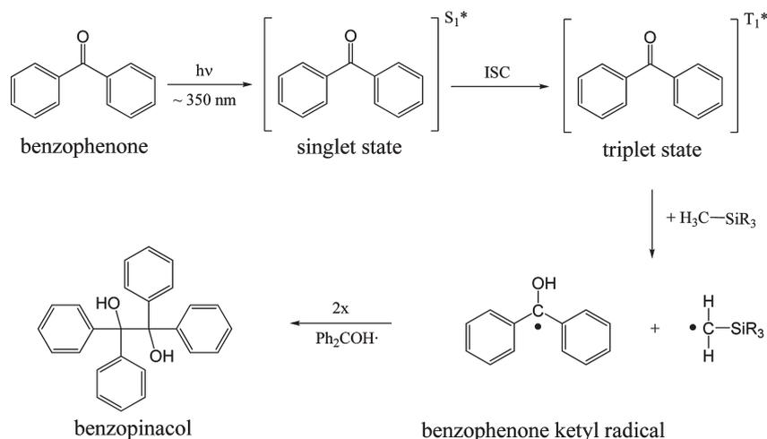
**Figure 1.** Reaction schematic of the dominant pathway for graft photoinitiation with BP: Triplet BP is produced via absorption of a photon and subsequent  $S_1 \rightarrow T_1$  transition via ISC. Triplet BP then abstracts an H-atom from a PDMS methyl-group to form the BP ketyl radical. While the methyl radical can serve as an initiator for AA polymerization, BP ketyl radicals combine with each other to form benzopinacol eventually.
