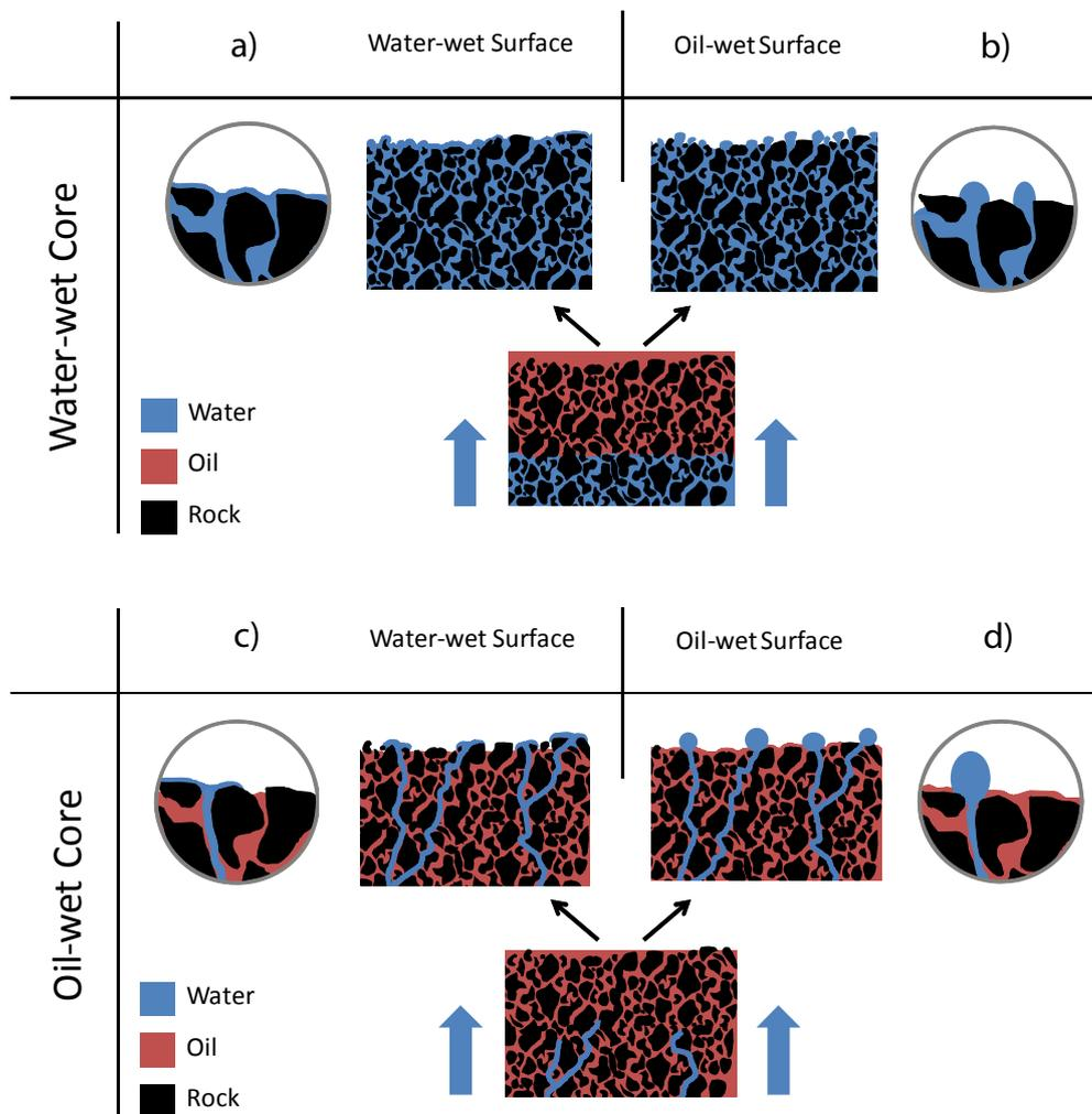
Figure 1: Schematic description of the injection concept: For a particular range of capillary numbers distinct fluid fronts are expected to develop. (a,b) flat fluid front is expected for imbibition, and (c,d) capillary fingering is expected for drainage. Surface wettability causes different behavior upon breakthrough; i.e., spreading over grains (a,c) or droplet formation (c,d).
