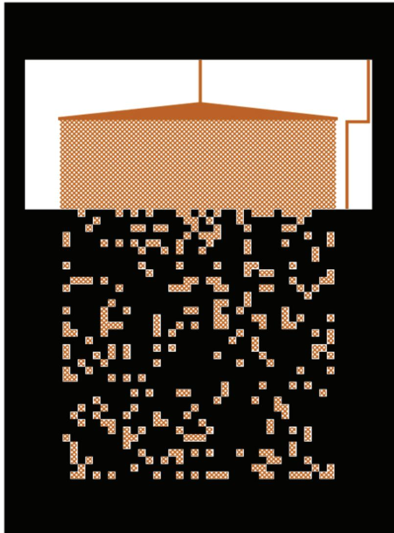
Figure B.4: UV exposure mask designed for wettability patterning with 20% water-wet area ( $f_w = 0.2$ ). The top part of the mask provides a wide opening for full exposure. A micromodel (type I) is schematically shown in the background.
