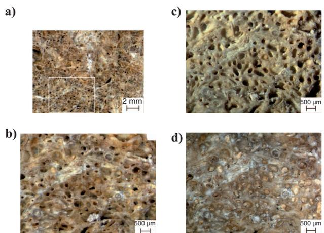
Figure 8. Comparison of rock-imaging techniques. (a) A digital core image obtained with the MGI, and (b) a detail view of the same image. Parts c and d show images of the same rock section as in Part b, obtained with a stereo microscope. Part c shows an image obtained with highly oblique illumination; Part d was obtained with axis-parallel illumination.
