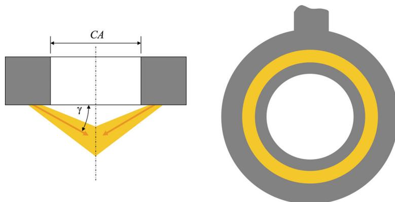
Figure C.10: Ring-light guide for angular illumination.
