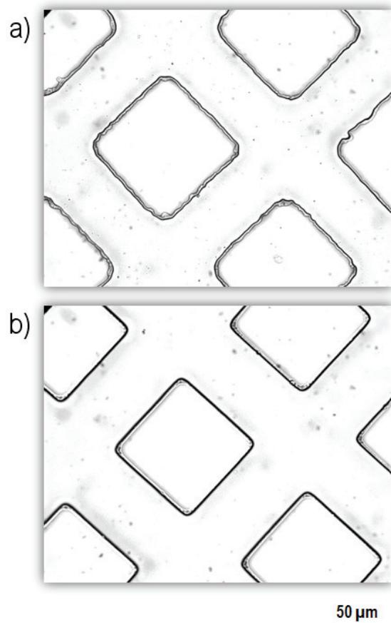
Figure 2.10: Microscopic images of a PDMS microfluidic network. PDMS was cast from a master made with (a) ink-printed foil mask and (b) chrome mask. The sections show 6 pillars with the surrounding channels.
