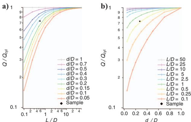
Figure 17. Simulation results for the correction factor  $\beta$  for different aspect ratios of the sample. The correction factor  $\beta = Q/Q_{\text{cyl}}$  relates the flow rate to the sample with a cored hole to the flow rate of a cylindrical sample without the annulus section. (a) Diagram shows the correction factor as a function of the cylinder length. (b) Diagram shows the correction factor as a function of the cored-hole diameter.
