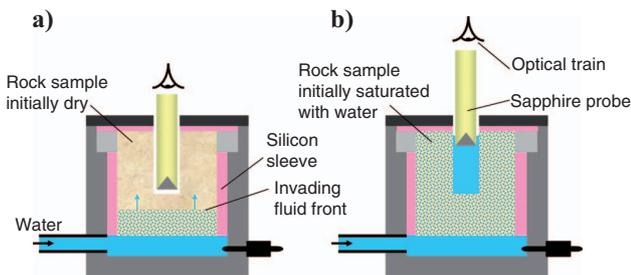
Figure 14. Setup for fluid injection experiments. (a) True imbibition case whereby water is injected into an initially dry rock sample, hence providing a transient state measurement. (b) Steady state measurement, whereby water is pushed through an already saturated rock sample.
