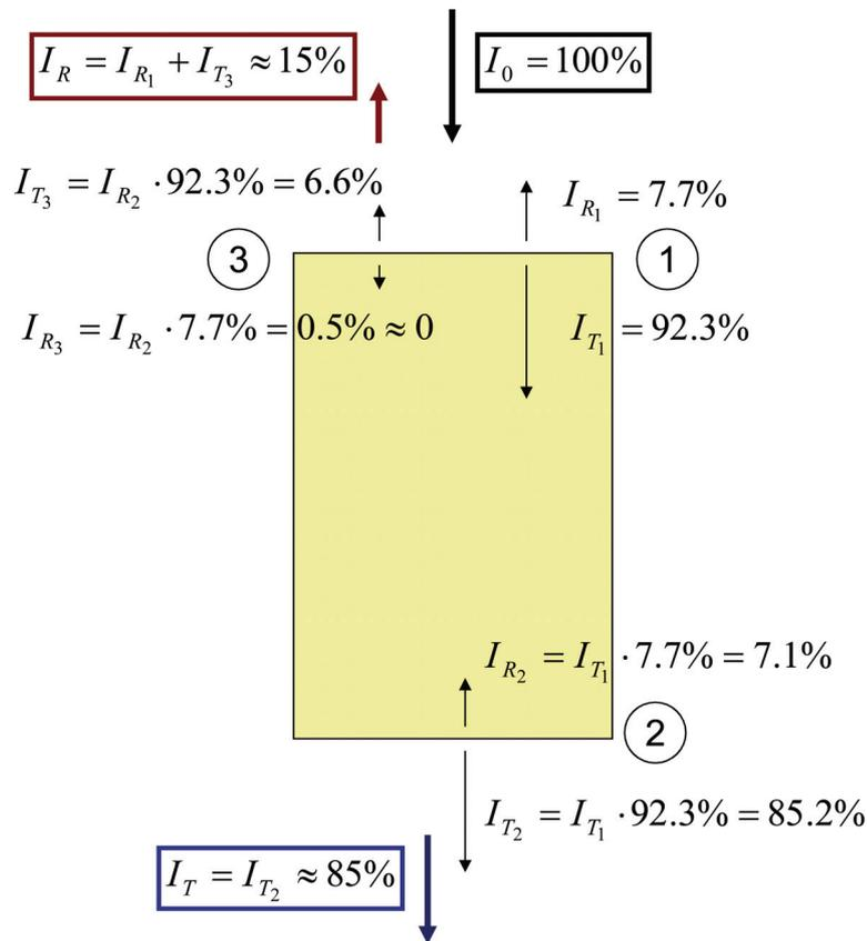
Figure C.8: Transmittance and reflection at the sapphire probe.
