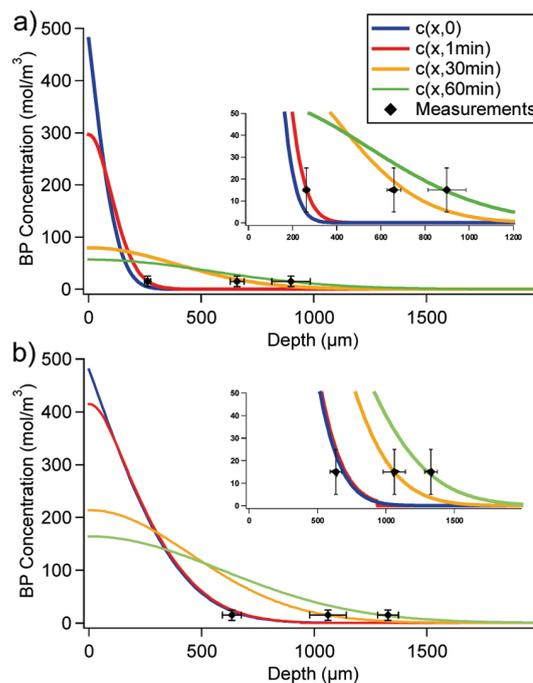
**Figure 10.** BP concentration profiles during the drying period at discrete time steps calculated according to linear diffusion are plotted as solid lines. Black markers show experimental data. Initial priming was performed with a flow of 10 wt % BP in acetone for (a) 1 min and (b) 10 min.
