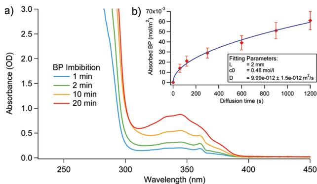
**Figure 5.** (a) UV absorption spectra of PDMS imbibed with BP. PDMS samples were saturated with acetone prior to diffusion experiments and then immersed in a 10 wt % BP solution in acetone for the indicated times. (b) Amounts of absorbed BP determined via UV absorption (markers) and curve fit (solid line) as a function of diffusion time.
