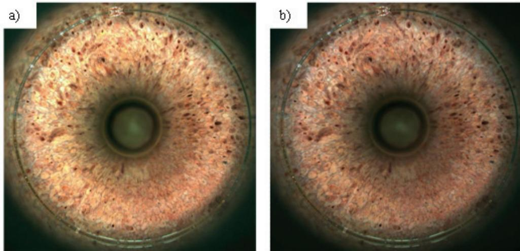
Figure C.5: Images of the same rock sample taken with a plate beam splitter and a polarizer. a) Polarizer at position X, b) Polarizer at position X + 90°.
