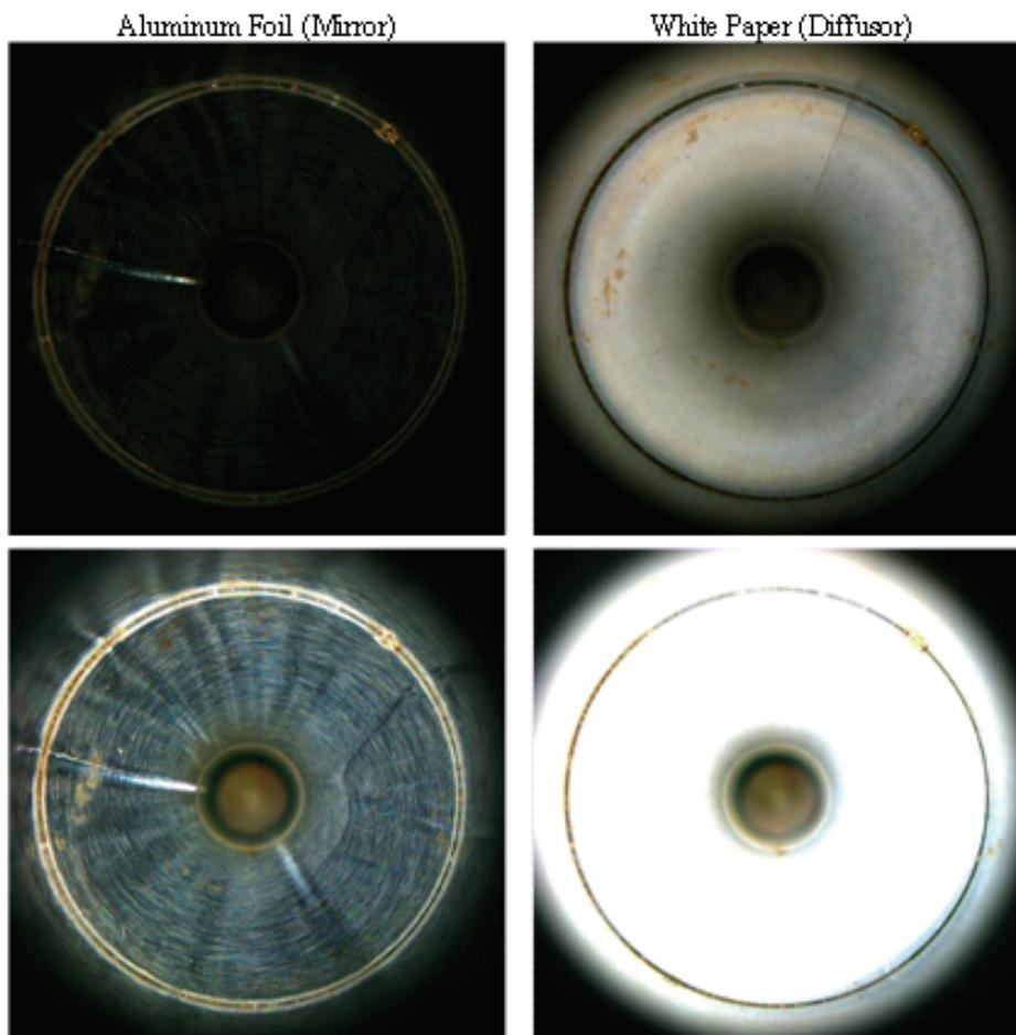
Figure C.16: Images obtained with the ring-light illumination setup for a sapphire probe surrounded by a mirror and a diffuser. Images in each row are taken with identical illumination intensity.
