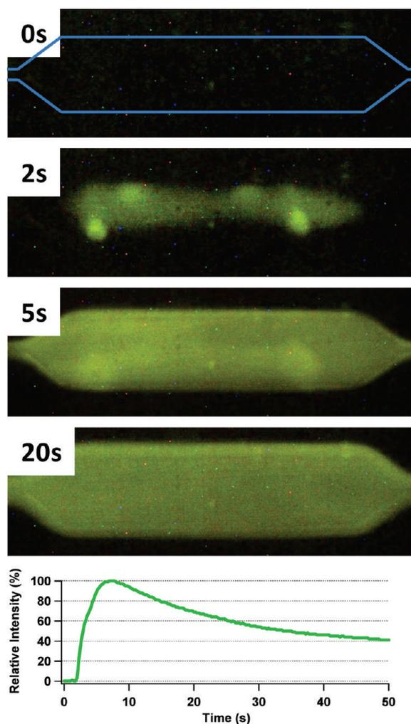
**Figure 11.** In situ monitoring of reacted BP phosphorescence during graft polymerization of a cavity structure enclosed in PDMS. The shape of the cavity is outlined in blue in the first frame. Images at various time steps are given. The evolution of the average phosphorescence intensity over the first 50 s is shown on the bottom.
