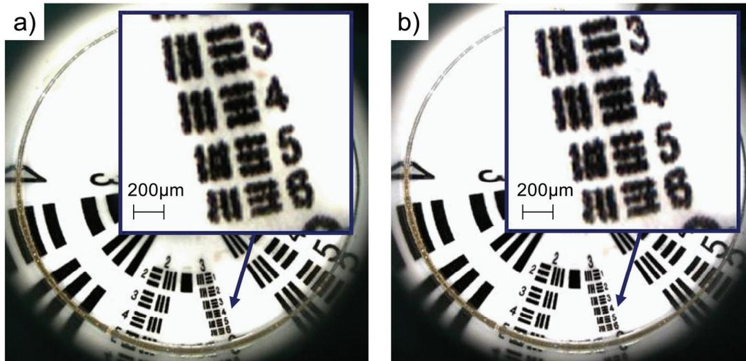
Figure C.6: Image of a resolution target obtained with a) beam splitter, b) mirror. The exposure time was adjusted to compensate for the lower intensity with the beam splitter setup.
