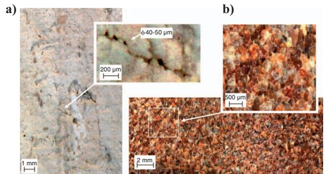
Figure 7. Examples of digital cores from two rock samples. (a) Digital core image obtained from a white chalky carbonate rock. (b) Digital core image obtained from sandstone. Additional zoom views of distinct features are shown for both digital cores highlighting the true resolution of the images.
