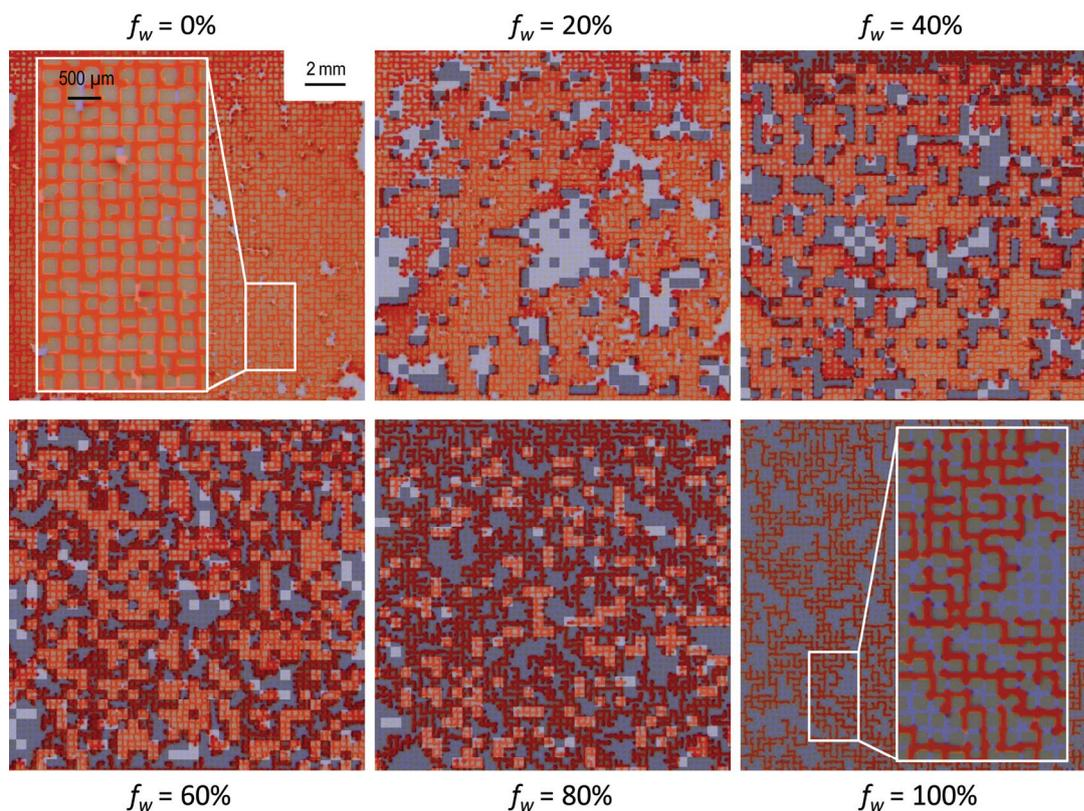
Figure 2.17: Water-saturated micromodels with channel size distribution (Type III) at various hydrophilic wettability fractions  $f_w$  showing oil invasion after breakthrough. Hydrophilic (water-wet) pore clusters are indicated by dark shades while bright shades represent hydrophobic (oil-wet) zones.
