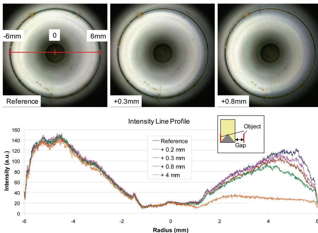
Figure C.20: Illumination intensity at different gap sizes.
