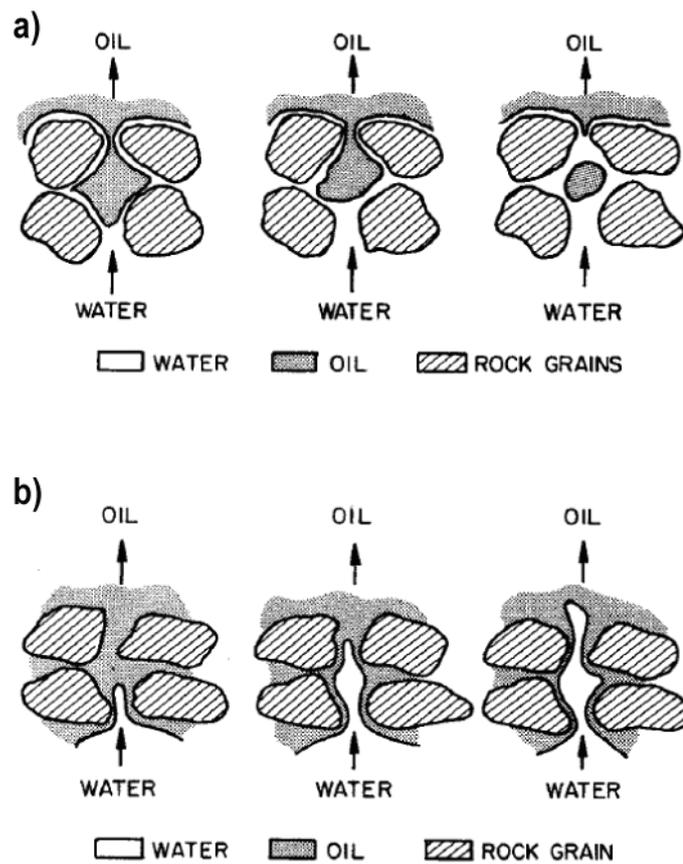
Figure 1.8: Water displacing oil from a pore in (a) a strongly water-wet rock, and (b) a strongly oil-wet rock [107].
