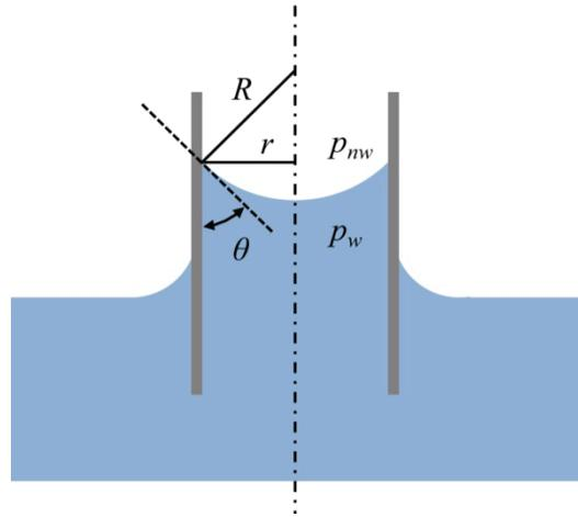
Figure 1.4: Capillary rise in a cylindrical tube of radius  $r$ . The tube (gray) shown in cross-section is dipped in water (blue). Water is wetting the tube material and a spherical meniscus of radius  $R$  is formed.
