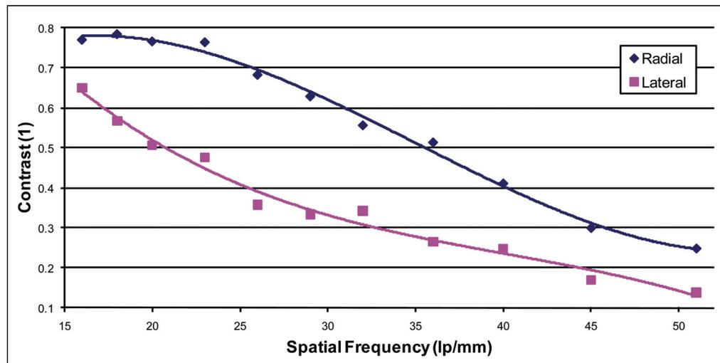
Figure C.25: Contrast transfer function for different spatial frequencies in radial and lateral direction.
