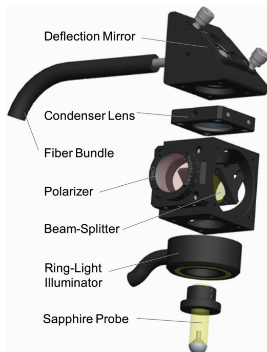
Figure C.3: Detail view of the MGI setup. The beam-splitter cube, sapphire probe and the functional components of the illumination systems are shown. Mechanical supports are not shown in the figure. The orientation is such that the camera can look through the polarizer into the beam-splitter cube.
