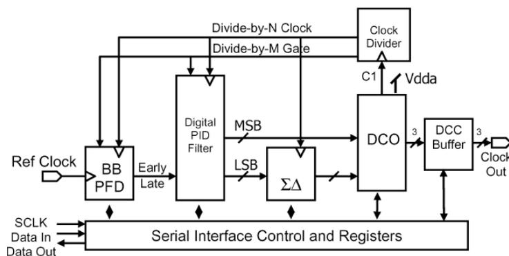
Figure 1.13: The ADPLL architecture proposed in [4] for  $4\text{GHz}$  applications
