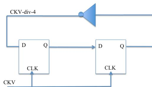
Figure 3.34: Block diagram of the frequency divider
