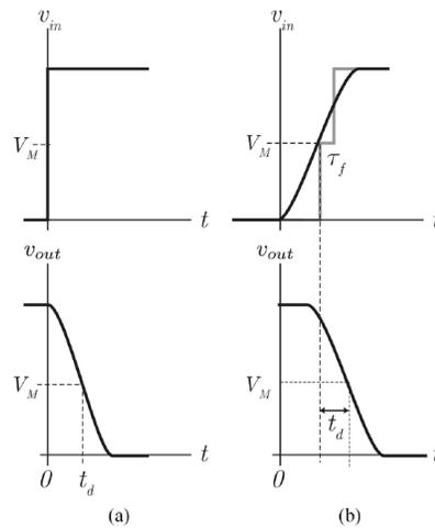
Figure 3.5: Delay times in case of: (a) Ideal step input. (b) Real step input
