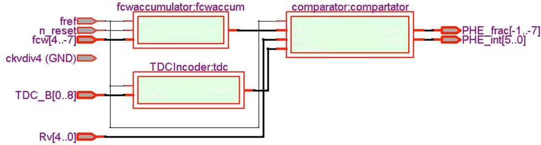
Figure 3.36: The phase detector block diagram implemented on FPGA
