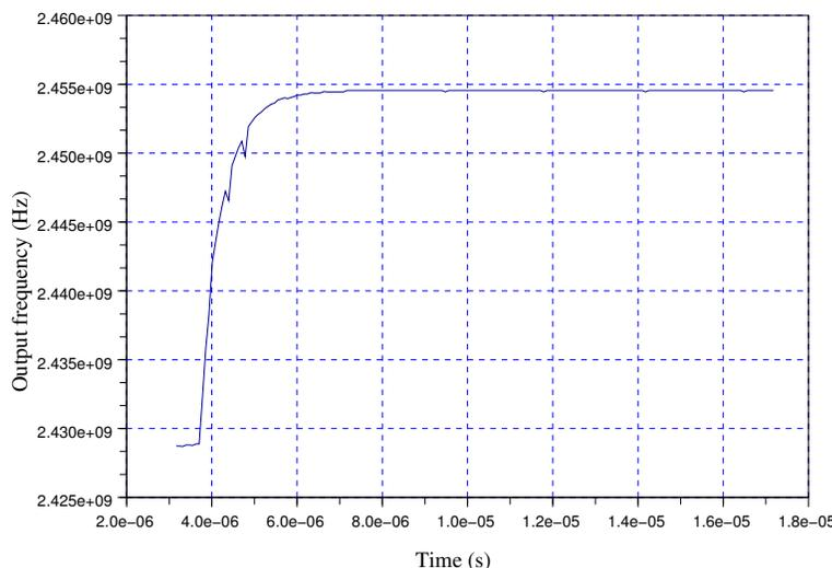
Figure 2.17: Transient simulation of the VHDL-AMS model of ADPLL. The lock time is equal to  $5\mu s$
