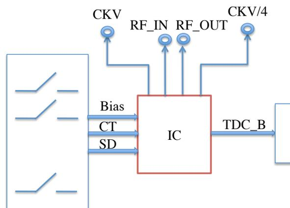
Figure 4.1: Block diagram of open loop test card
