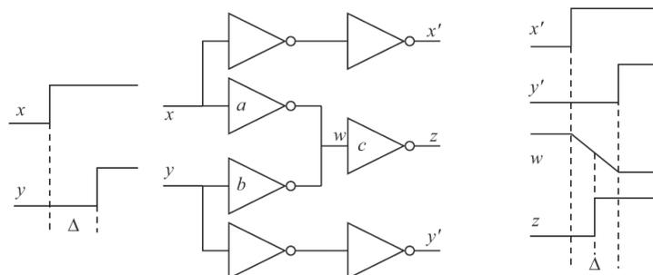
Figure 3.7: The inverter interpolator of [8, 9]
