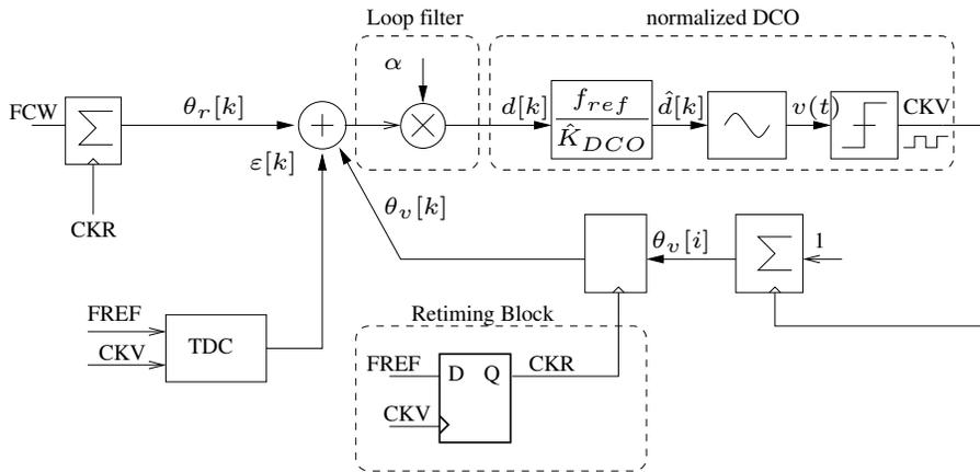
Figure 2.1: The block diagram of our ADPLL model
