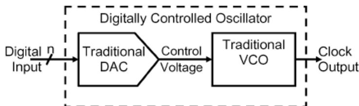
Figure 1.14: DCO formed by DAC and VCO
