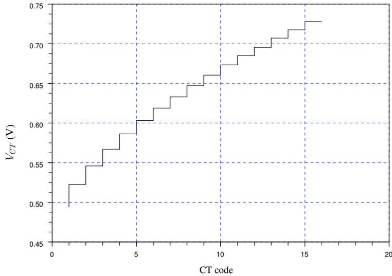
Figure 3.24: Simulation result of 16 bit DAC shows the variation of  $V_{CT}$  in function of CT code
