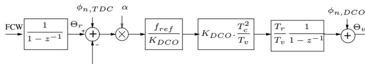
Figure 2.21: The ADPLL model with noise
