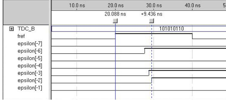
Figure 3.39: Simulation result of the TDC encoder. Delay time is around 10ns
