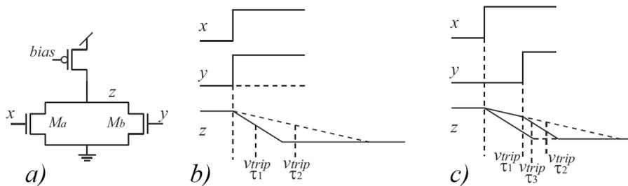
Figure 3.8: A modified digital interpolator, its timing diagram with b) equal time inputs, and c) unequal time inputs, [10]
