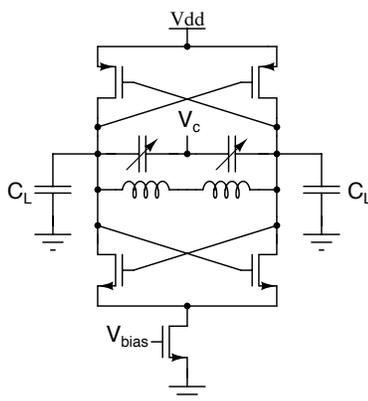
Figure 1.3: A cross coupled LC oscillator
