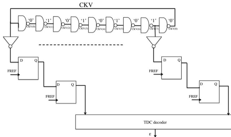
Figure 3.25: The TDC reads the output of each stage of the ring at the rising edge of the FREF. This state is then decoded to determine  $\varepsilon$
