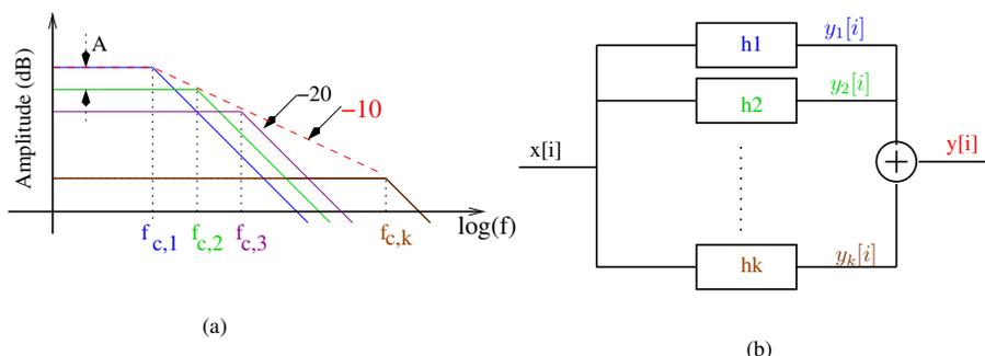
Figure 2.11: (a): Composition of -10 dB slope from low-pass responses of -20 dB slopes. (b): The generated 1/f noise signal from the sum of low-pass filtered white noise signals
