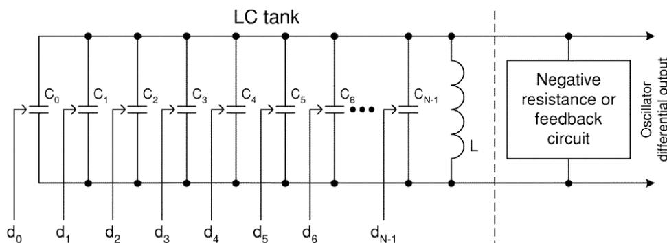
Figure 1.16: LC-tank-based oscillator with switchable capacitors
