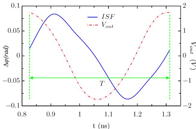
Figure 2.15: The ISF function of the LC oscillator
