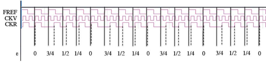
Figure 2.4: The retiming error is periodic
