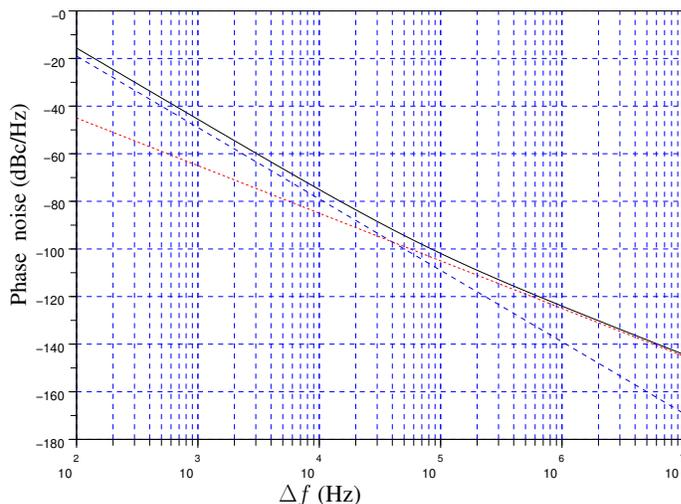
Figure 2.16: Simulation results of Pnoise analysis in solid line. The  $1/f^2$  and  $1/f^3$  phase noise estimation by the LTV model in dash lines. The  $\omega_{1/f^3}$  corner is viewed at 30kHz.
