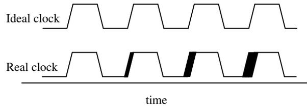
Figure 1.9: The jitter in periodic signal
