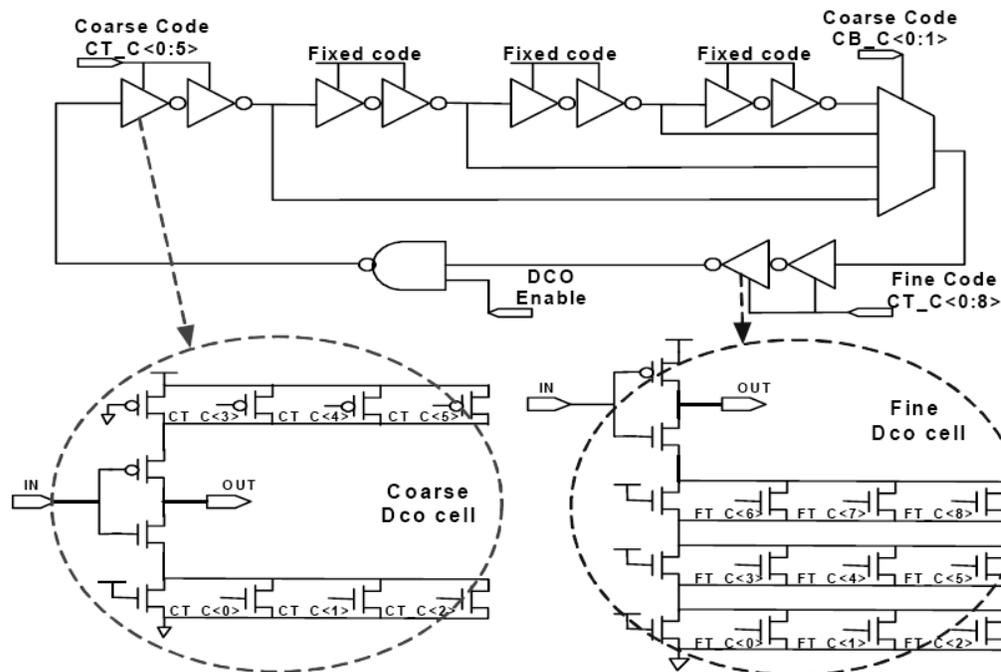
Figure 1.19: Ring DCO circuit of [5]
