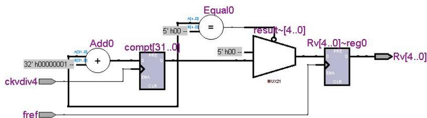
Figure 4.9: Block diagram of the digital counter implemented on the FPGA
