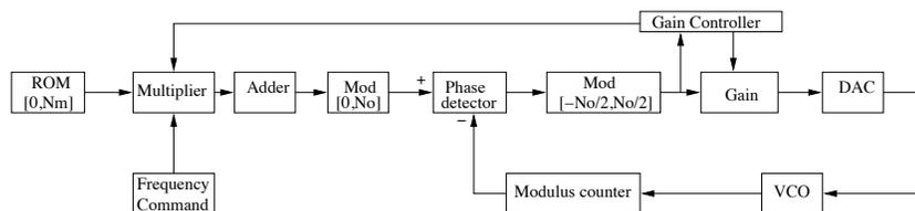
Figure 1.10: Integer digital frequency synthesizer [1]
