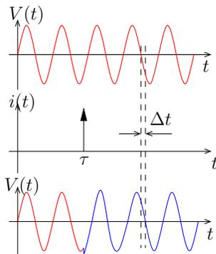
Figure 1.8: The response of an oscillator to current injection is time dependant
