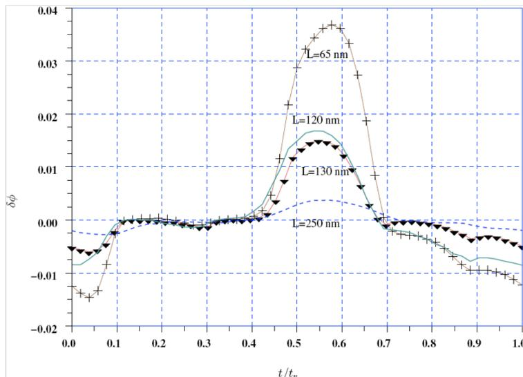
Figure 3.14: The ISF function for the ring oscillator interpolator for  $L = (65\text{nm}, 120\text{nm}, 130\text{nm}, 250\text{nm})$
