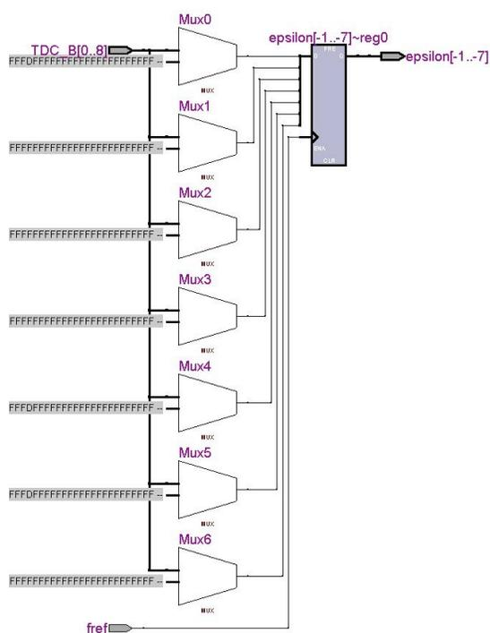
Figure C.1: The block diagram of the TDC encoder synthesized by Quartus and programmed on Stratix II
