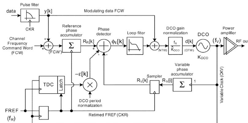
Figure 1.12: ADPLL frequency synthesizer for Bluetooth/GSM applications, [3]
