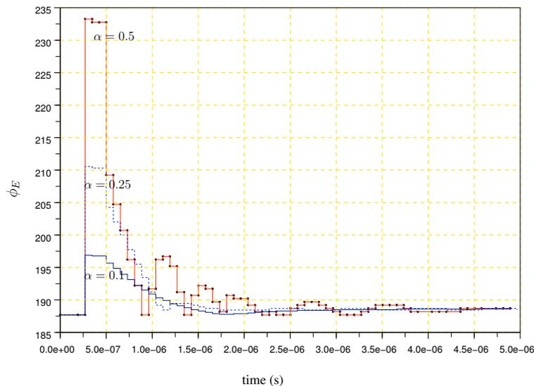
Figure 2.18: Variations of the ADPLL time response with the attenuation  $\alpha$
