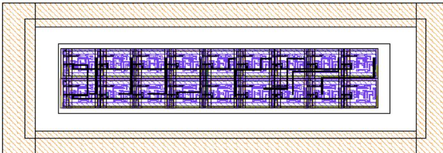
Figure 3.27: Layout view of the TDC register
