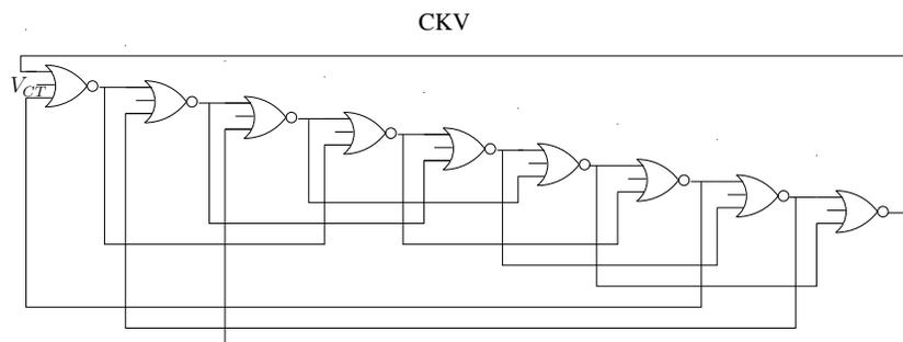
Figure 3.10: The interpolative oscillator (9,7) based on two ports NOR gates
