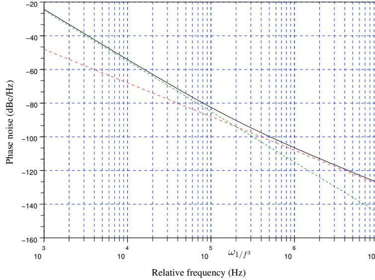
Figure 3.19: The Pnoise simulation results of the ring DCO
