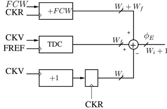
Figure 2.2: The phase detector diagram. CKR is the retimed reference clock
