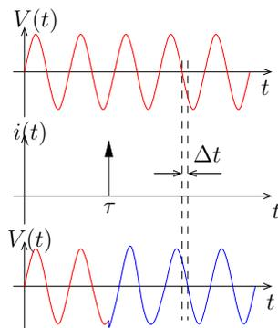
Figure 2.13: An impulse is injected at time  $\tau$  and the resulting shift  $\Delta t$  of zero-crossing is calculated few periods afterwards
