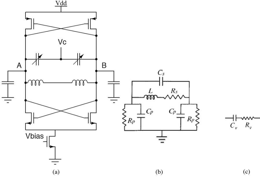
Figure 1.5: (a) Cross coupled LC VCO. (b) Inductor model. (c) varactor model
