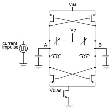
Figure 2.8: The LC oscillator of the ADPLL
