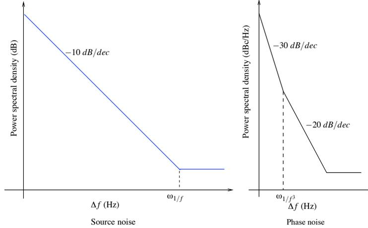
Figure 1.7: The up conversion of sources noise around carrier frequency
