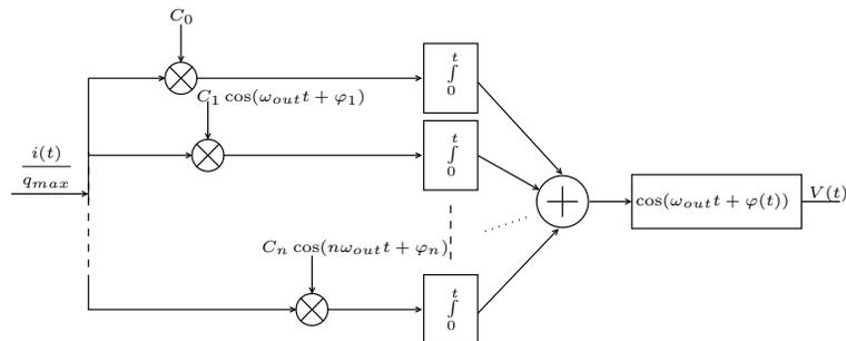
Figure 2.12: The DCO phase noise model
