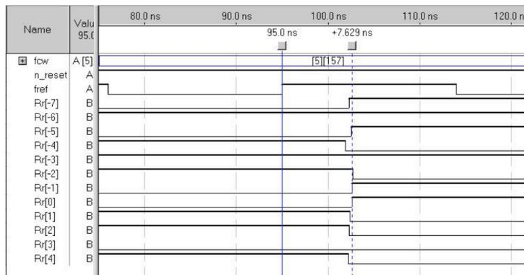
Figure 3.38: Delay time of FCW accumulator is around 7ns
