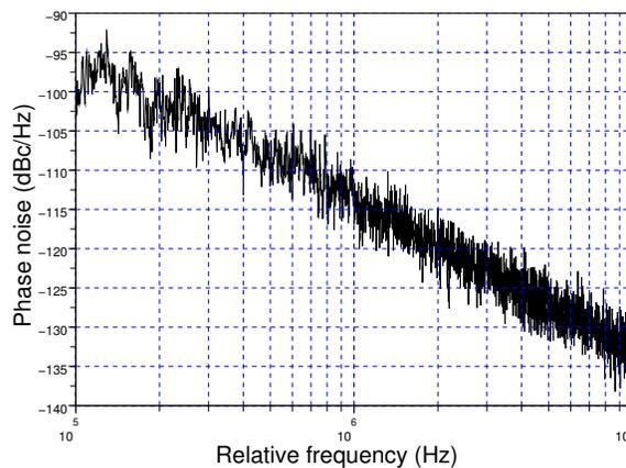
Figure 4.11: The measured phase noise of CKV/4 signal. CKV frequency is equal to  $472\text{MHz}$
