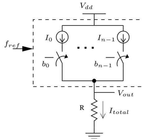
Figure 3.20: Digital-to-Voltage block diagram
