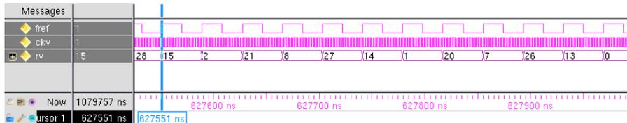
Figure 3.29: Modelsim result of digital counter model.
