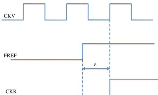
Figure 2.3: The retiming error
