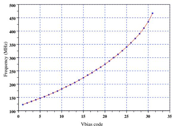
Figure 4.3: The DCO tuning range in function of the bias word with CT=1
