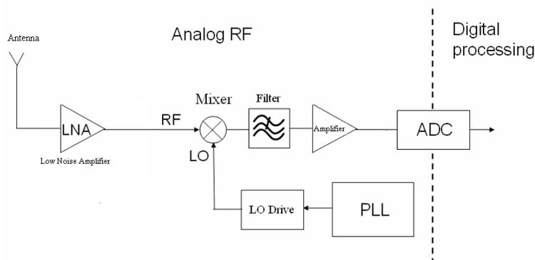
Figure 3.2: RF front-end of TV receiver
