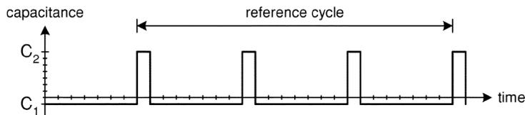
Figure 1.17: DCO dithering by changing the discrete capacitance at high rate
