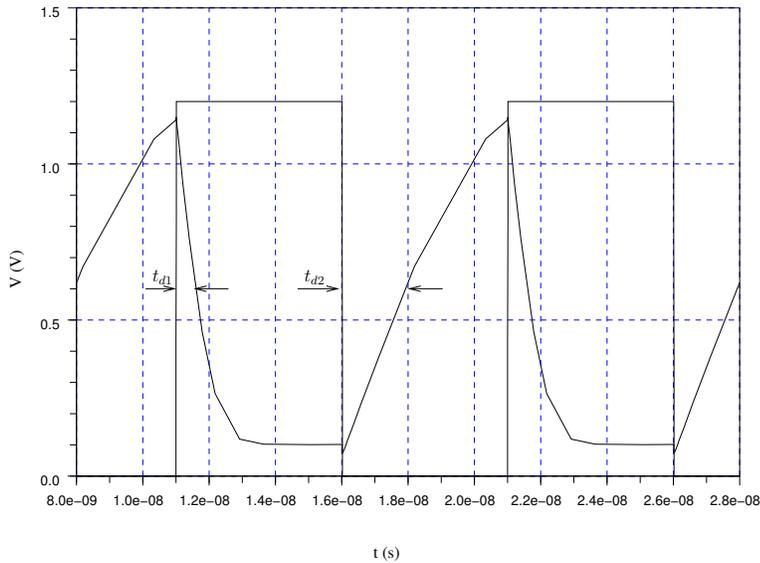
Figure 3.12: Delay times of rising and falling edges of NOR cell
