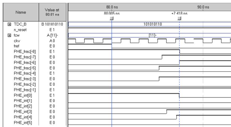
Figure 3.40: Delay time of the phase comparator block in the FPGA is around 9ns
