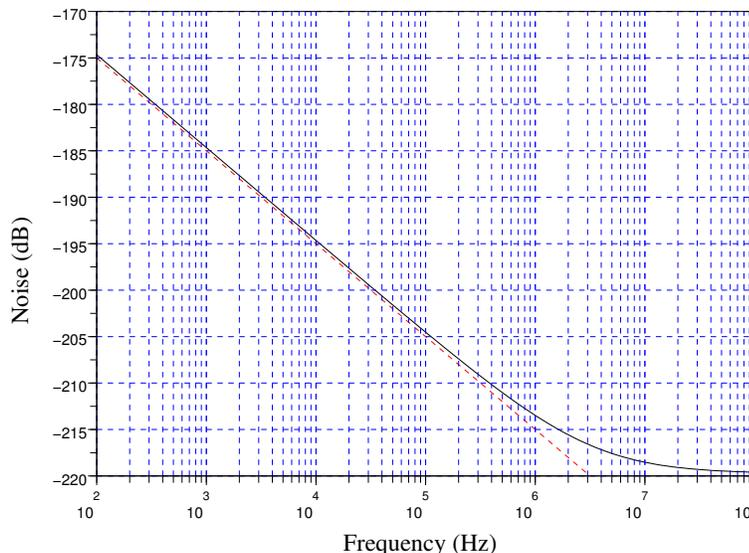
Figure 2.10: The CMOS noise of the LC oscillator. This is the result of Spectre analysis
