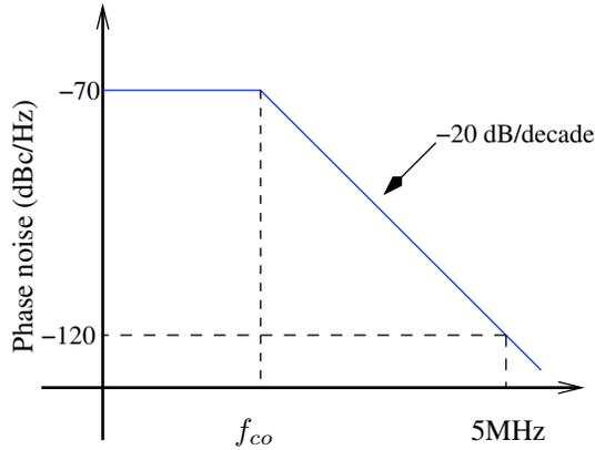
Figure 3.3: Phase noise behavior of first order ADPLL designed for TV application
