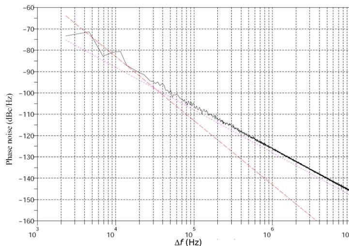
Figure 2.19: The power spectral density of DCO phase noise. The  $\omega_1/f^3$  point is observed at 30kHz
