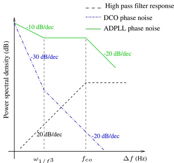
Figure 2.22: The ADPLL phase noise transfer function of DCO noise
