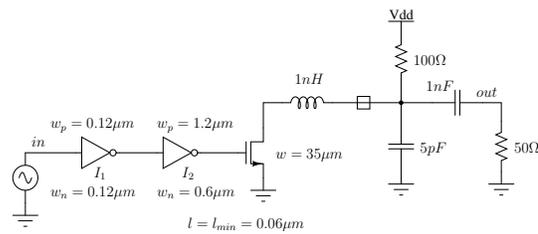
Figure 3.30: The output buffer
