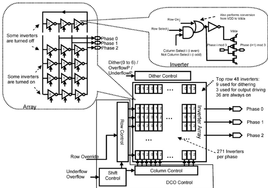
Figure 1.18: Tri-state inverter based DCO proposed in [4]
