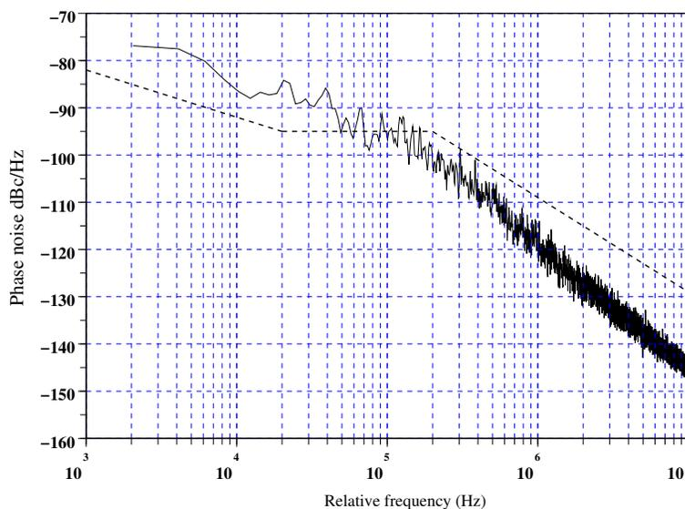
Figure 2.23: The power spectral density of RF output signal of the ADPLL
