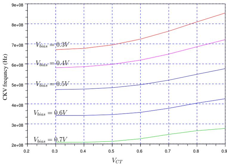
Figure 3.18: DCO tuning range in function of  $V_{bias}$  and  $V_{CT}$
