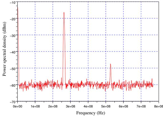
Figure 4.5: Measured CKV power spectral density. CKV has a peak at 263MHz and an amplitude of -16dBm
