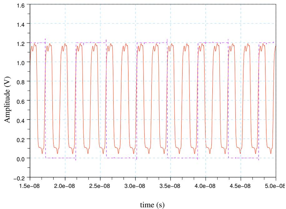
Figure 3.35: CKV and CKV/4 signals have respectively 427.320MHz and 106.791MHz frequencies (CT=7, bias=15).
