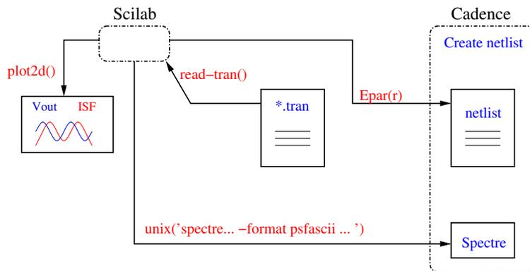
Figure 2.14: The automatic implementation of the ISF between Spectre and Scilab
