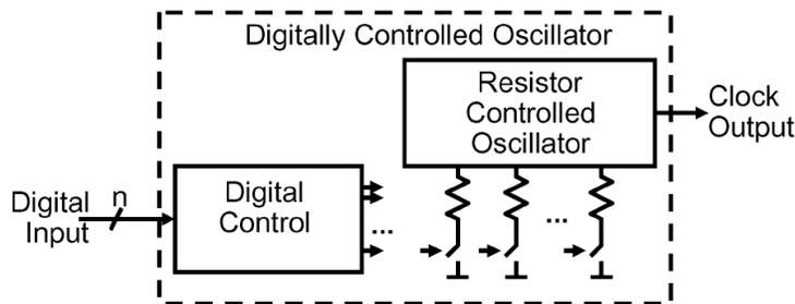
Figure 1.15: The direct digital approach of DCO control
