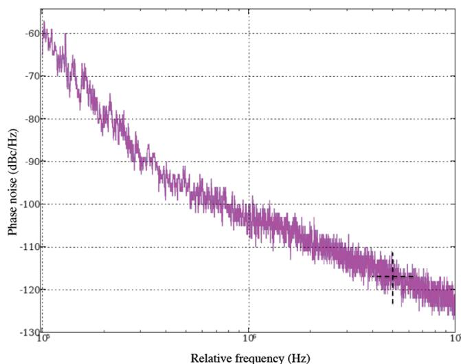
Figure 4.4: Measured phase noise of CKV for  $f_{CKV}=470\text{MHz}$
