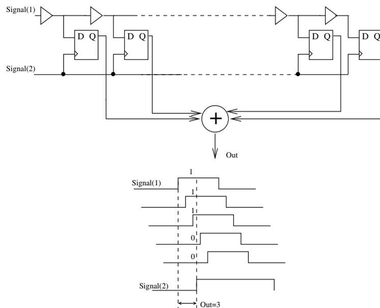
Figure 1.22: TDC delay line architecture
