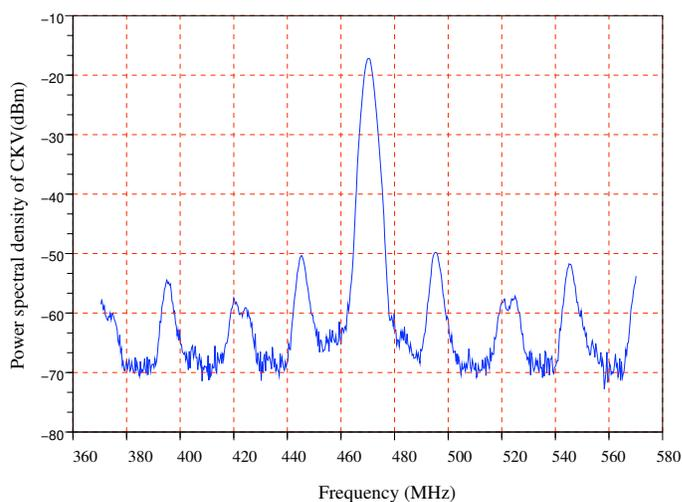
Figure 4.6: Power spectral density of CKV in the presence of FREF
