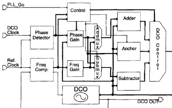
Figure 1.11: ADPLL architecture of fractional frequency synthesis proposed by [2]
