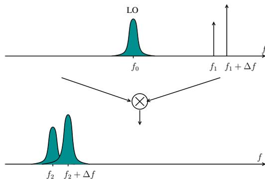
Figure 1.6: Effects of the phase noise behavior of LO on the received signal
