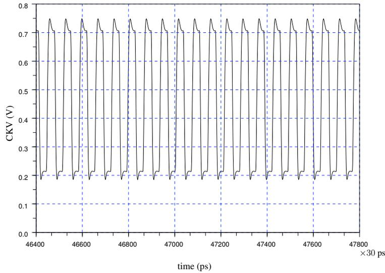
Figure 3.32: Transient analysis results of the buffer
