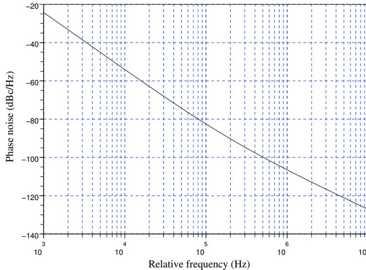
Figure 3.33: Pnoise analysis results with the buffer
