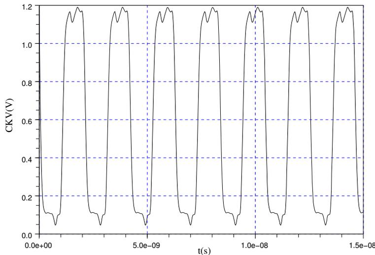
Figure 3.17: The CKV signal before the buffer stage. Its frequency is equal to 427.320 MHz and the digital control words are  $CT=7$  and  $Bias = 15$
