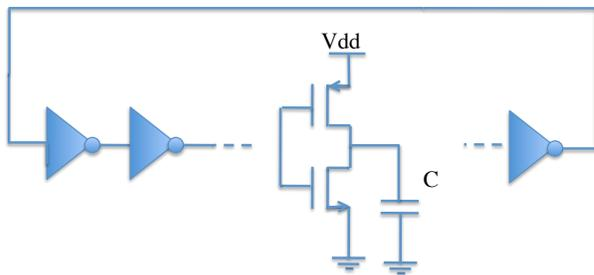
Figure 3.6: ring oscillator based on inverter gates
