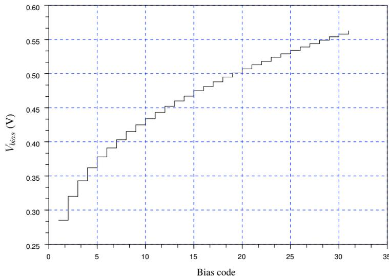
Figure 3.23: Simulation result of 31 bit DAC shows the variation of  $V_{bias}$  in function of Bias code
