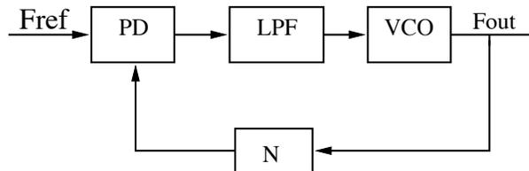
Figure 1.1: Integer frequency synthesizer
