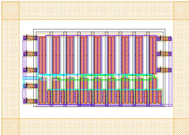
Figure 3.16: Layout view of nine interpolative DCO
