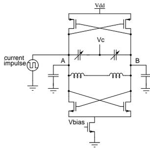
Figure A.1: The cross coupled LC oscillator
