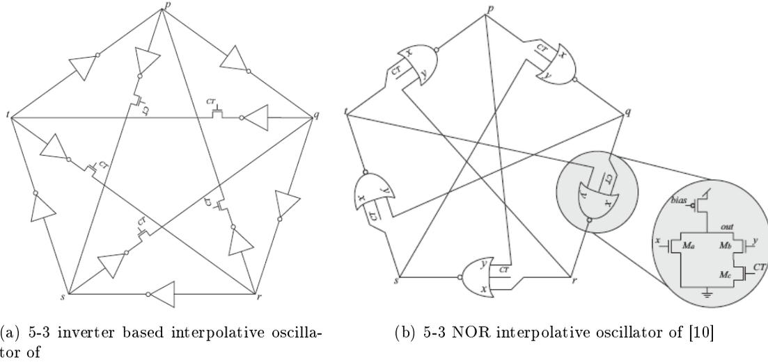
Figure 3.9: Two implementations of balanced 5-3 interpolative oscillator
