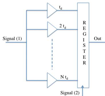
Figure 1.23: TDC architecture formed by parallel delay gates [6]
