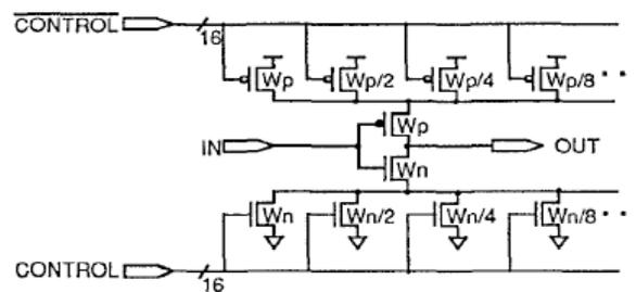
Figure 1.21: The digital control word is binary coded in the DCO of [2]
