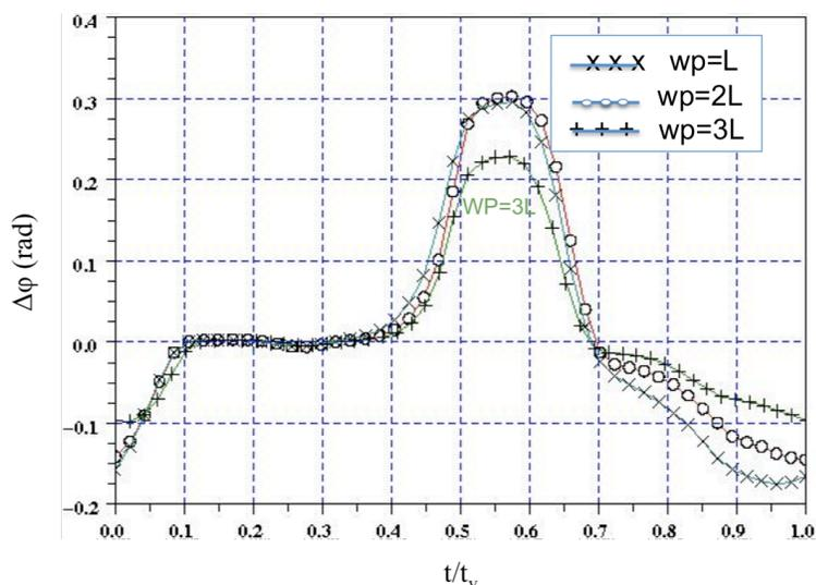
Figure 3.15: The ISF function of the interpolative oscillator in function of  $W_p/W_n$  for the  $W_n=L=250\text{nm}$
