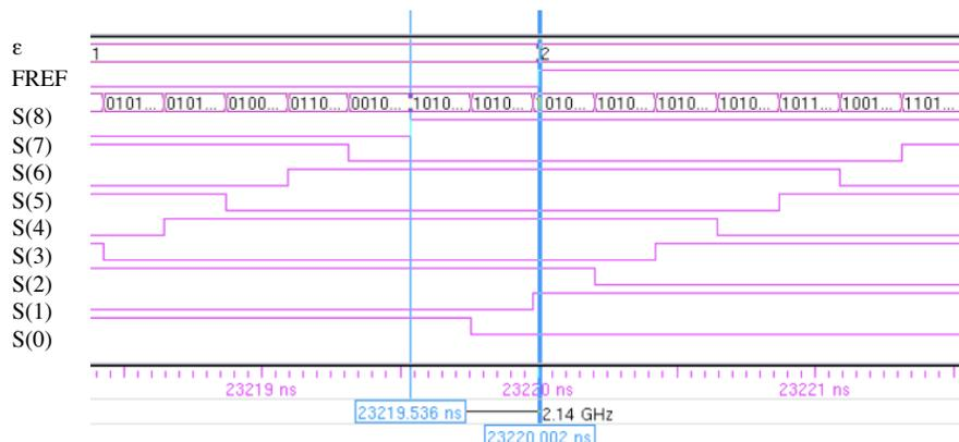
Figure 3.28: The simulation results of the TDC.  $\varepsilon$  is the delay time between the rising edges of FREF and CKV.
