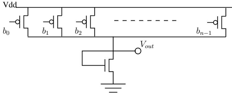
Figure 3.22: The Digital to Voltage Converter
