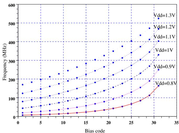
Figure 4.7: Variation of the tuning range of the DCO as a function of DCO supply  $V_{dda}$
