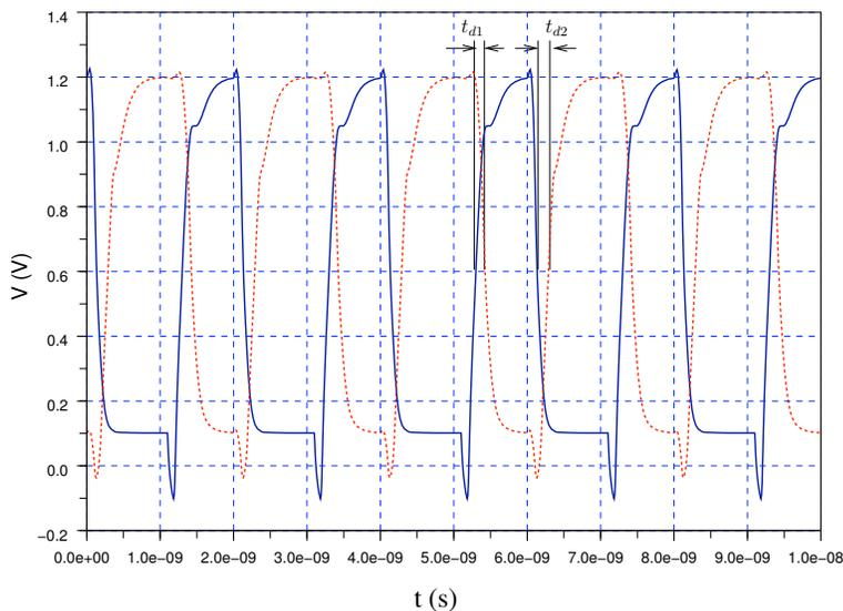
Figure 3.13: Delay times of rising and falling edges of the NOR gate
