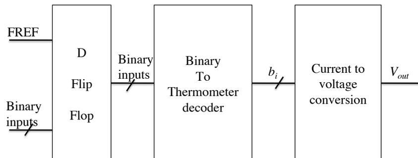
Figure 3.21: Block diagram of Digital-to-voltage converter synchronized with FREF
