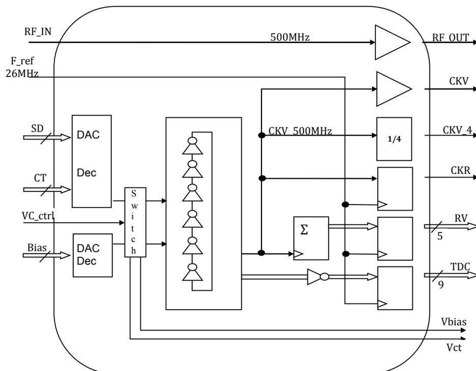
Figure 3.4: Block diagram of the CMOS 65nm part of the ADPLL
