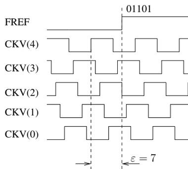
Figure 3.26: Ring status example for 5 stages ring oscillator
