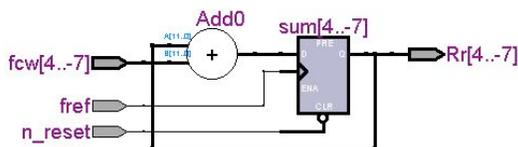
Figure 3.37: An accumulator of the frequency control word
