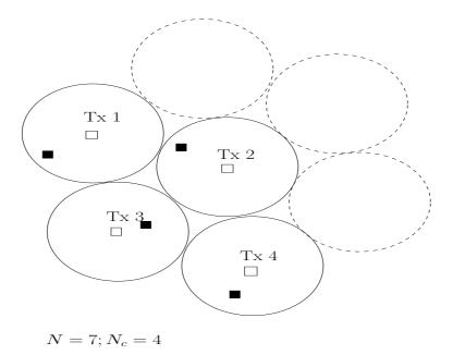
Figure 4.1: This figure illustrates a system of N=7 cells where  $N_c=4$  cells form a coordination cluster. Empty squares represent transmitters whereas filled squares represent receivers. The noise power (which includes out-of-cluster interference) undergone in each cell varies from link to link.
