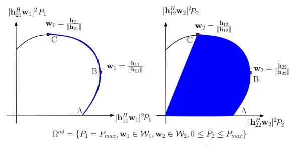
Figure 5.3: The graphical illustration of the candidate set  $\Omega^{nd}$  as the shaded area which is a subset of the received power regions  $\Phi_i$ .
