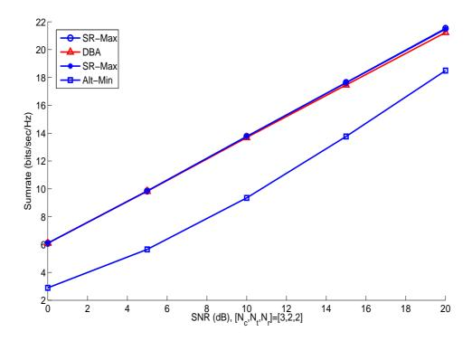
Figure 4.2: Sum rate comparison in multi links systems is illustrated in Fig. 4.2 with  $[N_c, N_t, N_r] = [3, 2, 2]$  with increasing SNR. DBA, SR-Max and Max-SINR achieve very close performance.
