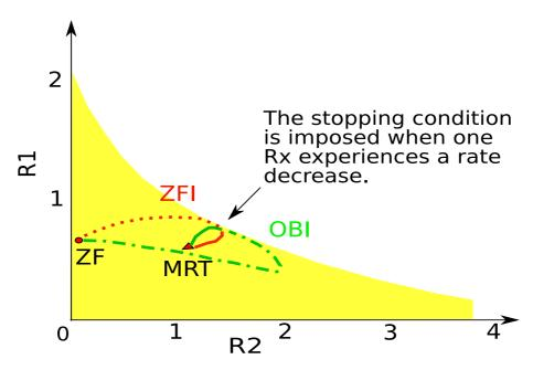
Figure 3.1: The trajectory of DBS within the rate region in the 2-user MISO-IC-SUD at SNR 15dB. The trajectories of both ZFI and OBI, starting at the MRT point (triangle), are illustrated in solid lines, with colors red and green respectively, whereas if there are no stopping conditions, the trajectories continue and end at the ZF point (circle) and are shown in dotted lines. As shown in the figure, the algorithms stop close to the Pareto boundary.
