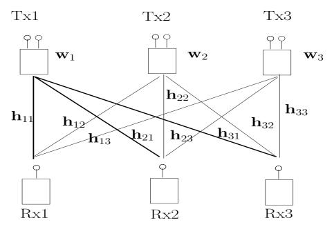
Figure 2.2: The channel model of the MISO-IC with N=3 and  $N_t=2$ .
