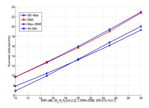
Figure 4.5: Sum rate performance for asymmetric channel, with one link under strong interference within the cooperating cluster, is illustrated.
