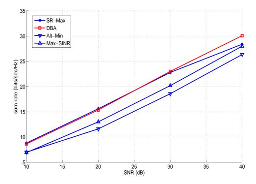
Figure 4.4: Sum rate performance for asymmetric channel, with one link under strong noise, is illustrated. The strong noise, from out of cluster interference, is  $20 \, \mathrm{dB}$  stronger than other links. DBA outperforms standard IA methods thanks to a proper balance between egoistic and altruistic beamforming algorithm.
