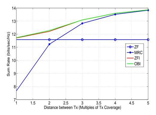
Figure 3.3: The performance comparison of DBS against distance between transmitters at SNR  $10\mathrm{dB}$ .
