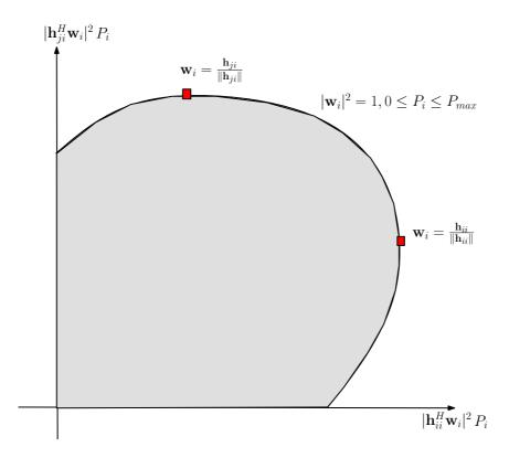
Figure 5.2: The power gain region for Tx i.
