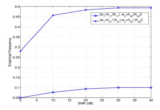
Figure 5.8: MRT optimality in  $\mathbb{R}^{nd}$  when SNR increases: interference should be maximized half of the time when SNR goes to infinity.
