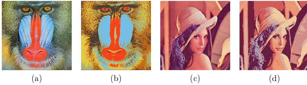
Figure 4.3: Two typical images used in computer vision to test segmentation algorithms: Baboon (on the left) and Lena (on the right). From the original images \{(a),(c)\} , the K-Means algorithm was launched to classify image pixels using: (b) K = 6 clusters, and (d) K = 8 clusters.
