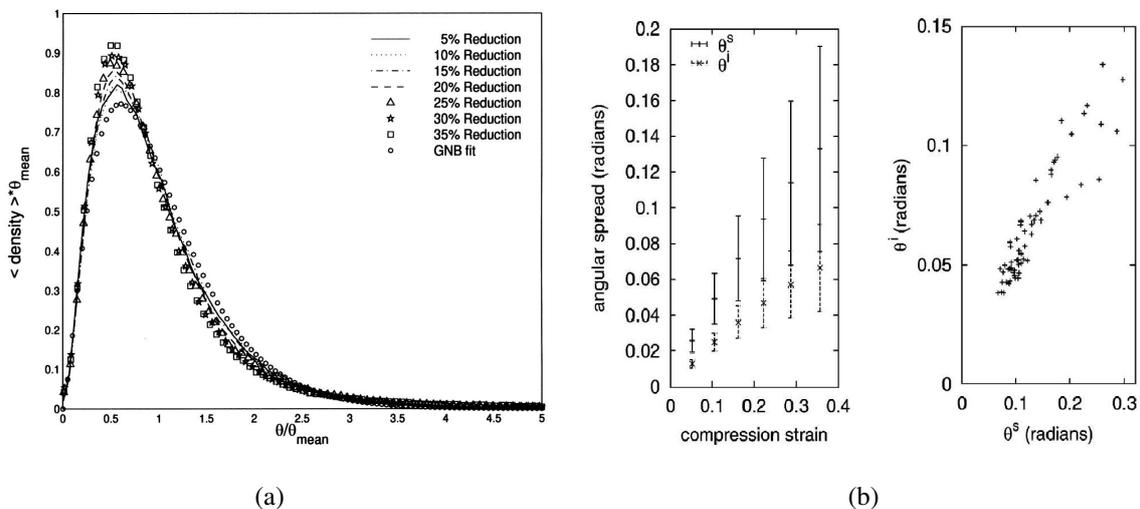
Fig. 6.7: (a) Intragranular misorientation scaled with the average misorientation for a group of crystals and fit from [HUGHES et al., 1997] (b) Correlation between grain orientation spread  $\theta^s$  and grain average misorientation  $\theta^i$  and their evolution with compressive strain [DAWSON et al., 2002]
