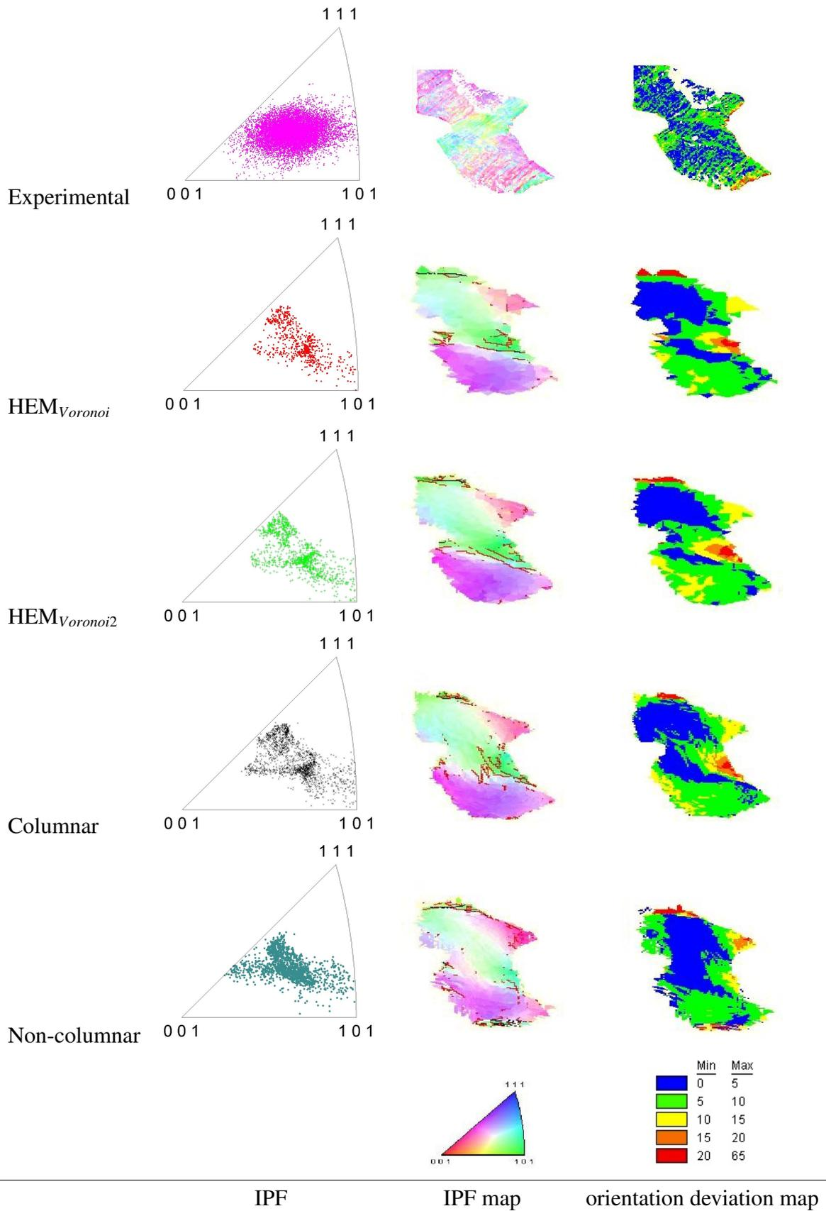
Fig. 6.45: Orientation deviation map and inverse pole figures (sample normal axis) for grain 2. Black and red segments in the IPF maps of the simulations represent high angle ( $>15^\circ$ ) and low angle grain boundaries respectively ( $>5^\circ$ ).
