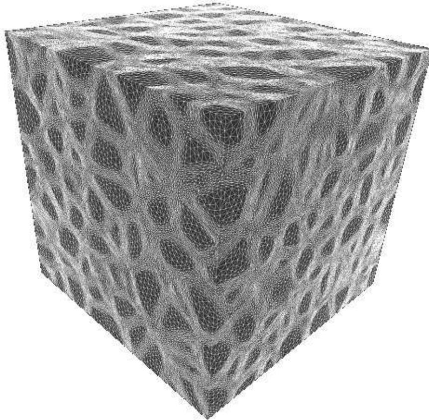
Figure 4 : Anisotropic mesh constructed from a digital microstructure made of 1000 grains
