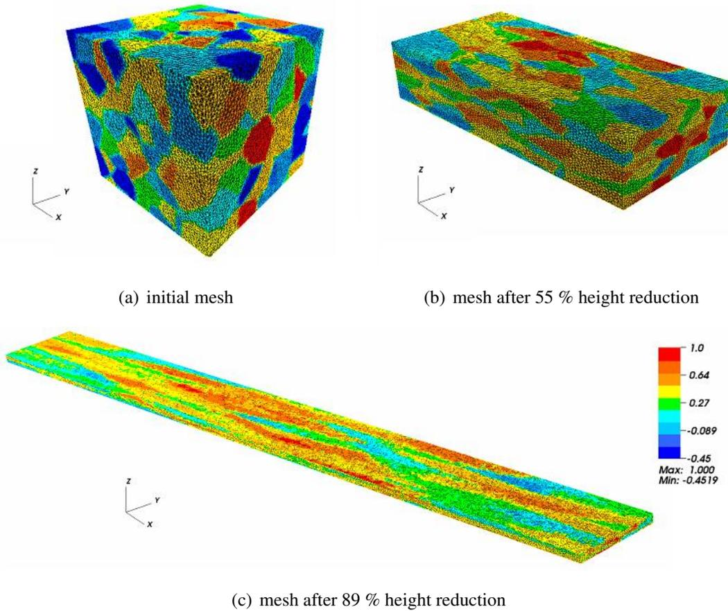
Fig. 6.10: 1st quaternion of a 500 grains polycrystal
