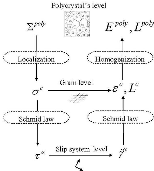
Fig. 2.2: From Polycrystal level to slip system level
