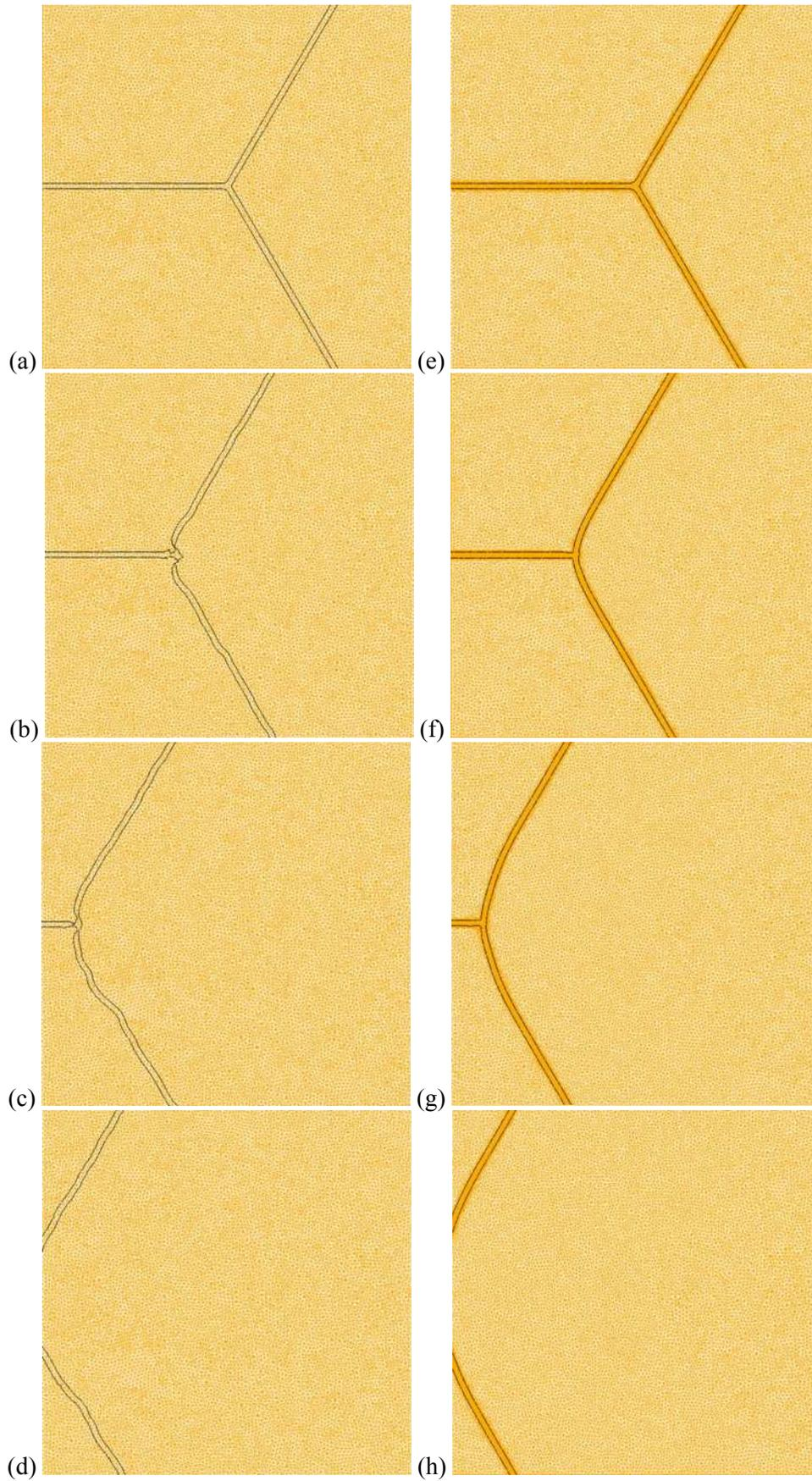
**Figure 7.**  $\pm 5 \cdot 10^{-3}$  isovalues of the three distance functions with isotropic mesh after (a) 0, (b) 120, (c) 300 and (d) 395 time steps and with adapted anisotropic mesh at the grain boundaries (darker orange) after (e) 0, (f) 120, (g) 300 and (h) 395 time steps
