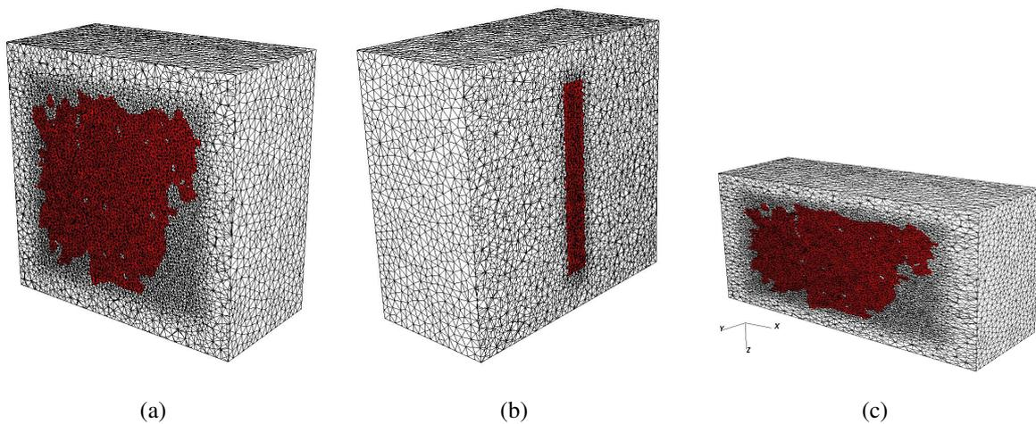
Fig. 6.19: (a) Cut along the Y axis revealing the inner mesh and the microstructure (484649 elements and 87993 nodes); (b) cut along the X axis; (c) cut along the Y axis for  $\boldsymbol{\varepsilon} = 0.4$
