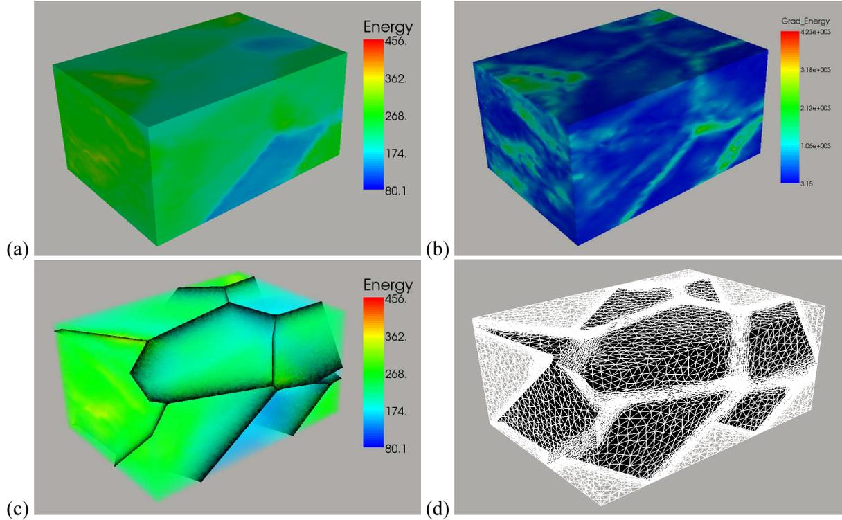
**Figure 10.** A 3D ten grains microstructure after plastic deformation: (a) external surface view of stored energy, (b) corresponding norm of the stored energy gradient ( $\|\nabla En\|$ ), (c) volumetric view of the stored energy with grain boundaries in black and (d) adaptive and anisotropic meshing in white, grain boundaries in black.
