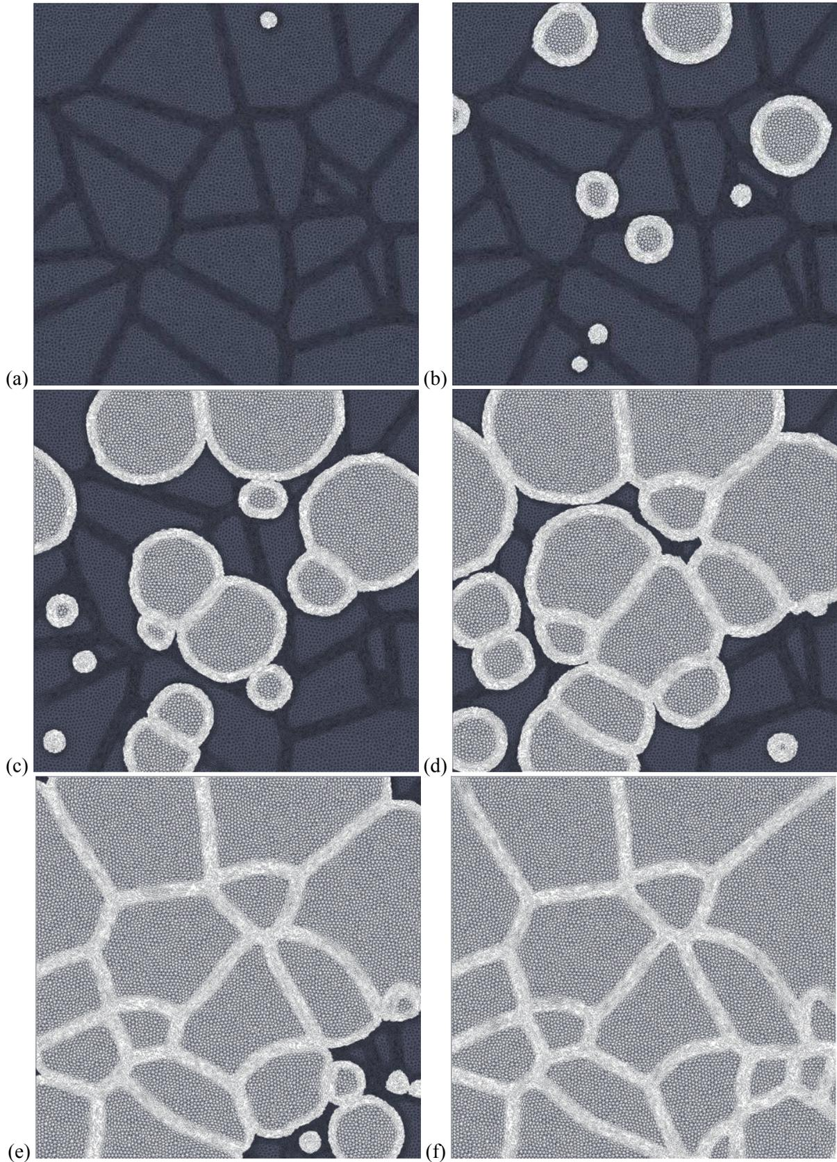
**Figure 8.** 2D simulation of primary recrystallization with an initial uniform stored energy. Recrystallized part in white corresponding to volume fractions of (a) 1%, (b) 10%, (c) 40%, (d) 60%, (e) 90% and (f) 100%
