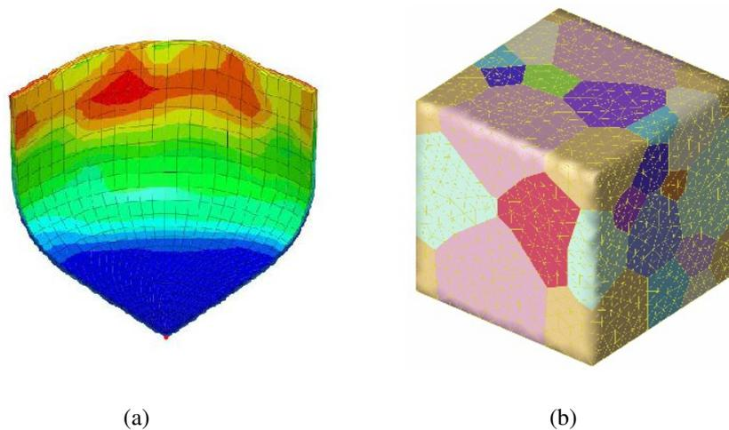
Fig. 1.3: Real-scale and small scale FE simulations: (a) simulation of deep drawing process using polycrystal plasticity [ROUSSELIER et al., 2009]; (b) A meshed polycrystal made of 17 grains [MANIATTY et al., 2007]
