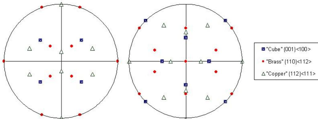
Fig. 6.2: 111 and 100 pole figures showing typical texture components that might appear during rolling
