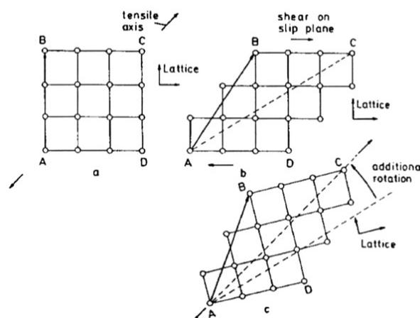
Fig. 2.1: “(a) and (b) A shear  $\gamma$  on a slip plane does not cause the lattice to rotate, although a material vector may rotate; (b) and (c) An additional rotation - which also causes the crystal lattice to rotate - will bring the crystal in a position corresponding to the strain forced upon it: e.g. pure elongation in the direction AC” [PEETERS et al., 2001]
