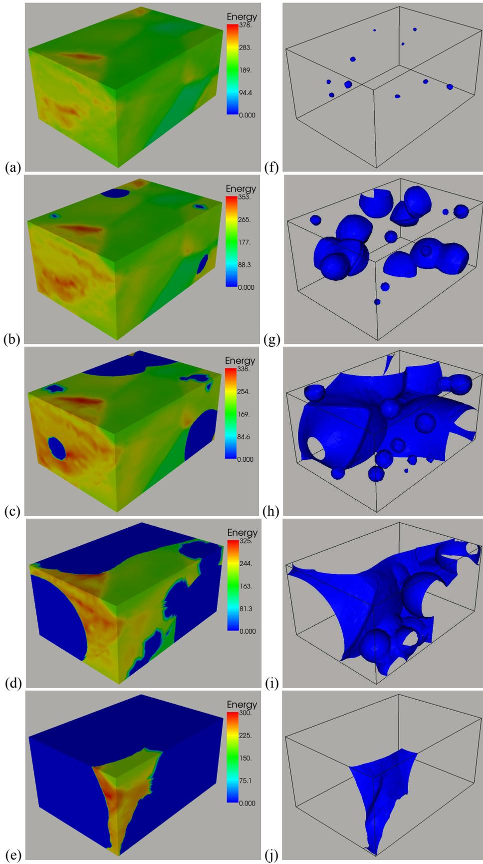
**Figure 11.** 3D recrystallization with a non uniform initial stored energy field: external surface view of the stored energy for recrystallized volume fractions of (a) 1%, (b) 15%, (c) 58%, (d) 80%, (e) 95%, and corresponding recrystallized front in blue (f-j).
