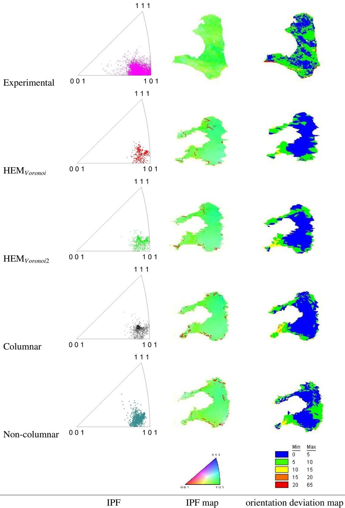
Fig. 6.51: Orientation deviation map and inverse pole figures (sample normal axis) for grain 8. Black and red segments in the IPF maps of the simulations represent high angle ( $>15^\circ$ ) and low angle grain boundaries respectively ( $>5^\circ$ ).
