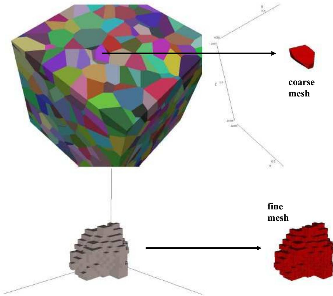
Figure 2 : Conversion of a digital sample into an initial finite element mesh, starting from a Voronoi tessellation (top) or a voxel representation (bottom).
