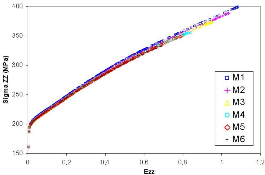
Fig. 5.5: Stress-strain curve for the different isotropic meshes
