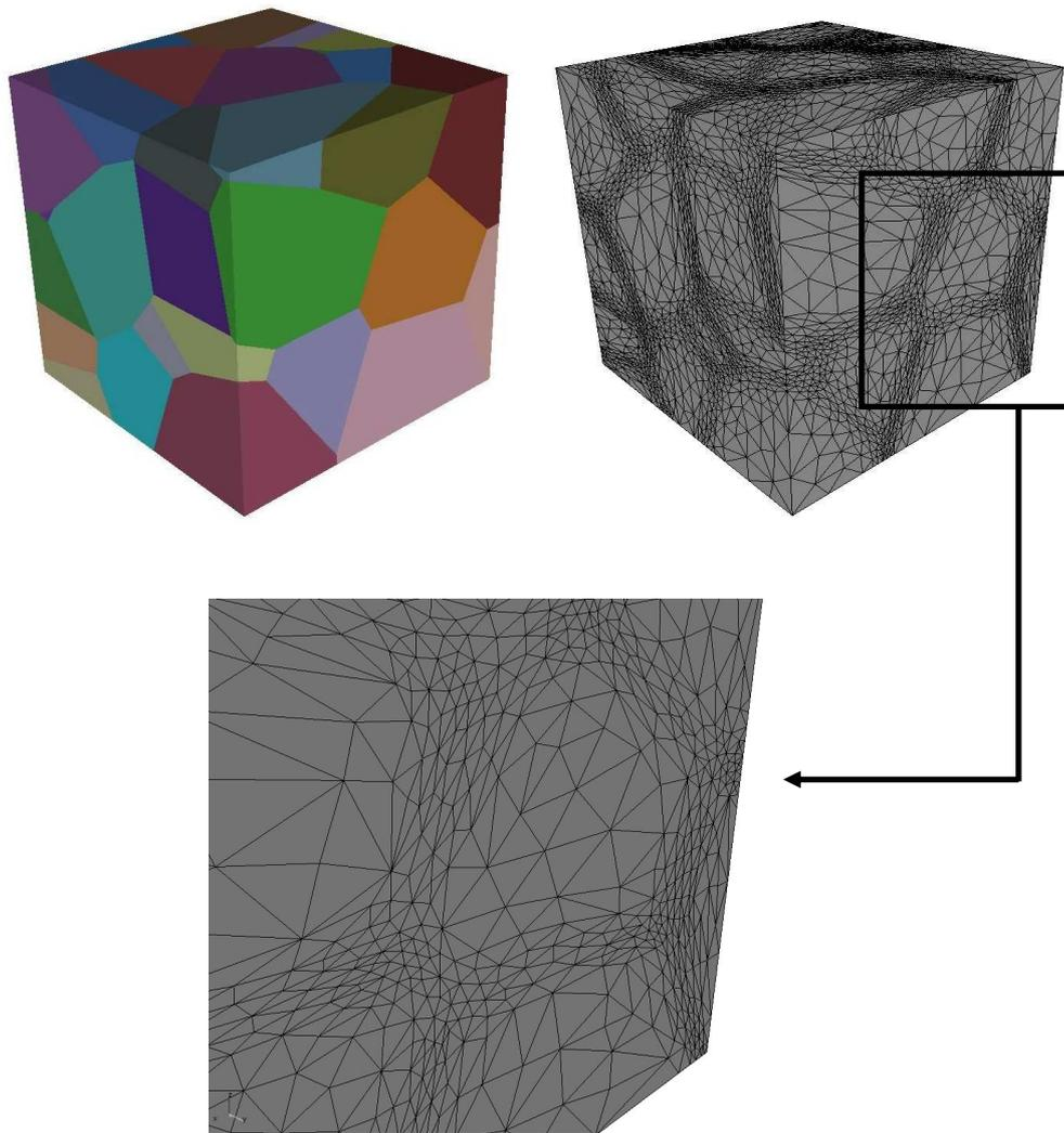
Figure 3 : A 50 grains microstructure and the corresponding finite element mesh (68 631 nodes, 385 494 elements). Anisotropic refining of the mesh is done close to the boundaries according to the  $\{\phi_i, 1 \leq i \leq 50\}$  distance functions, as detailed in the enlarged section (bottom).
