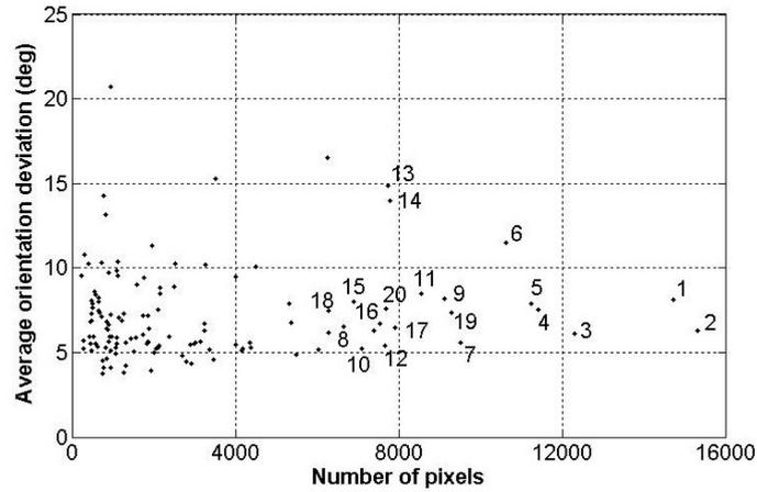
Fig. 6.27: Average orientation deviation as function of grain size (pixels) after deformation for the 129 grains obtained experimentally. The first 20 grains are labelled.
