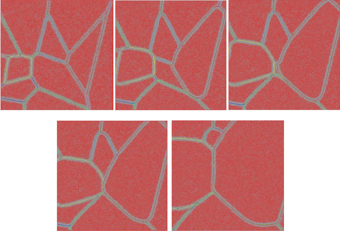
Figure 10 : microstructure evolution of a 12 grains aggregate
