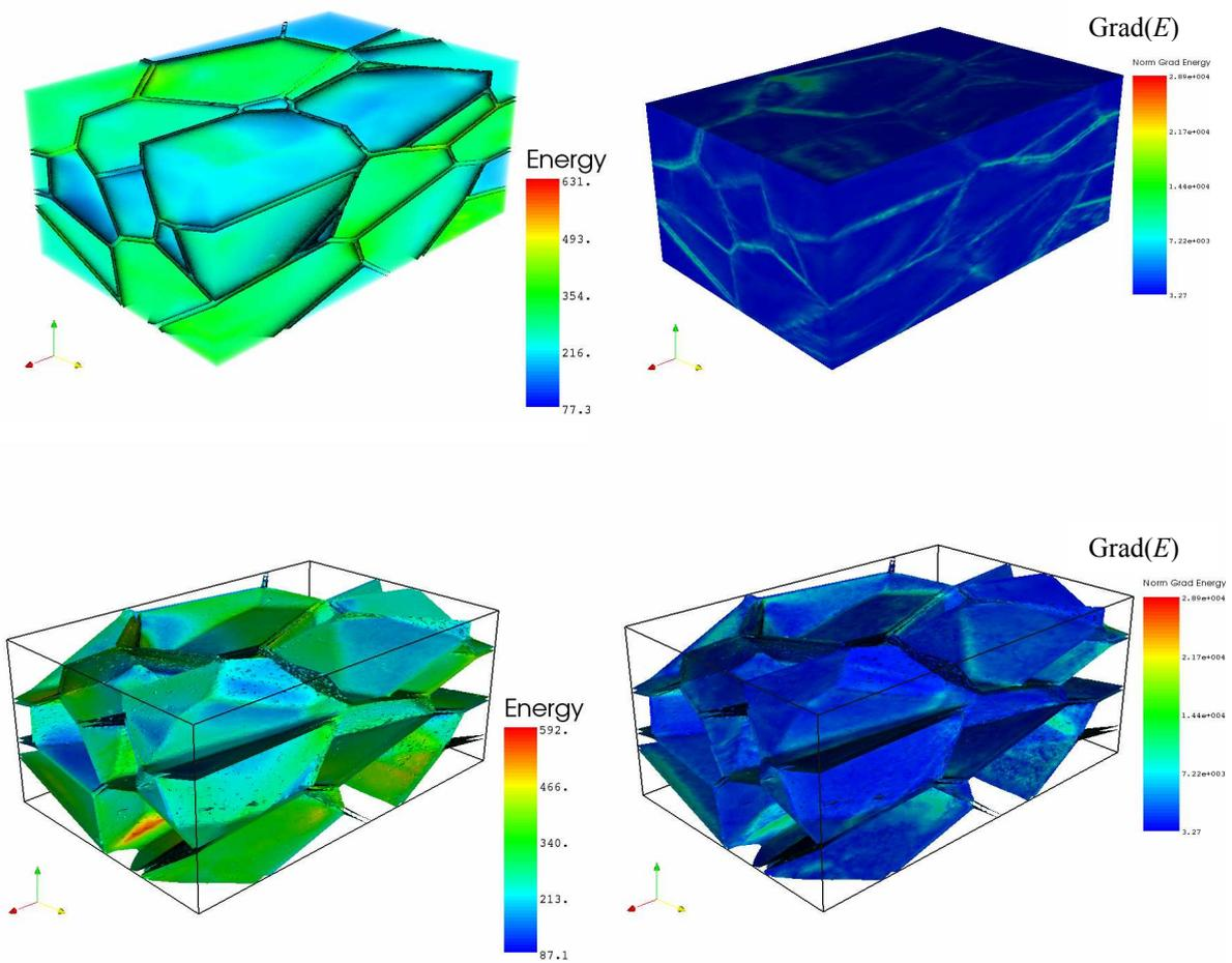
Figure 6 : Distribution of the stored energy  $E$  (left) and of the gradient of the stored energy  $\text{grad}(E)$  (right). Illustrations include the external surfaces of the 3D volume element (top) and internal grain boundaries identified as the zero level of the  $\{\phi_i, 1 \leq i \leq N_G\}$  functions (bottom).
