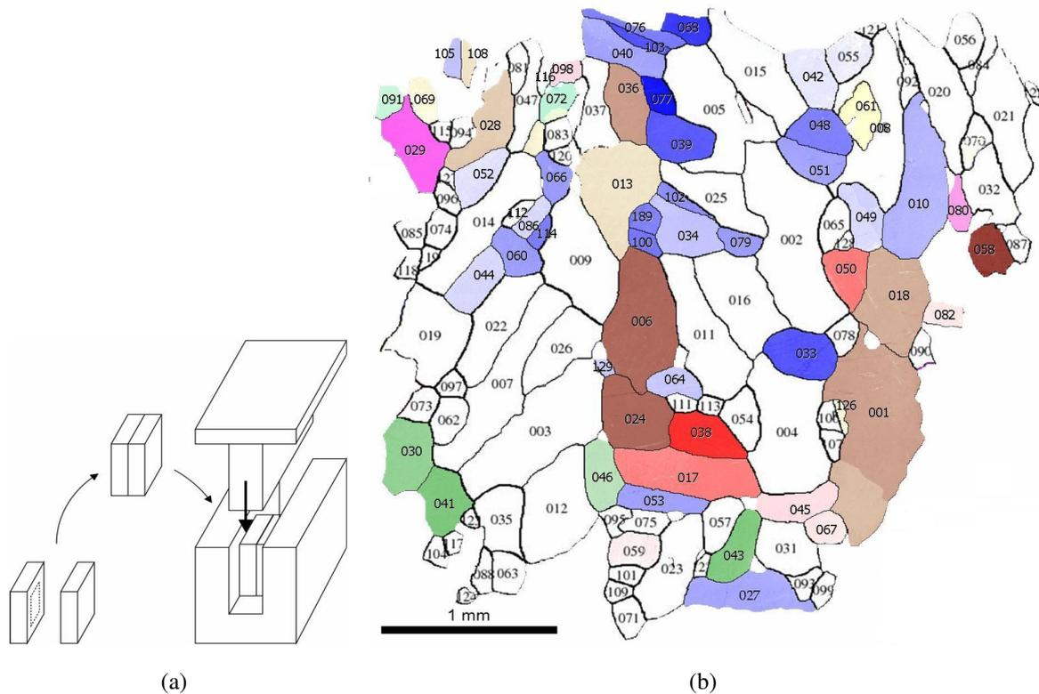
Fig. 6.13: Experimental setup and initial microstructure: (a) split sample in channel die compression; (b) grain structure in the undeformed state showing grain numbering. Grain boundaries ( $> 5^\circ$ ) are represented by black segments.
