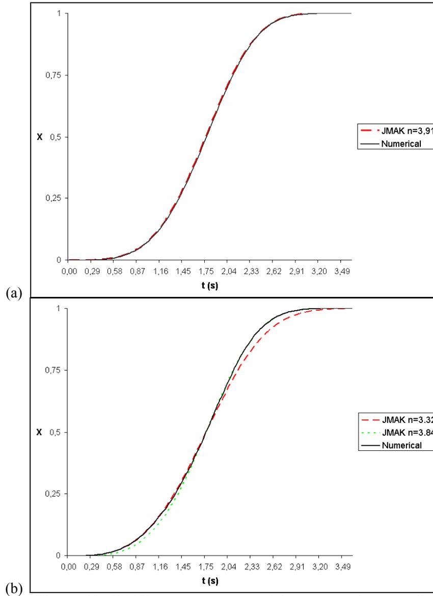
**Figure 12.** JMAK approximations of the numerical recrystallization kinetics extracted from Figure 11: (a) random choice of nucleation sites, low and constant nucleation rate of  $2 \cdot 10^{-4}$ ; (b) considering the non uniform stored energy field and choosing nucleation sites at highest values of  $\|\nabla E_n\|$ .
