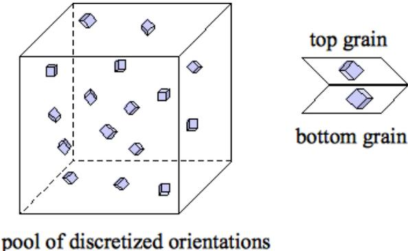
Fig. 3.2: Illustration of the LAMEL orientation selection procedure
