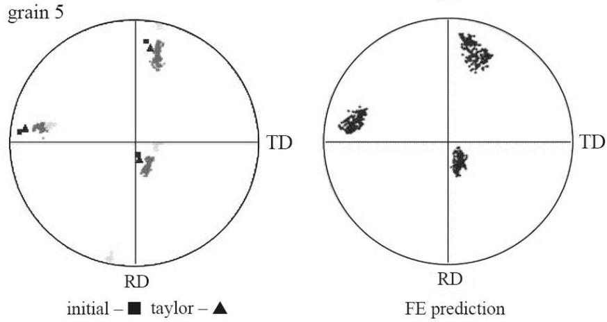
Fig. 6.3: (100) pole figures showing the initial orientation, the Taylor FC prediction and the cloud experimentally measured after 40 % plain strain compression on the left-hand side, and the finite element (FE) prediction after on the right-hand side for a particular grain [KALIDINDI et al., 2004]
