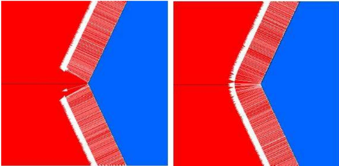
Figure 7 : Triple junction in 2D with a stored energy  $E$  lower in the grain on the right ( $E_1 = 1$ ) than in the two grains on the left ( $E_2 = E_3 = 2$ ). Representation of the velocity field with no smoothing (left), and with smoothing (right).
