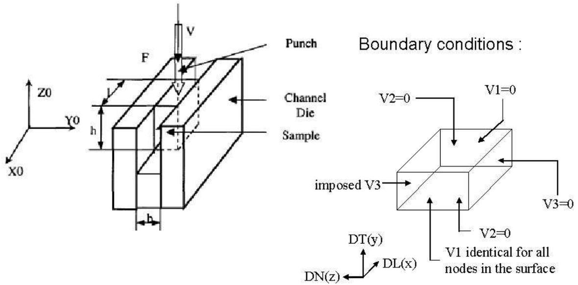
Figure 5 : Channel die test configuration and definition of boundary conditions
