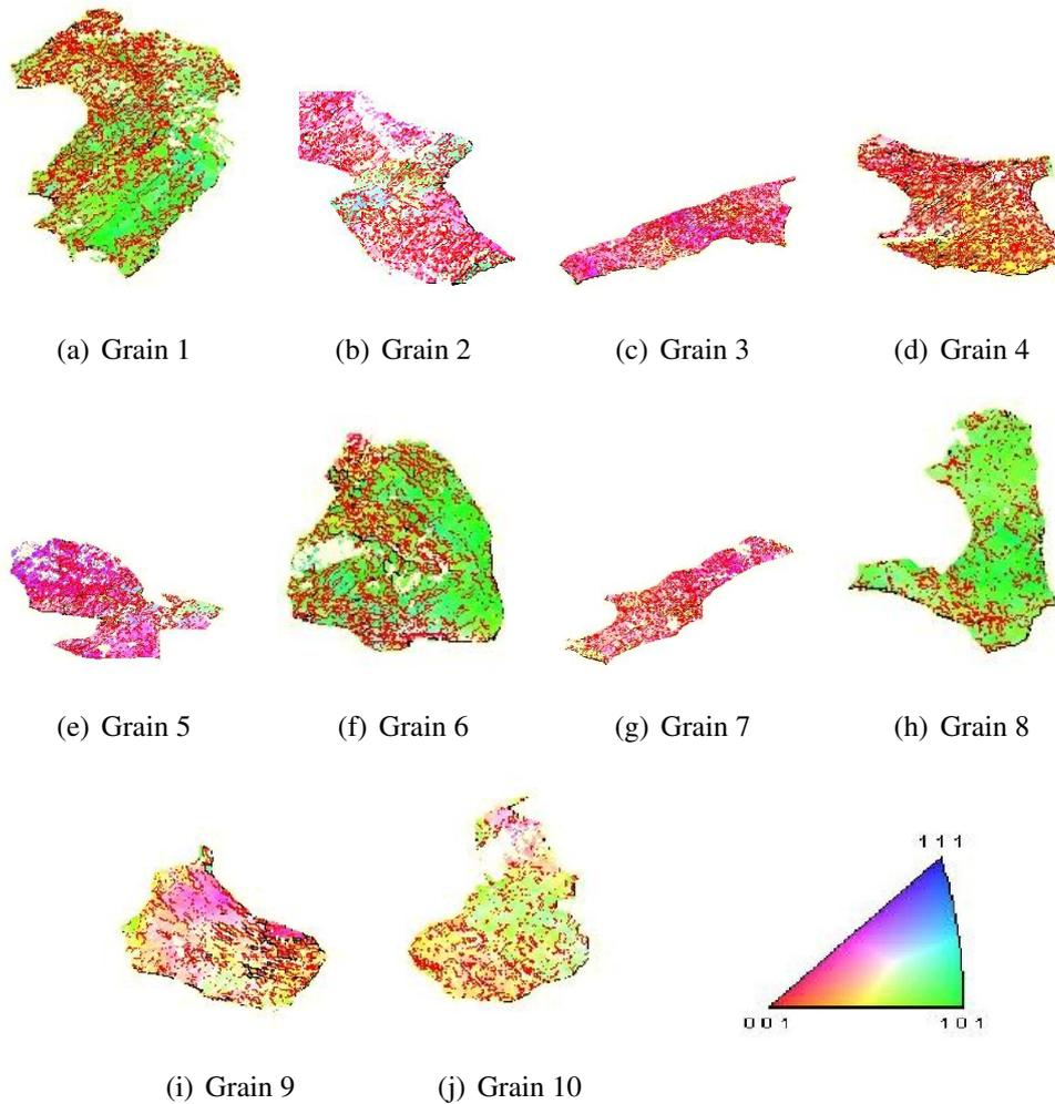
Fig. D.1: Experimental inverse pole figure (IPF) maps for sample normal axis for the first ten grains of the experimental microstructure in chapter 6. Black and red segments represent high angle ( $>15^\circ$ ) and low angle grain boundaries respectively ( $>5^\circ$ ).
