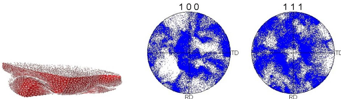
Fig. 4.20: Deformed mesh in the case of remeshing after 53.7 % true strain and the corresponding  $\{100\}$  and  $\{111\}$  pole figures.
