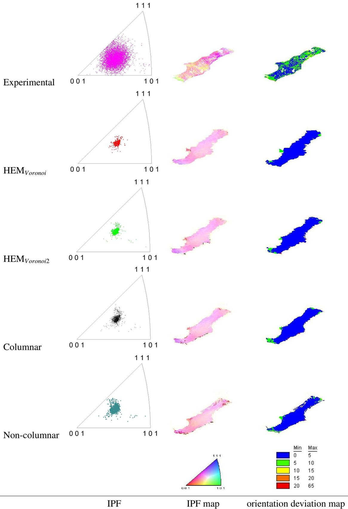
Fig. 6.50: Orientation deviation map and inverse pole figures (sample normal axis) for grain 7. Black and red segments in the IPF maps of the simulations represent high angle ( $>15^\circ$ ) and low angle grain boundaries respectively ( $>5^\circ$ ).
