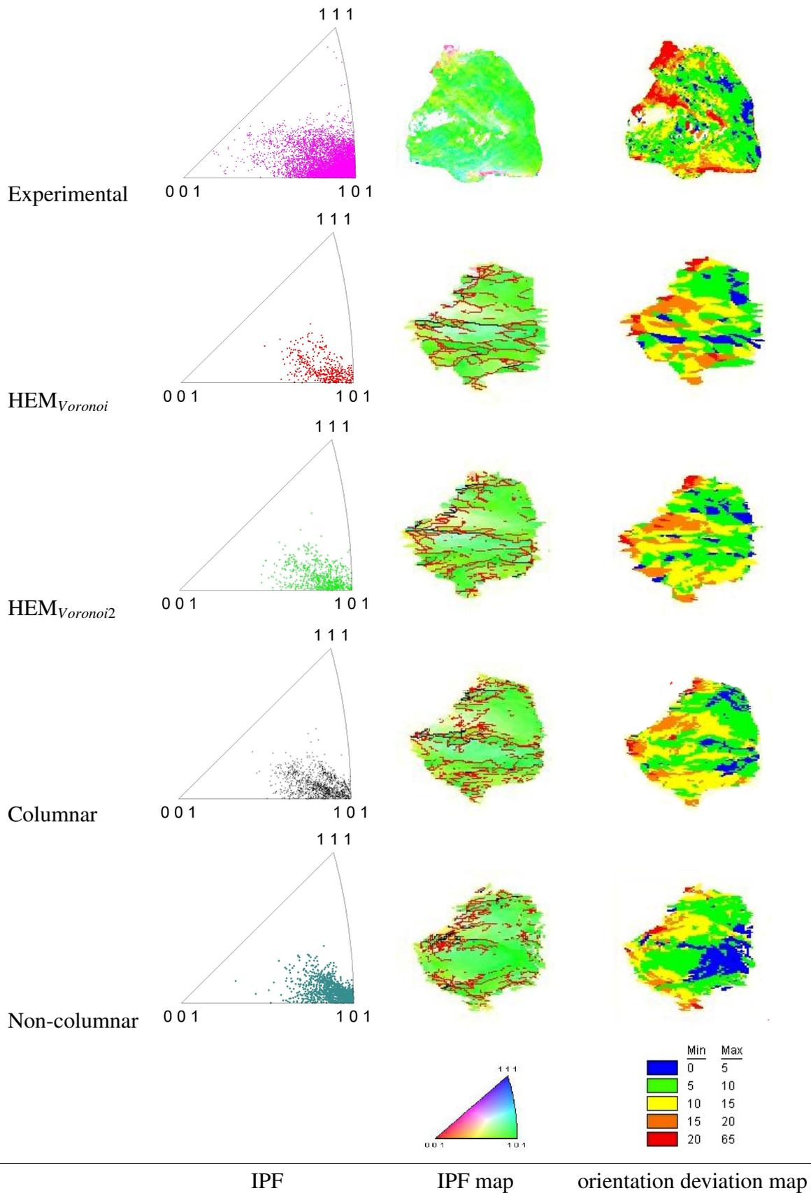
Fig. 6.49: Orientation deviation map and inverse pole figures (sample normal axis) for grain 6. Black and red segments in the IPF maps of the simulations represent high angle ( $>15^\circ$ ) and low angle grain boundaries respectively ( $>5^\circ$ ).
