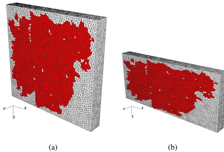
Fig. 6.18: (a) Initial mesh used in the slice case (207951 elements and 40682 nodes); (b) deformed mesh after  $\boldsymbol{\varepsilon} = 0.4$
