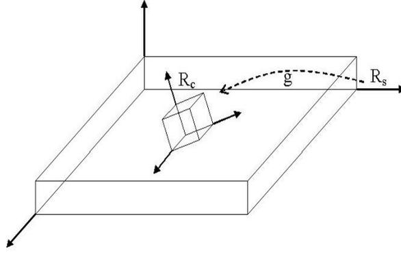
Fig. 6.1: Definition of the orientation of a crystal
