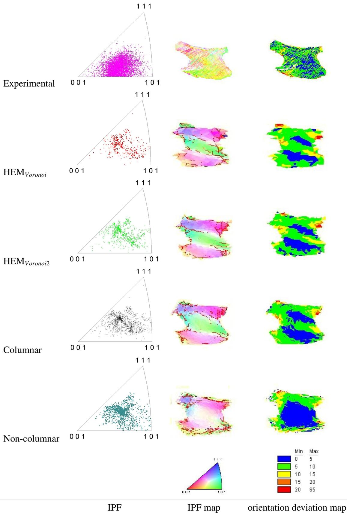
Fig. 6.47: Orientation deviation map and inverse pole figures (sample normal axis) for grain 4. Black and red segments in the IPF maps of the simulations represent high angle ( $>15^\circ$ ) and low angle grain boundaries respectively ( $>5^\circ$ ).
