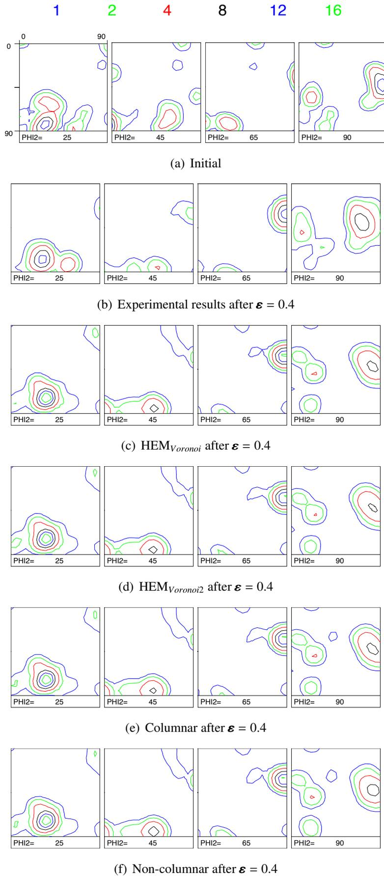
Fig. 6.35: ODF representing texture predictions obtained experimentally and numerically for different microstructures and mesh types ( $\varphi_2 = 25^\circ, 45^\circ, 65^\circ$  and  $90^\circ$ ).
