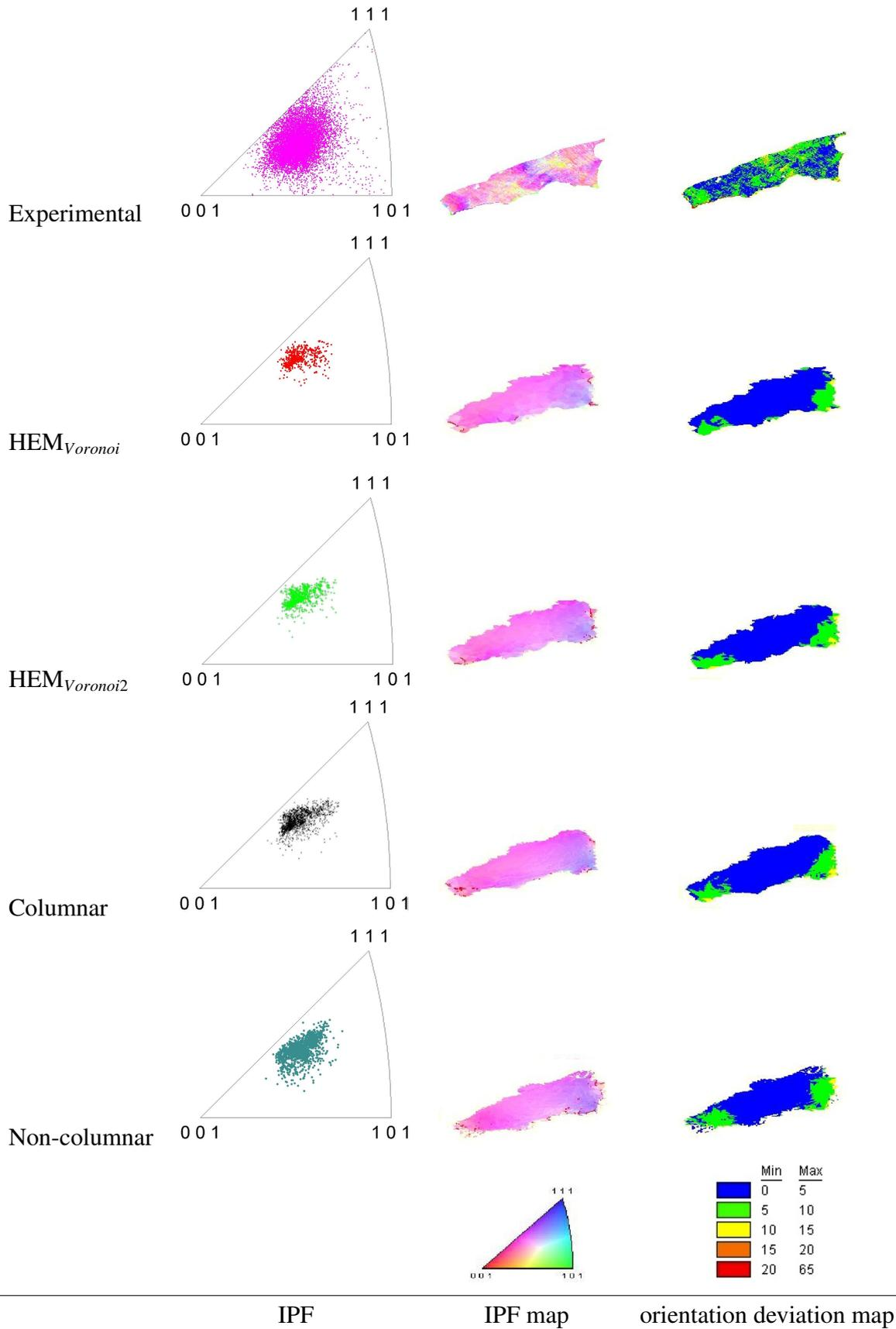
Fig. 6.46: Orientation deviation map and inverse pole figures (sample normal axis) for grain 3. Black and red segments in the IPF maps of the simulations represent high angle ( $>15^\circ$ ) and low angle grain boundaries respectively ( $>5^\circ$ ).
