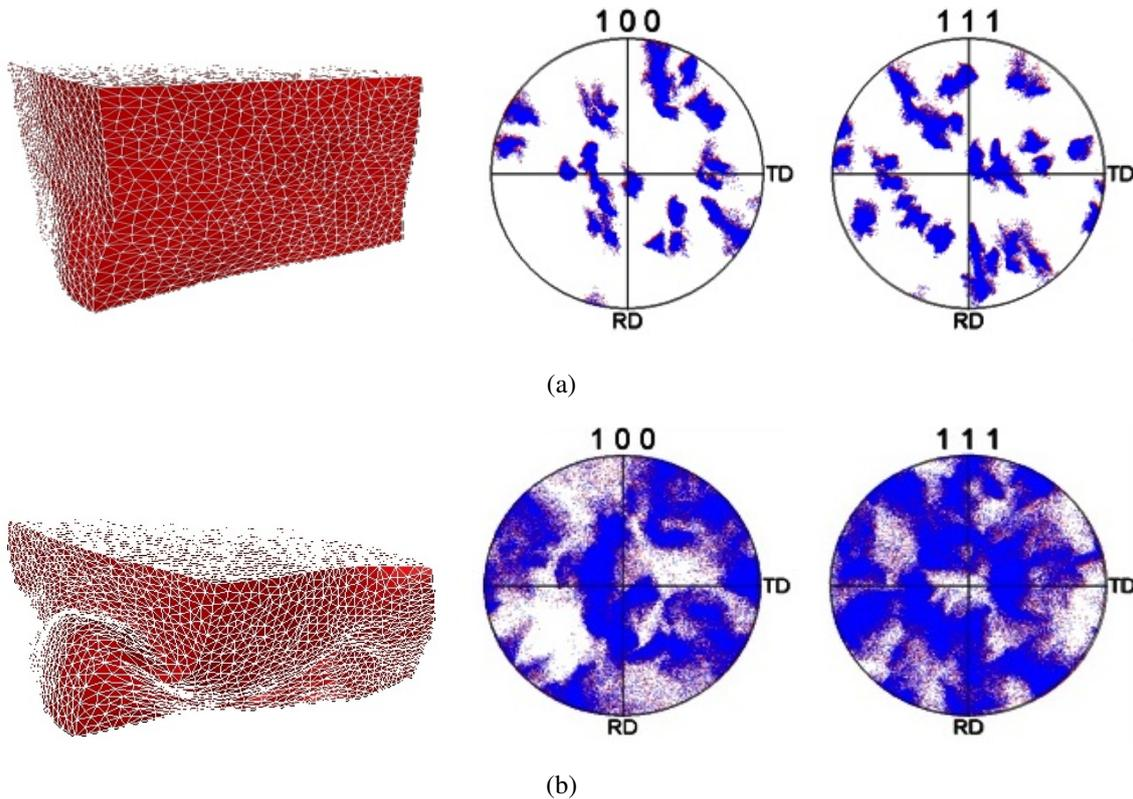
Fig. 4.19: Deformed mesh and the corresponding  $\{100\}$  and  $\{111\}$  pole figures: (a) after 12.5 % true strain; (b): after 42.5 % true strain. The pole figures with and without remeshing are superposed, the red being obtained without remeshing and the blue after remeshing.
