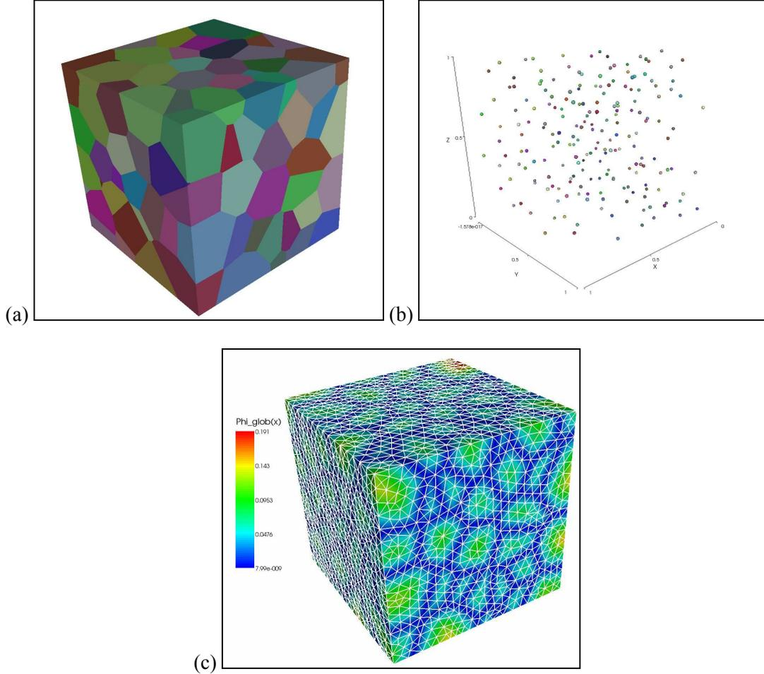
**Figure 2.** (a) A 200 grains virtual cubic microstructure; the color scale describes the identity of the different grains, (b) the corresponding Voronoi sites, (c) the corresponding  $\phi_{glob}(x)$  function for the finite element mesh, the latter appears in white.
