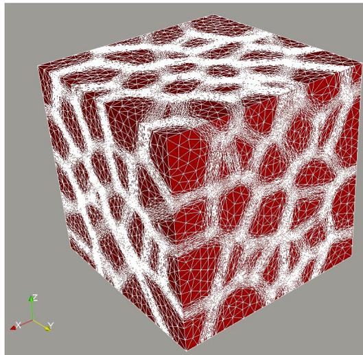
Fig. 4.15: A 300 grains polycrystal anisotropically meshed
