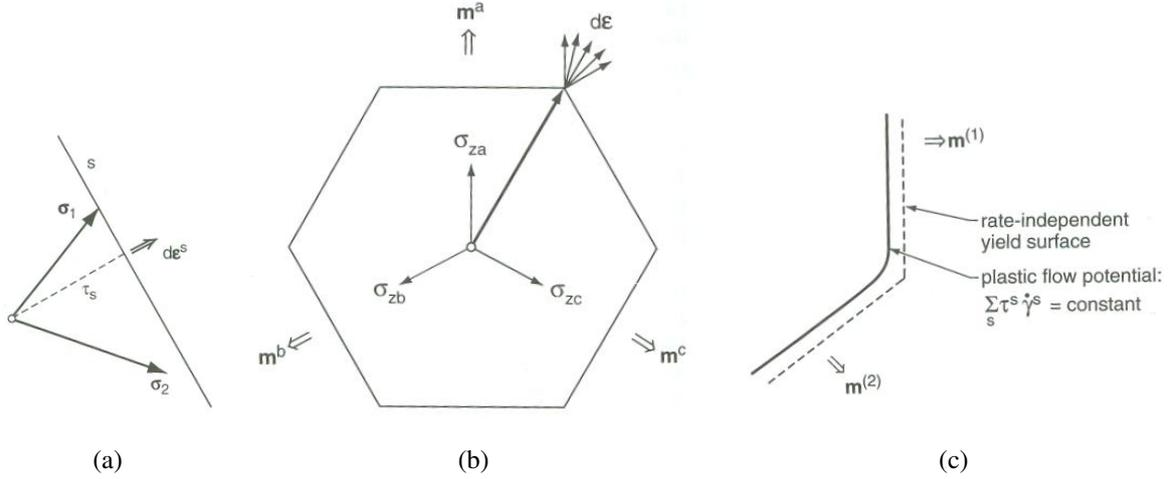
Fig. 2.3: 2D projection of yield surface in stress space (a) single slip representation; (b) multiple slip representation; (c) rate independent vs rate dependent plasticity [Kocks, 1998a]. Here  $s$  stands for slip system and  $m$  is the Schmid tensor
