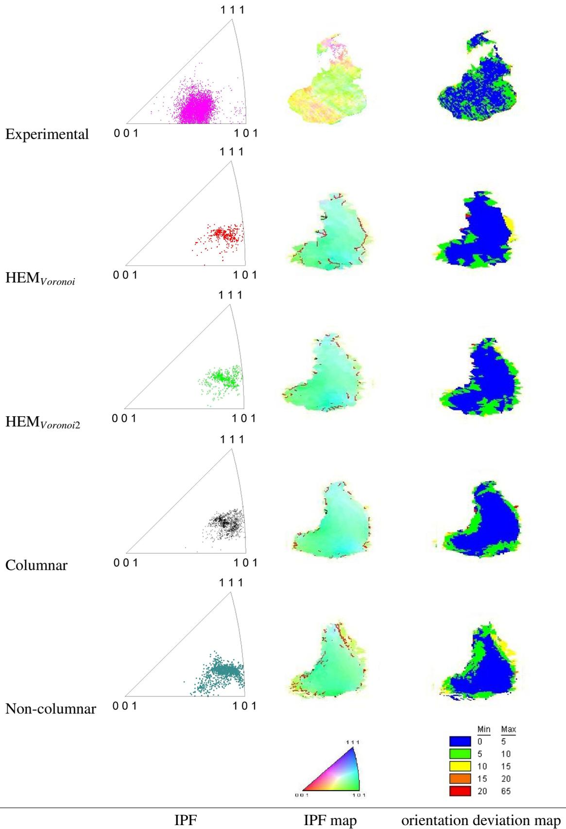
Fig. 6.53: Orientation deviation map and inverse pole figures (sample normal axis) for grain 10. Black and red segments in the IPF maps of the simulations represent high angle ( $>15^\circ$ ) and low angle grain boundaries respectively ( $>5^\circ$ ).
