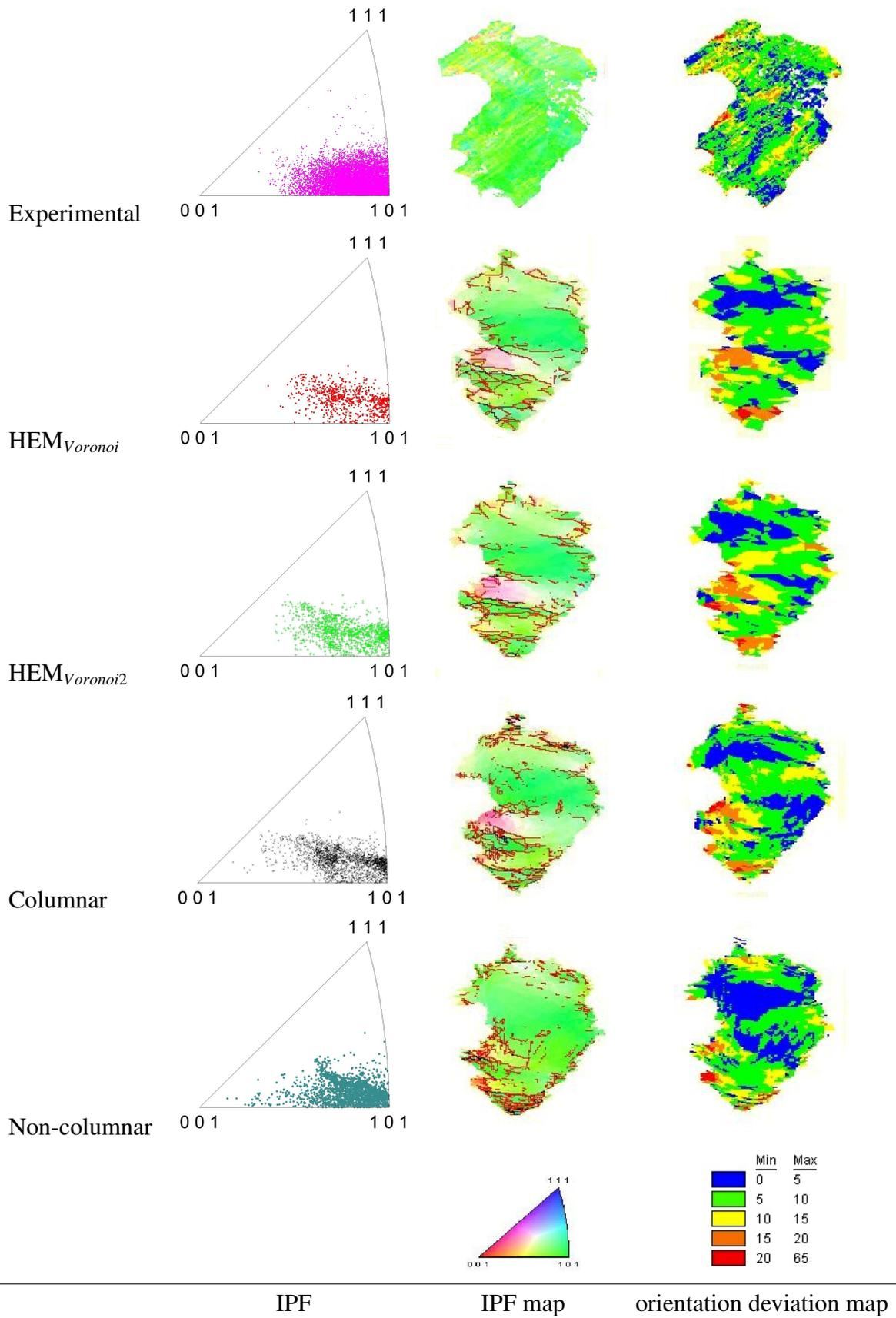
Fig. 6.44: Orientation deviation map and inverse pole figures (sample normal axis) for grain 1. Black and red segments in the IPF maps of the simulations represent high angle ( $>15^\circ$ ) and low angle grain boundaries respectively ( $>5^\circ$ ).
