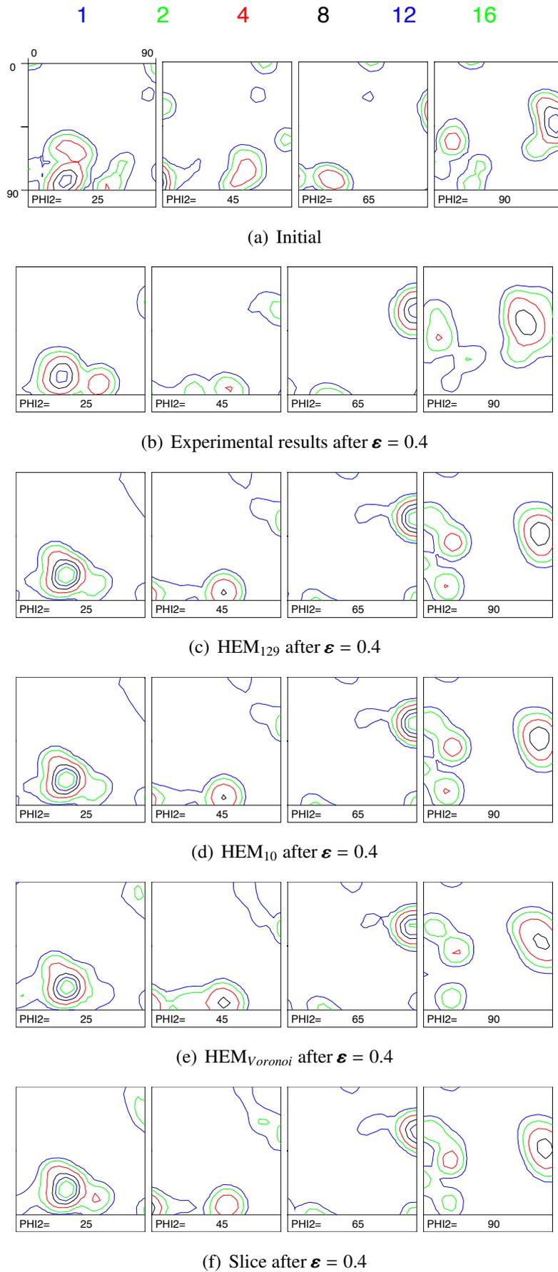
Fig. 6.21: ODF representing texture predictions obtained experimentally and numerically for different surrounding media ( $\varphi_2 = 25^\circ, 45^\circ, 65^\circ$  and  $90^\circ$ ).
