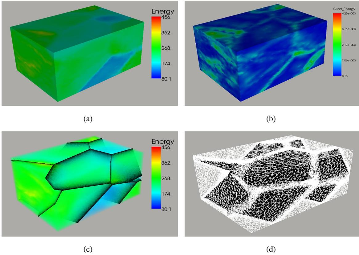
Fig. 5.13: A 3D ten grains microstructure after plastic deformation: (a) external surface view of stored energy, (b) corresponding norm of the stored energy gradient,(c)volumetric view of the stored energy with grain boundaries in black and (d) adaptive and anisotropic meshing in white, grain boundaries in black
