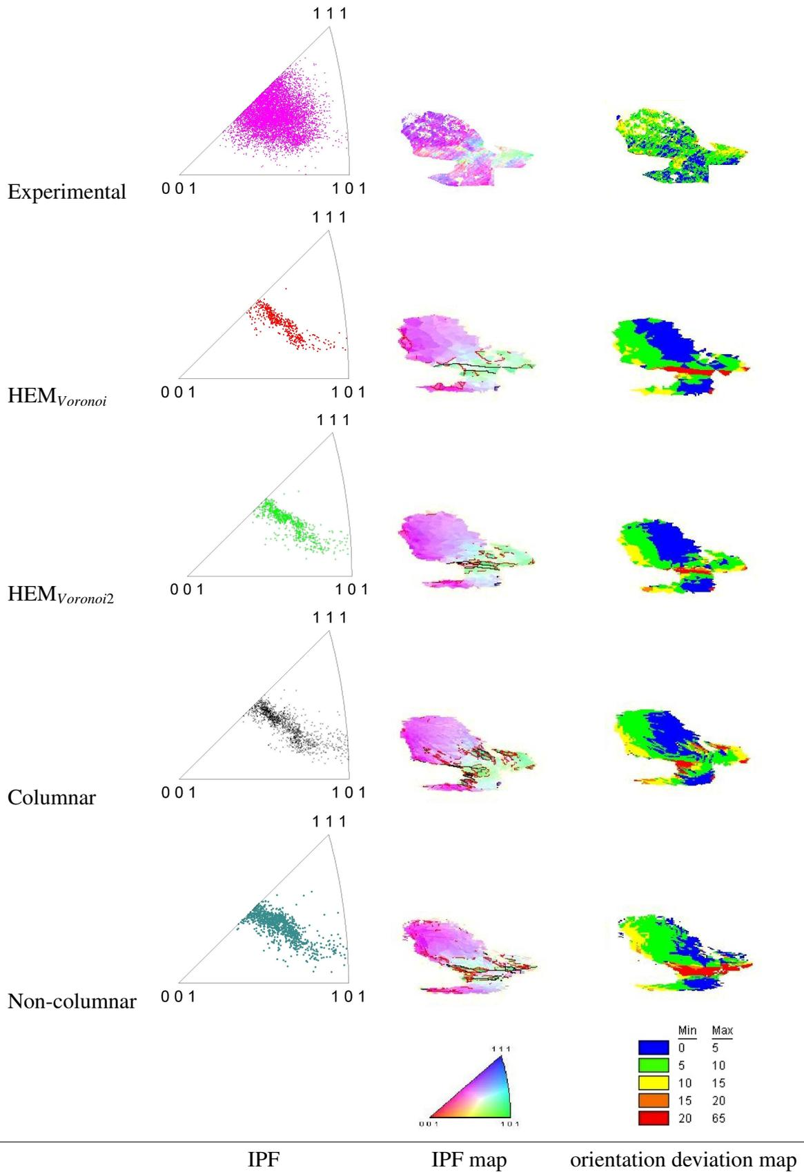
Fig. 6.48: Orientation deviation map and inverse pole figures (sample normal axis) for grain 5. Black and red segments in the IPF maps of the simulations represent high angle ( $>15^\circ$ ) and low angle grain boundaries respectively ( $>5^\circ$ ).
