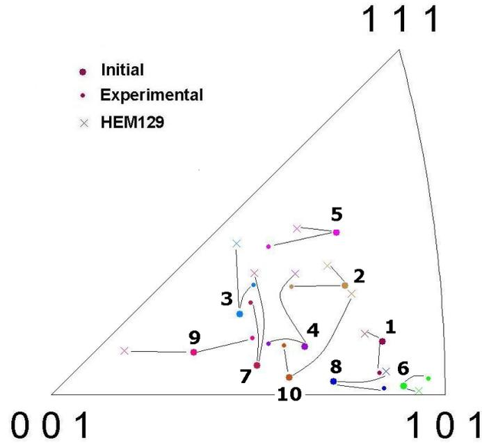
Fig. 6.30: Grain rotation paths (for the mean orientation) obtained experimentally and for the  $\text{HEM}_{129}$  case.
