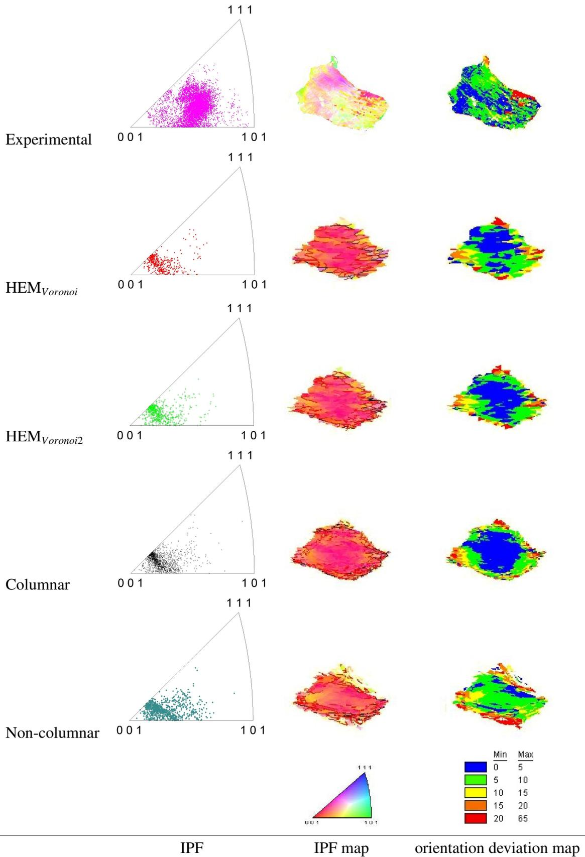
Fig. 6.52: Orientation deviation map and inverse pole figures (sample normal axis) for grain 9. Black and red segments in the IPF maps of the simulations represent high angle (>15°) and low angle grain boundaries respectively (> 5°).
