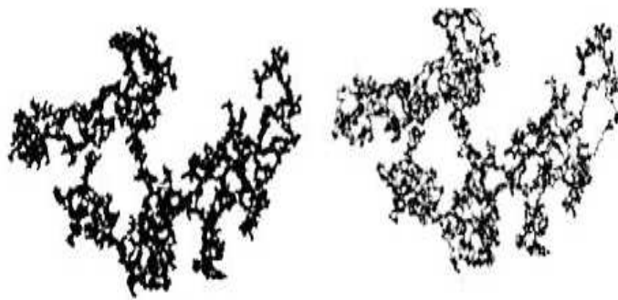
FIGURE 3.24 – Structure fractale en masse D_m = 1.82 [9]
