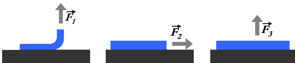
Figure 6 - Schematic representation of the peel ( F_1 ), shear ( F_2 ) and tensile ( F_3 ) forces that can be measured during an adhesion test.
