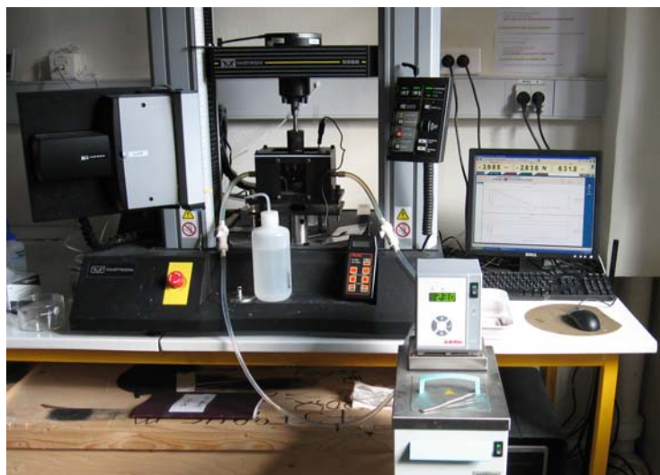
Figure 11 - Picture of the setup for underwater adhesion measurement adapted on the Instron 5565 machine.
