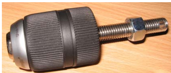
Figure 10 - Picture of the sample-holder of the punch. Based on a commercial mandrel of a drilling machine, it allows a tight junction between the load cell and the punch.
