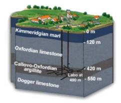
Figure 60: geological 3D model of the underground lab of ANDRA at Bure (ANDRA 2000).
