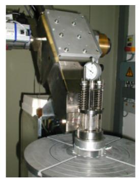
Figure 67: Sample holding device during a solution test under load in front of the X-ray  $\mu$ -focus source with a mechanical  $\mu$ -meter gauge to measure the strain.
