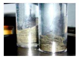
Figure 74 a), b): The left glass contains a 1.3 molar KCL solution. The other cylinder is filled with pure water G=56 nS. The KCL glass is completely covered with small gas bubbles and the sample does not disperse but cracked. Both glasses contain material from sample #05564, well 205.
