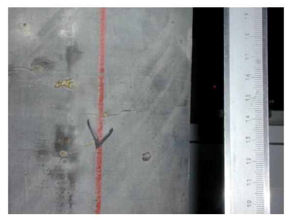
Figure 64: the core sample # 02517 from well 104 immediately after opening the storage device with radially propagated macroscopically visible cracks on the surface – most probably due to dehydration. The inhomogenities are clearly visible. The colour could also be interpreted as an indication of dehydration
