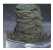
series 13: a), b), c):specimen #67, a) after 20 minutes in pure water at rehydrated state conditions (99% RH, 20 h, unloaded) and b) immediately after the glass cylinder was filled, at dehydrated state (5% RH, 20 h) and c) after 25 minutes
