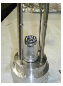
Figure 68: Device during preparation before a test with a solution (empty reservoir with sample and upper bearing.
