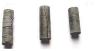
Figure 75: from left to right: specimen #1, #3 and #5, after immersion in a 2 molar KCl solution. The cracks in all three cases are in the direction of the bedding plane: 90° for #1, 0° for #3 and 45° for #5.
