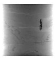
Series 9: specimen #28 in a 1,3 molar  $CaCl_2$  solution, immediately after the filling, after 16 minutes and after 45 minutes. The last image shows two main crack systems and many smaller cracks close to the bottom. Load =1.5 MPa, T =25°C, picture width = 16mm,  $\mu$ CR=22 $\mu$ m
