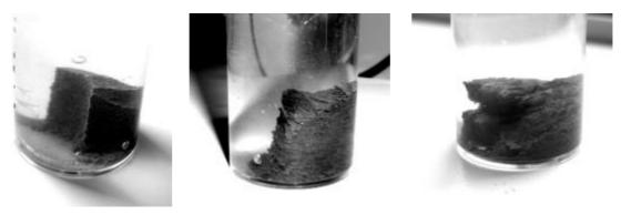
Figure 73 a), b), c): a) after immersion of the shale in pure water, b) after 10 minutes, c) the material dispersed completely after 20 minutes. The deterioration started in the stratification plane (sample #05564 well 205)
