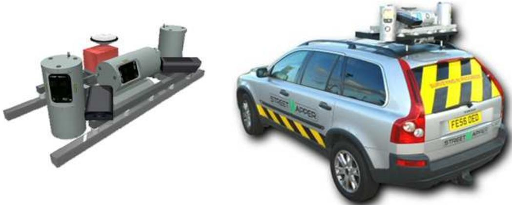
Figure 2-26 : StreetMapper, système de 3DLM (source [web 3DLM])
