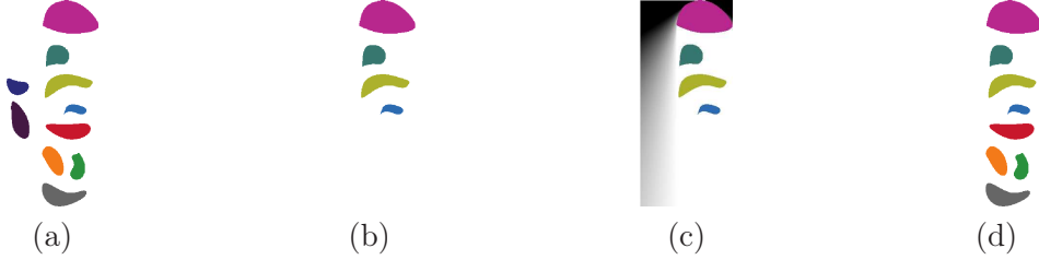
Figure 2.21: (a) Labeled image. (b) Locally aligned group. (c) The region seen by the group of (b) in the direction of the alignment (white = high value of visibility). (d) Group obtained after adding new elements.
