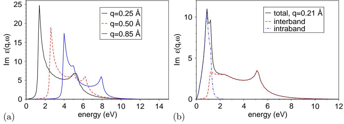
**Fig. C.1:** (a) The dielectric function  $\bar{\epsilon}$  of undoped graphite ( $d_0 = 3.35 \text{ \AA}$ ,  $E_F = 0 \text{ eV}$ ) for different in-plane momenta  $\bar{q}$  along the  $\Gamma K$  direction. Compare with [148, fig. 3(d)]. (b) The dielectric function  $\bar{\epsilon}$  of an stage-1 intercalated graphite compound ( $d_0 = 9.42 \text{ \AA}$ ,  $E_F = 0.75 \text{ eV}$ ) for an in-plane momentum  $\bar{q}$  along  $\Gamma M$ . Compare with [148, fig. 7(b)].
