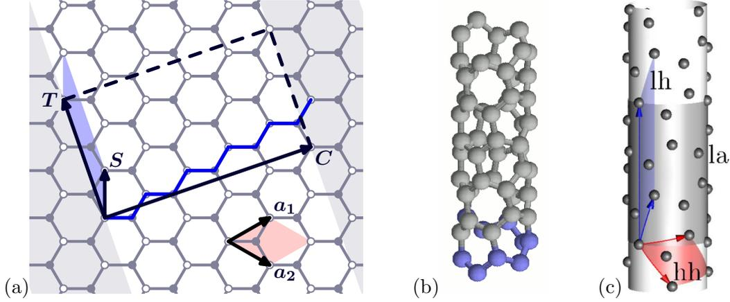
**Fig. 6.1:** Geometry of the chiral (4,1) nanotube. (a) Unit cell of the corresponding graphene-ribbon which is (b) rolled up into the nanotube. (c) Alternative choices for the unit cell of the tube: (la) linear-angular, (lh) linear-helical, and (hh) helical-helical unit cell.
