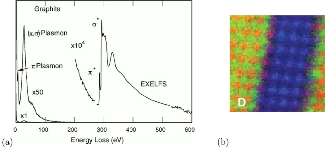
**Fig. 1.3:** STEM measurements. (a) Electron energy-loss spectrum for graphite in the valence- and core-loss region (Reprinted from [24], Micron © 2008, with permission from Elsevier). (b) An atomic-resolution elemental map of a multilayer system. Colours indicate different edge signals attributed to La (green), Ti (blue), and Mn (red) atoms (Reprinted by permission from Macmillan Publishers Ltd: [Nature Materials](#) [15], © 2009).
