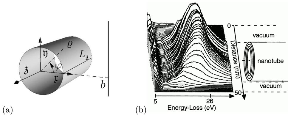
**Fig. 7.4:** (a) Geometry of the STEM measurements scanning across an isolated nanotube. (b) Experimental valence EEL spectra for an isolated multi-wall carbon nanotube (Reprinted from [173], Journal of Electron Spectroscopy © 2001, with permission from Elsevier).
