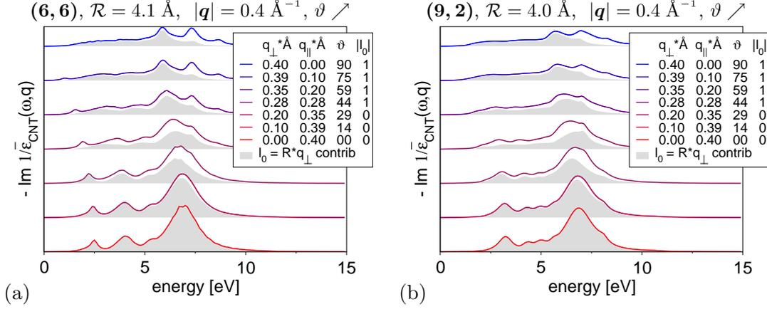
**Fig. 6.13:** Dependence of the loss function on the direction of the momentum transfer  $q = 0.4 \text{ \AA}^{-1}$ . We compare an (a) armchair and (b) chiral nanotube with similar radius  $\mathcal{R} \approx 4 \text{ \AA}$ .
