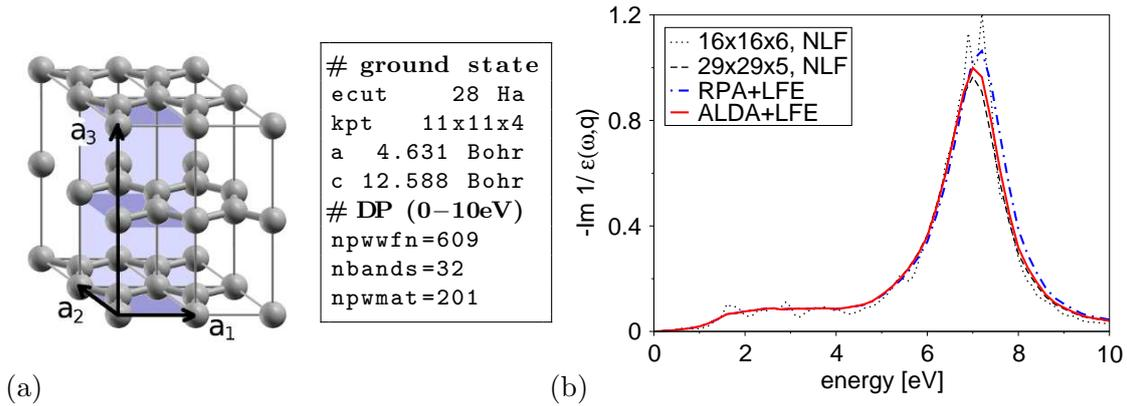
**Fig. 3.5:** (a) Unit cell (blue) and converged parameters for graphite (Bernal stacking). (b) Calculated loss function for graphite at small in-plane momentum  $q = 0.2 \text{ \AA}^{-1}$ . Two  $k$ -point samplings, calculations with and without LFE, and different TDDFT kernels  $f_{XC}$  are compared.
