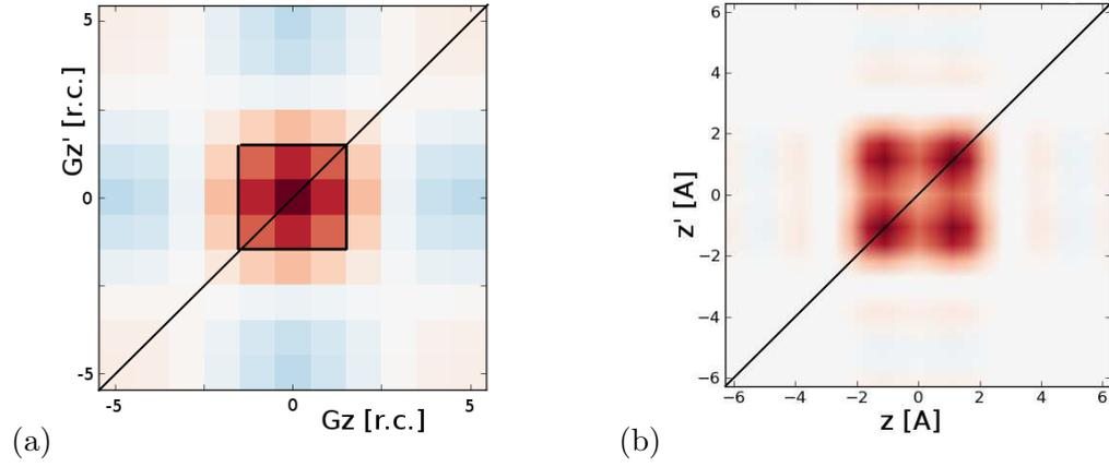
**Fig. C.2:** Independent-particle polarisability for a graphene stack with doubled interlayer distance  $d = 2d_0$ . (a) First, in reciprocal space  $\text{Im} \chi^0(\bar{q}\bar{q}'; G_z G'_z)$  and (b) second, in real space  $\text{Im} \chi^0(\bar{q}\bar{q}'; z z')$ . The other parameters are fixed as  $\bar{q} = \bar{q}' = 0.27 \text{\AA}^{-1}$ ,  $\omega = 4 \text{eV}$ .
