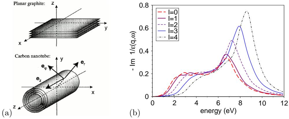
**Fig. 6.4:** (a) Model dielectric function of a multi-wall CNT. The dielectric tensor of graphite has been projected onto a cylinder. From [37]. (b) Tight-binding calculation for the loss function  $-\text{Im} \bar{\epsilon}_{\text{CNT}}^{-1}$  of a (23, 0) SWCNT for  $p = 0.2 \text{ \AA}^{-1}$  and different angular momenta  $l$ .
