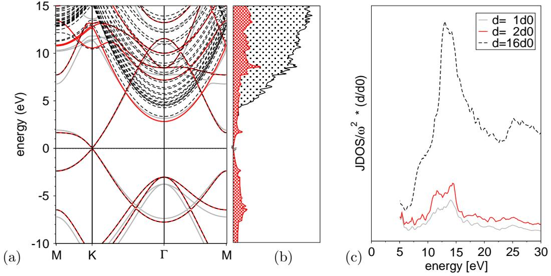
**Fig. 5.19:** (a) The Kohn-Sham bandstructure at  $k_z = 0$ , (b) the corresponding DOS and (c) JDOS for perpendicular polarisation  $q_z$  are compared for graphene stacks with different interlayer distances  $d$ . The contribution of free-electron states clearly vanishes for small supercell size  $d$ .
