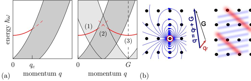
**Fig. 4.2:** (a) Excitation spectrum of free electrons (left) and electrons in a weak periodic crystal potential (right). Shaded regions indicate electron-hole excitations, thick, red lines the plasmon dispersion (adapted from [120]). (b) Visualisation of crystal local-field effects as induced dipoles (left) or Bragg reflected waves (right). See text.
