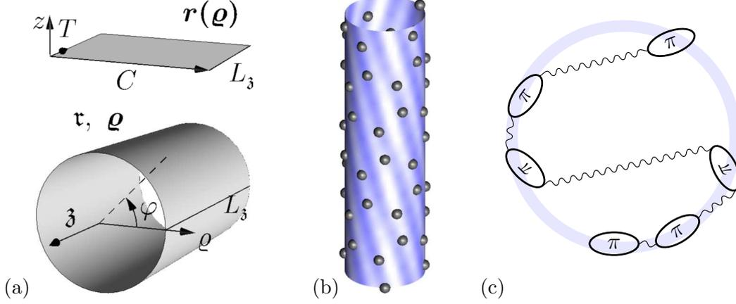
**Fig. 6.5:** Zone-folding for the microscopic polarisability. (a) Geometry of the cylinder and the unrolled graphene sheet. (b) Surface mode in a (4, 1) nanotube for a helical momentum  $\xi = (l, p)$  with angular projection  $l=10$  and on-axis part  $p=10 \text{ \AA}^{-1}$ . (c) Non-locality of the susceptibility.
