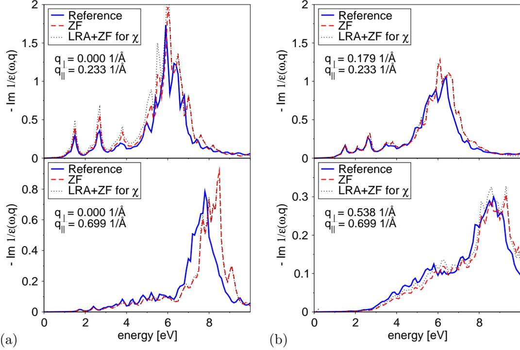
**Fig. 6.16:** Dielectric response of a (9,9) tube for (a) on-axis momentum transfer and (b) arbitrary direction of  $\mathbf{q}^0$  with small (top) and large magnitude (bottom). We compare full *ab-initio* calculations (solid, [187]) with the ZF results including (dashed lines) or excluding contributions of in-plane LFE (dotted lines). Compare with ZF+LRA results shown in fig. 6.8 and 6.10.
