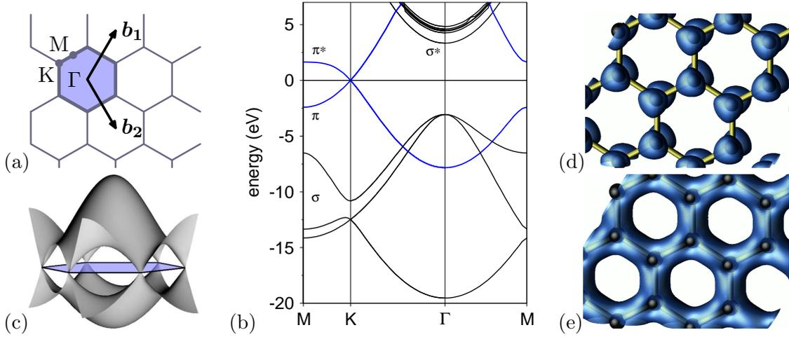
**Fig. 5.2:** (a) Brillouin zone of graphene in reciprocal space. (b) Electronic band structure of graphene. The  $\pi$  bands (blue) are also shown for the full Brillouin zone in (c). Partial-charge densities of a state at the  $\Gamma$  point for the  $\pi$  band (d), and the  $\sigma$  band (e).
