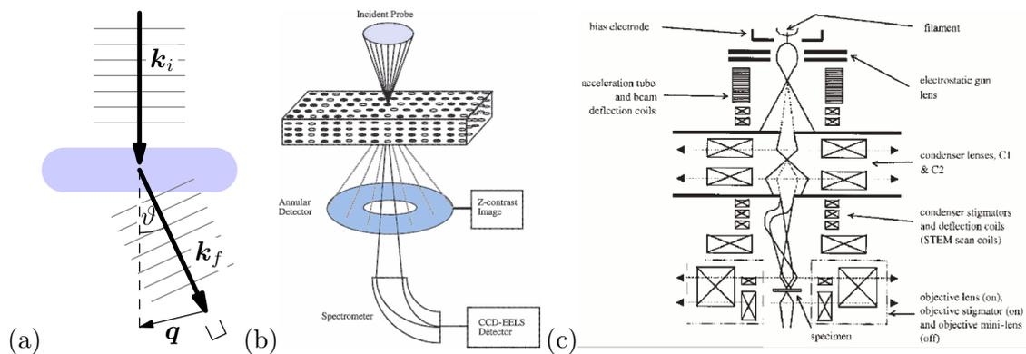
**Fig. 1.2:** (a) Geometry of an angular-resolved EELS experiment, (b) a scanning transmission electron microscope (STEM) and (c) a sketch of its experimental realisation. (Reprinted from [19] with permission from John Wiley & Sons Inc. © 2006).
