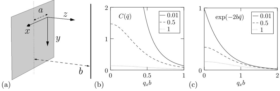
**Fig. 7.1:** (a) Geometry for the SR-EELS calculation in a planar sheet. (b) Probe factor  $C(q_x)$  for three different parameters  $\zeta = \frac{b\omega}{v}$  [see eq. (7.7)]. (c) Exponential  $e^{-2\bar{q}b}$  for the same parameters.
