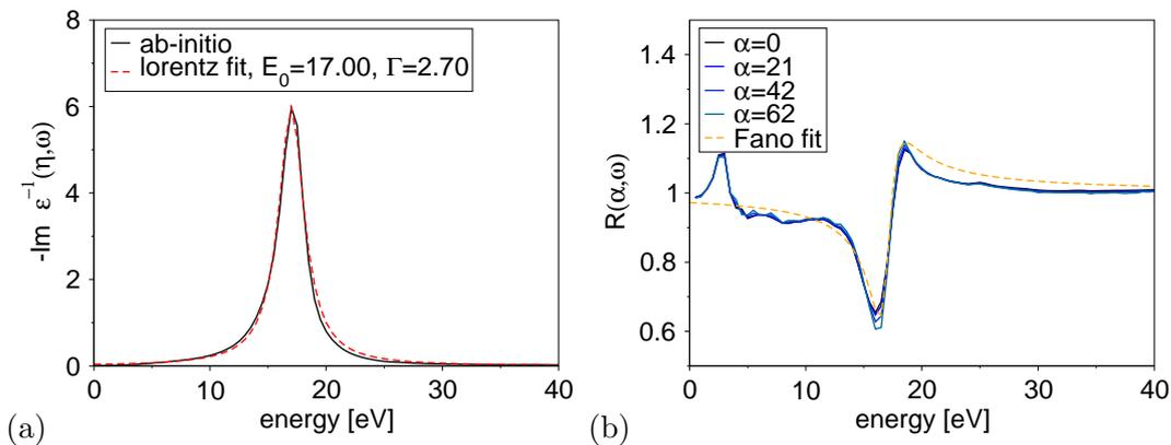
**Fig. 4.9:** Analysis of the Fano line shape. (a) Lorentz fit for the plasmon resonance at low momentum transfer. (b) Fano fit for the loss function at large momentum transfer close to the  $(1, 1, 1)$  reflection (see text). We used the  $2 \times 2$  model dielectric function  $\tilde{\epsilon}^{\text{NLF}}$  calculated in RPA.
