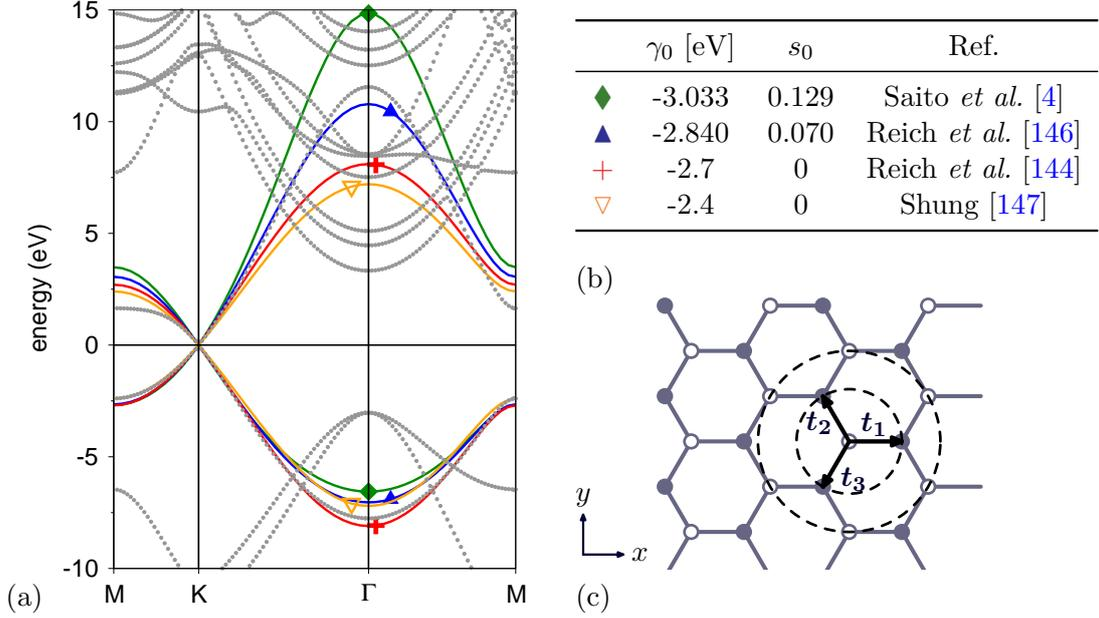
**Fig. 5.5:** Tight-binding bandstructure of graphene in nearest-neighbour approximation. (a) The  $\pi$  bands (lines) are calculated from eq. (5.14) for different parameters  $\gamma_0$  and  $s_0$  taken from literature (b). For comparison, an *ab-initio* bandstructure (dots) of LDA Kohn-Sham energies is shown. (c) Nearest and second-nearest neighbours of the A atom.
