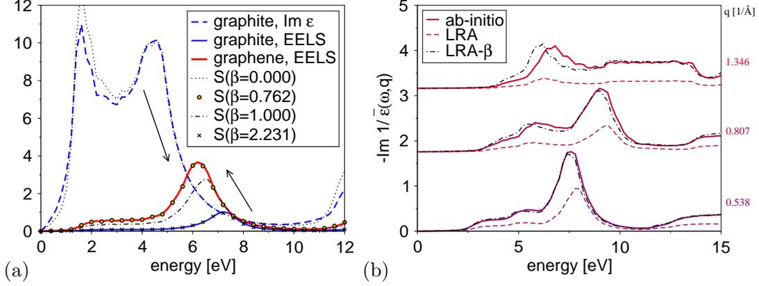
**Fig. 5.13:** (a) Comparison of graphite and graphene spectra for  $q=0.269 \text{ \AA}^{-1}$  with the generalised spectra  $\mathcal{S}_\beta$  for different parameters  $\beta$  (see text). (b) Best fit of the generalised spectrum  $\mathcal{S}_\beta$  (dash-dotted line) to the *ab-initio* graphene loss function (solid lines) for large momentum transfers. The LRA result, i. e.,  $\mathcal{S}_1$  is shown for comparison (dashed lines).
