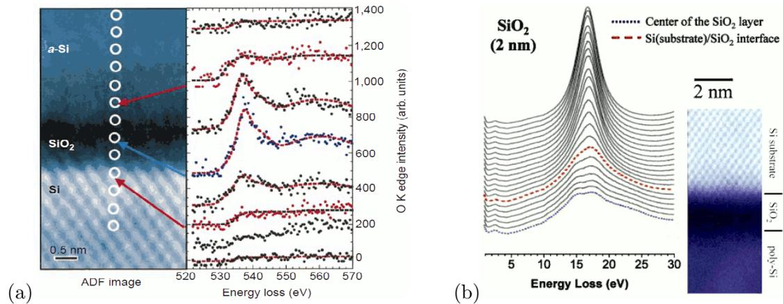
**Fig. 1.4:** Experimental EEL spectra from a STEM measurement scanning across a Si/SiO<sub>2</sub> interface. (a) The background-corrected oxygen K-edge (Reprinted by permission from Macmillan Publishers Ltd: [Nature](#) [31], © 1999) and (b) the valence-loss signal are shown for different positions across the interface (Reprinted from [32], © 2008 by The American Physical Society).
