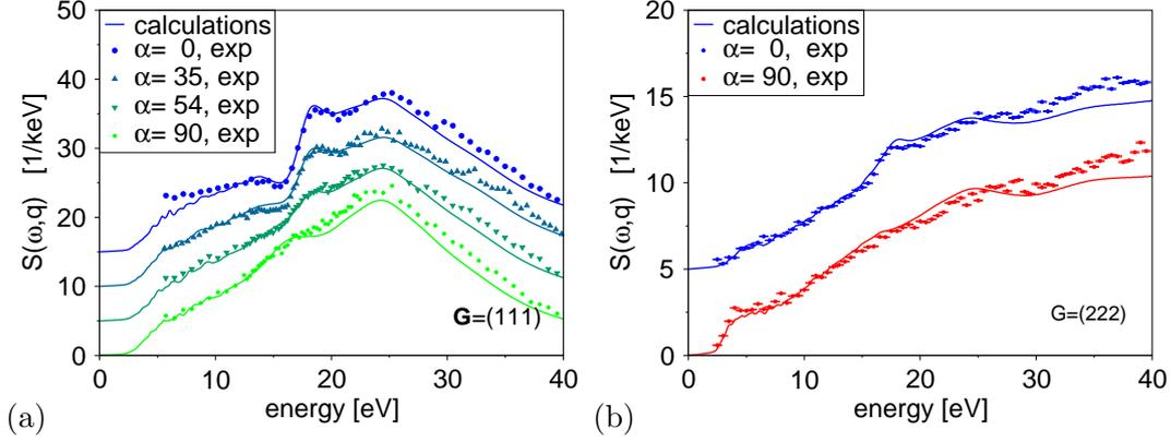
**Fig. 4.11:** Experimental verification of the angular anomaly in silicon. We compare IXS measurement (dots) and ALDA+LT calculations (solid lines) for loss functions close to the (a) (111) and (b) (222) reflections. The exact momentum transfers are given in fig. 4.1. The experimental curves have been scaled by a factor of 5 and 7 in (a) and (b), respectively. All curves are shifted for better visibility.
