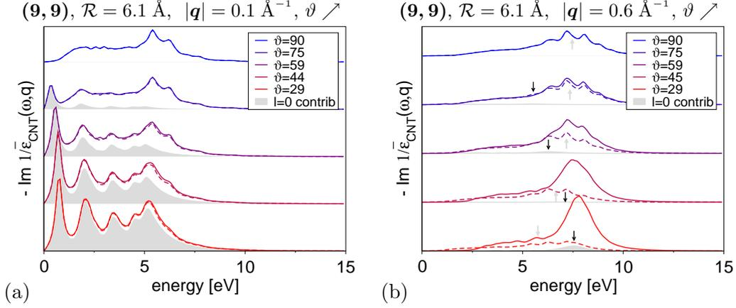
**Fig. 6.14:** Loss function of a (9,9) tube (solid) and the sum of perpendicular and parallel contribution (dashed) for (a) small  $q = 0.1 \text{ \AA}^{-1}$  and (b) large  $q = 0.6 \text{ \AA}^{-1}$  and different orientations  $\vartheta$ .
