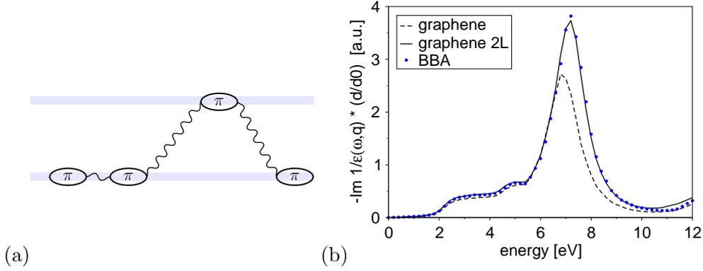
**Fig. 5.16:** (a) Coulomb interaction between sheets. (b) Loss spectrum of single- (dashed line) and double-layer graphene (solid line) for in-plane momentum transfer  $q = 0.41 \text{ \AA}^{-1}$ . The dots correspond to the result from the building-block approach (see text).
