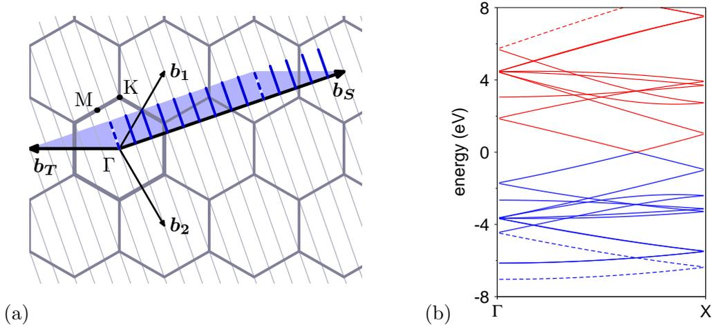
**Fig. 6.2:** Zone-folding for the chiral (4,1) nanotube. (a) Superposition of the reciprocal space of graphene (plane) and the nanotube (cutting lines). The Brillouin zone of the tube is spanned by  $\mathbf{b}_T$  and  $\mathbf{b}_S$  and contains  $N$  parallel line segments (blue) of length  $2\pi/T$ . (b) Tight-binding bandstructure of the (4,1) tube within the zone-folding model ( $\gamma_0 = -2.84$  eV,  $s_0 = 0.07$ ).
