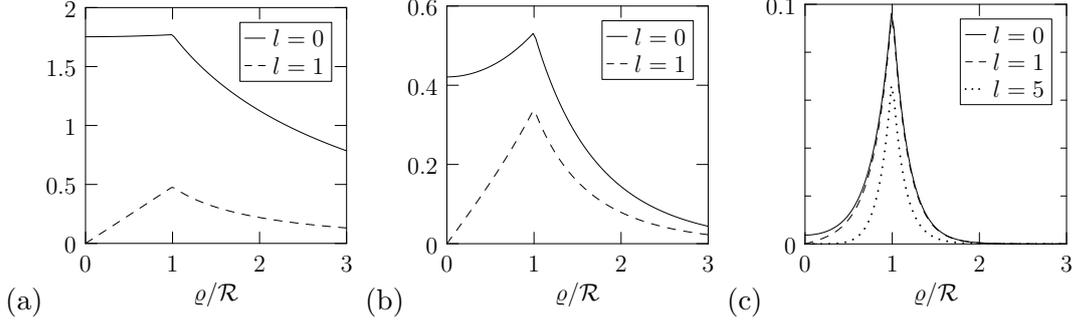
**Fig. 6.6:** Behaviour of the Coulomb potential  $\frac{\epsilon_0}{\epsilon} v(lp; q, q')$  for fixed radius  $q' = \mathcal{R}$  and increasing on-axis momentum transfers from left to right: (a)  $p = 0.2/\mathcal{R}$ , (b)  $p = 1/\mathcal{R}$ , and (c)  $p = 5/\mathcal{R}$ .
