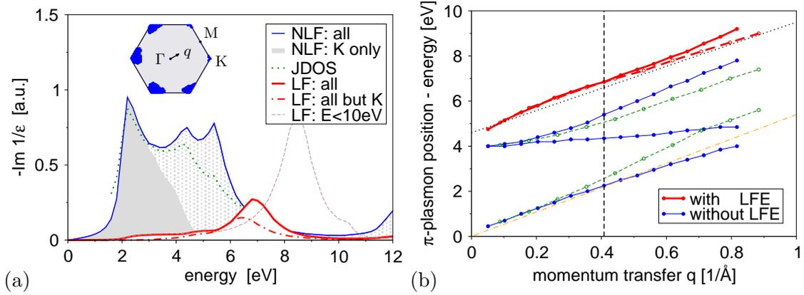
**Fig. 5.9:** (a) Loss function of graphene at  $q = 0.41 \text{ \AA}^{-1}$  along  $\Gamma M$  calculated from the JDOS (dots), within the bare RPA (blue) and in RPA including LFE (red, thick). The latter changes significantly, when transitions next to the K point (shaded area, see inset) are excluded (red, dot-dashed). (b) Dispersion of the peaks in the loss function for different momenta along  $\Gamma M$  (solid lines) and  $\Gamma K$  (dashed lines).
