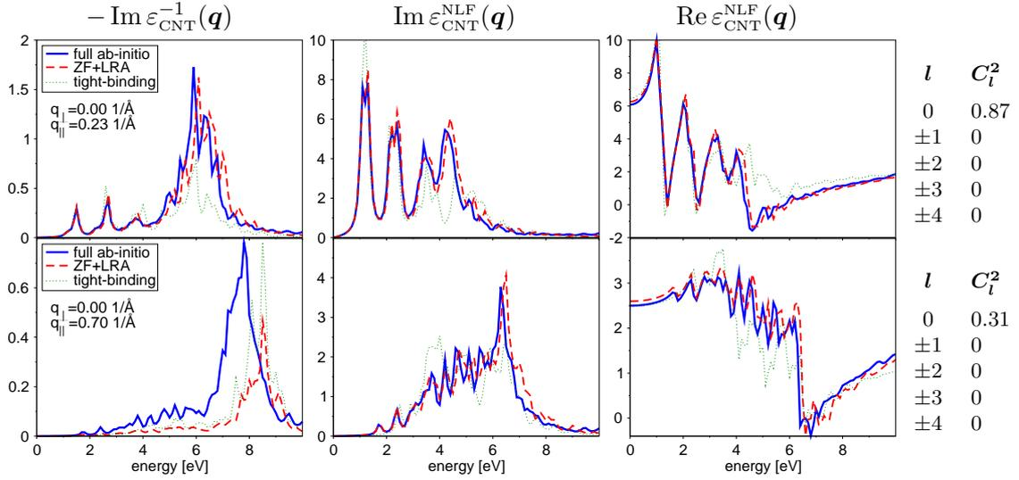
**Fig. 6.8:** AR-EEL spectra (left) and dielectric function  $\varepsilon_{\text{CNT}}^{\text{NLF}}(\mathbf{q}) = \varepsilon_{\text{CNT}}(\mathbf{q}\mathbf{q})$  (middle+right) of the (9,9) nanotube for two momentum transfers along the tube axis. We compare full *ab-initio* calculations (solid, [187]) with the ZF+LRA method IV (dashed, see text) and the tight-binding results (dotted). The weights  $C_l^2(\mathbf{q})$  for the contributing modes are indicated at the right.
