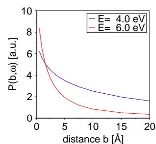
**Fig. 7.3:** delocalisation of the loss signal in graphene
