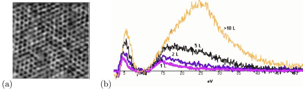
**Fig. 5.3:** (a) Annular dark field STEM image of a free-standing graphene sheet. (b) Experimental electron energy-loss spectra of one, two, five and many layers of graphene. Main features are the  $\pi$ - and  $\pi+\sigma$ -plasmon excitations at about 6 eV and 15–25 eV, respectively. Both figures are reproduced from [141], © 2008 by The American Physical Society.
