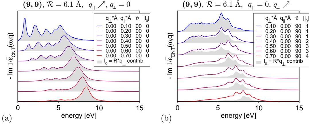
**Fig. 6.11:** Tight-binding calculations for the plasmon dispersion in the (9,9) nanotube. The loss function for several momentum transfers (a) parallel and (b) perpendicular to the tube axis are shown. The shaded area corresponds to the contribution of the  $l_0 = \lfloor q_{\perp} \mathcal{R} \rfloor$  mode in eq. (6.23).
