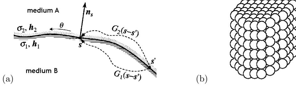
**Fig. 1.5:** (a) Boundary-element method (Reproduced from [41], © 2002 by The American Physical Society) and (b) discrete-dipole approximation. The balls indicate a single dipole.
