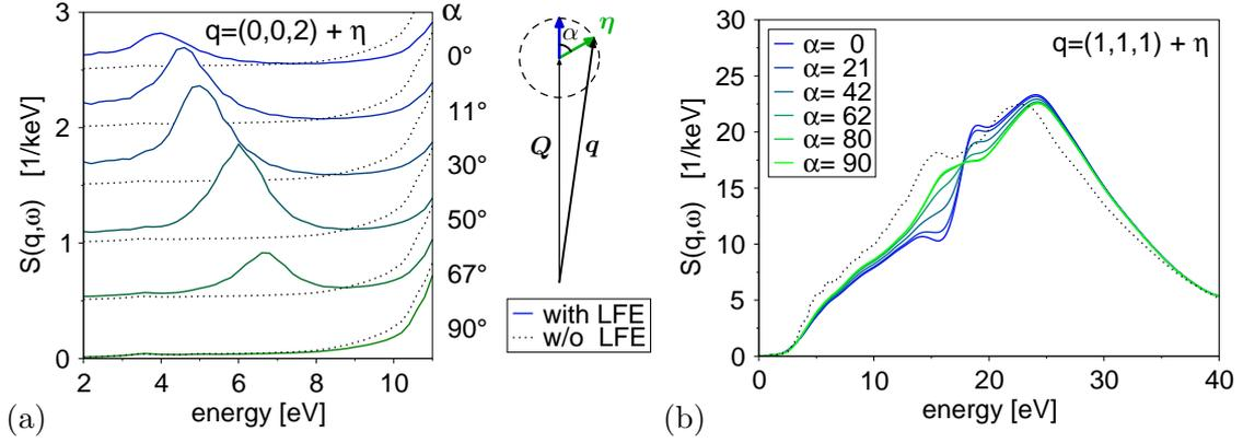
**Fig. 4.1:** Prediction of anisotropic behaviour of the dynamic structure factor  $S(\mathbf{q}, \omega)$  in the vicinity of a Bragg reflection (a)  $\mathbf{Q} = (0, 0, 2)$  for graphite and (b)  $\mathbf{Q} = (1, 1, 1)$  for silicon (see text). Spectra in (a) are shifted along the ordinate for better visibility.
