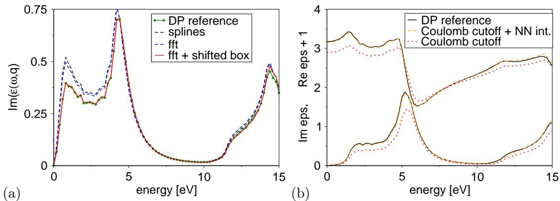
**Fig. C.4:** (a) Energy-loss function of a graphene stack with interlayer distance  $d = 16d_0$  and in-plane momentum  $\bar{q} = 0.07 \text{ \AA}^{-1}$ . (b) Loss function for a graphene stack with  $d = 4d_0$  and in-plane momentum  $\bar{q} = 0.27 \text{ \AA}^{-1}$ . See text for further details.
