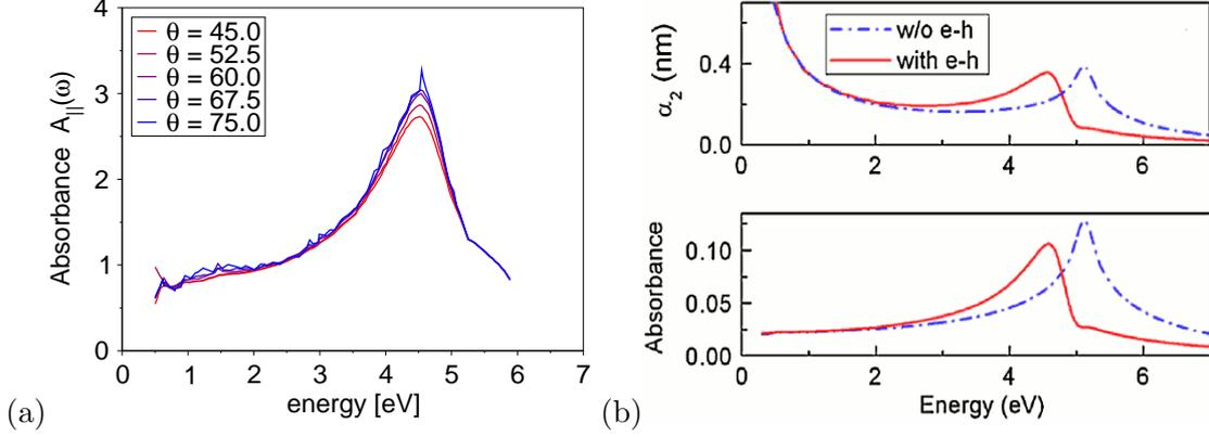
**Fig. 6.15:** Decomposition for the X-ray absorption measurements on isolated nanotubes of Murakami *et al.* [161]. We compare (a) the on-axis contribution  $A_{||}$  to the absorbance of the tubes which is calculated from the experimental data shown in fig. 6.3a with (b) the absorbance of graphene obtained from a Bethe-Salpeter calculation by Yang *et al.* [159] (Reproduced from [159], © 2009 by The American Physical Society).
