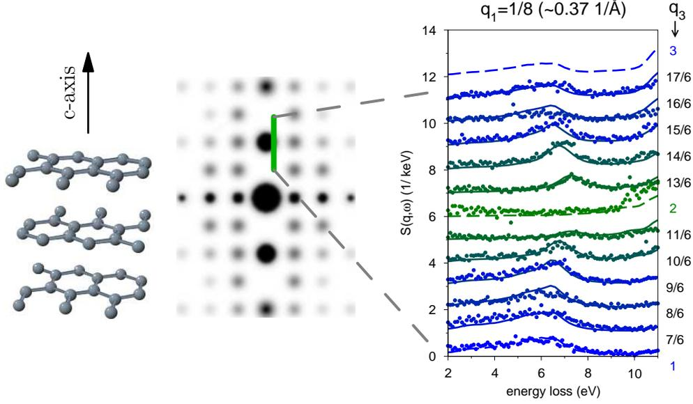
**Fig. 4.7:** Comparison of the structure factor  $S(\mathbf{q}, \omega)$  measured by IXS-experiments (dots) and calculated in RPA (lines; dashed for integer  $q_3$ ) for  $\mathbf{q} = (\frac{1}{8}, 0, q_3)$ . The position of the momentum transfer in reciprocal space is indicated on the left. The elastic tail has been removed from the raw experimental data and a uniform scaling has been applied.
