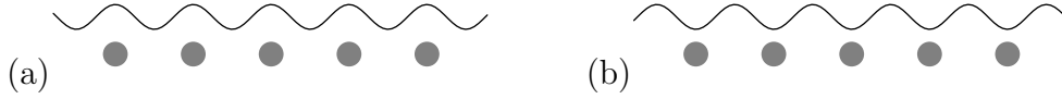
Fig. 2.3: Probability density |\phi(\mathbf{s})| of the incident electron in the two-beam case (2.19) for k_i - k'_i = 2\pi/a and a phase shift (a) \varphi = 0 and (b) \varphi = \pi . The origin is at the first atom.
