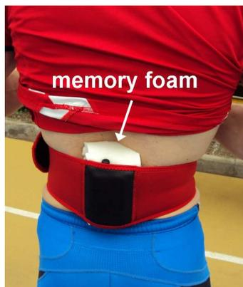
**Figure 3:** Belt and sensor unit location on the lower back trunk of an elite athlete of group B. Indication of the memory foam material location is also provided.
