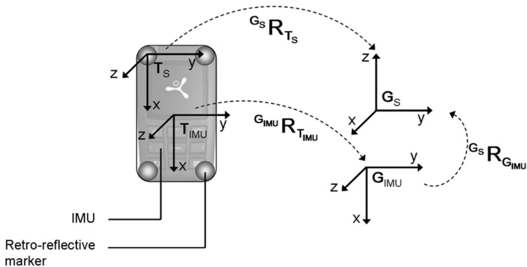
**Figure 2 (3.2):** Technical (T) and Global (G) frames for the inertial sensor (IMU) and the stereophotogrammetric system (S).
