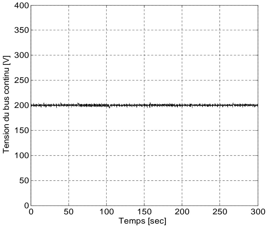
Figure 2.32 Tension de bus continu DC
