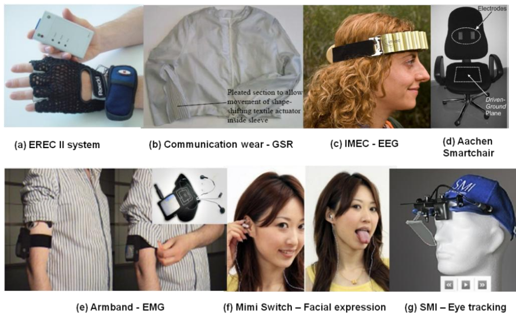
Figure 45. Examples of new physiological sensors in HCI
