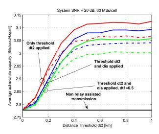
Figure 6.10: Sum-rate versus distance threshold  $d_{t2}$  for different versions of Algorithm 6 (threshold  $d_{t2}$  is always applied). Solid lines: DF, Dashed lines: AF.
