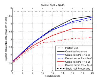
Figure 4.8: Digital Feedback: Sum-rate versus the number of feedback bits (System SNR = 10 dB). Blue curves:  $P_e = 10^{-3}$ , Red curves:  $P_e = 10^{-2}$ . 'Cent': centralized framework, 'Decent': decentralized framework.
