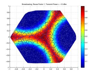
Figure 7.4: Probability of Sensor Inactivity in the areas of the sensing field for the case of Reuse Factor 1 Schedule Broadcast Transmission.
