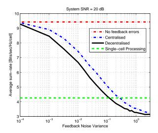
Figure 4.7: Analog Feedback: Sum-rate versus the feedback error noise variance for the decentralized and the centralized framework.
