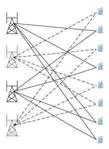
Figure 3.1: A graph representation of the case of 4 BSs with 2 antennas each.
