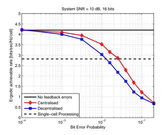
Figure 4.10: Digital Feedback: Sum-rate versus bit error probability for both frameworks (System SNR = 10 dB, 16 bits employed).
