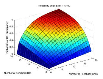
Figure 4.5: Probability of CSI discrepancy versus the number of feedback links and feedback bits  $(P_e = 10^{-3})$ .
