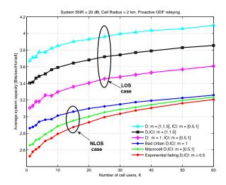
Figure 6.1: System capacity versus the number of cell users (ODF proactive relaying, System  $\rm SNR=20~dB)$  under different fading conditions.
