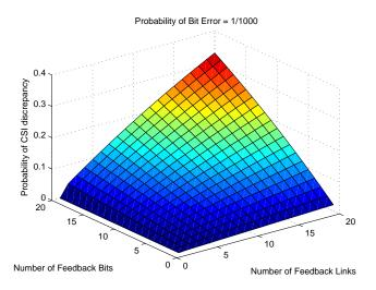
Figure 4.6: Probability of CSI discrepancy versus the number of independent links and feedback bits ( $P_e = 10^{-2}$ ).
