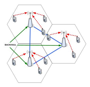
Figure 1.1: The MCP overheads. Red dashed lines represent feedback overhead, green lines represent backhaul overhead and blue lines infrastructural overheads (CSI exchange).
