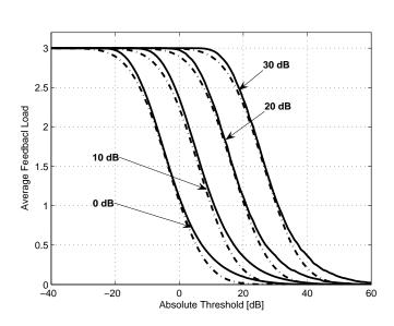
Figure 5.3: Average feedback per MS versus threshold for different values of system SNR (0 dB, 10 dB, 20 dB, 30 dB). Theoretical results are shown by the dashed lines and numerical ones by the solid ones.
