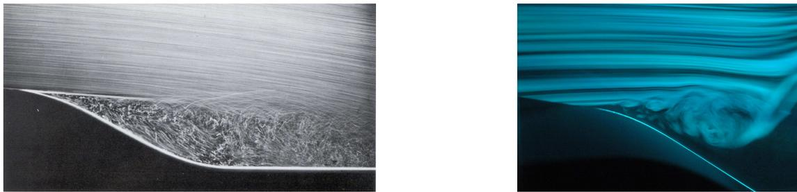
Figure 5: Left: laminar separation from a curved wall in a water tunnel. The flow is visualized by air bubbles and the Reynolds number based on the leading edge (not shown) is 20 000. ONERA picture, H. Werlé (1974). Right: Separated flow observed at the S19Ch wind tunnel of ONERA (2005). The flow is visualized by laser tomography.
