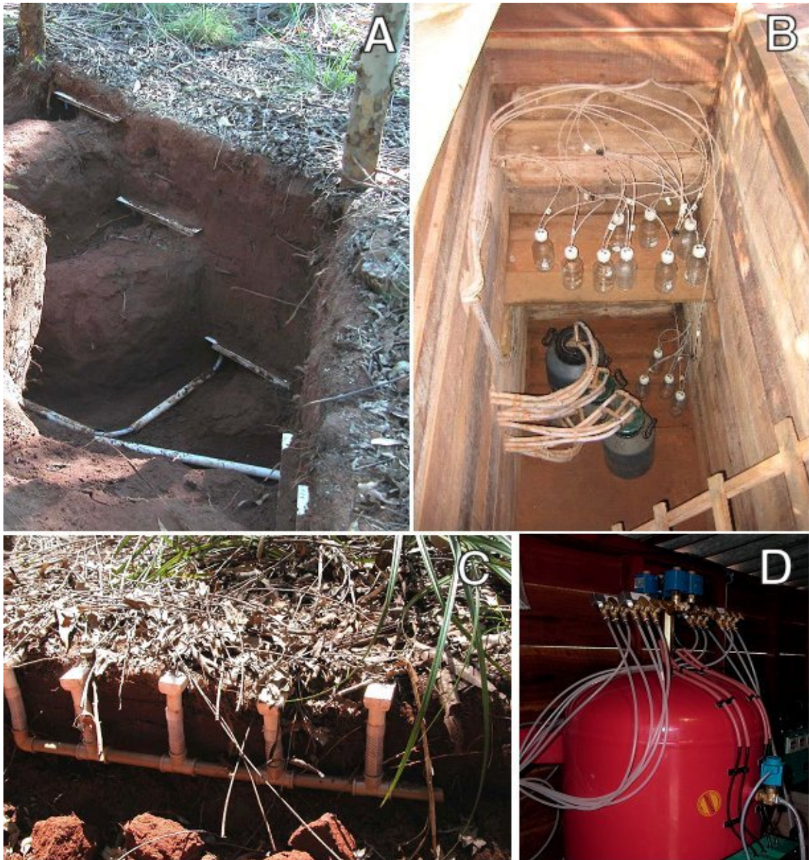
Figure 51 Soil solution sampling equipments: zero-tension lysimeters in soils (A) and under the forest floor (C), pit where soil solutions were kept in the field (B) and pump used to maintain vacuum in tension lysimeters (D).
