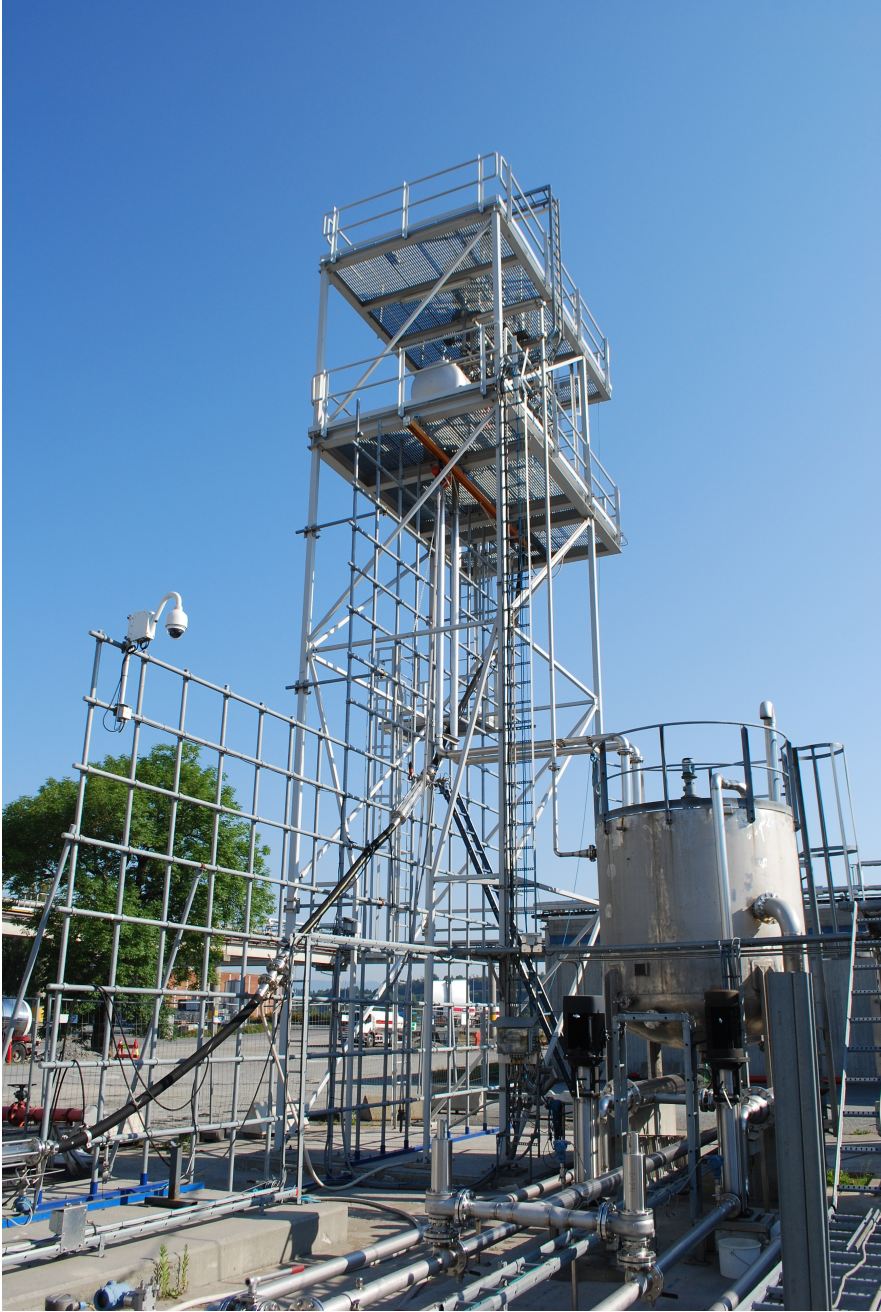
Figure 3.3: Picture of the rising section of the experimental multiphase flow loop MaS-CoT.
