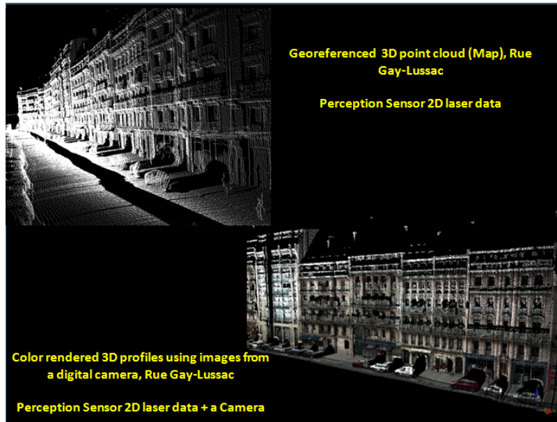
Figure 3.4: LARA-3D results - 3D point clouds generated from laser scanner measurements, and textured using the digital image
