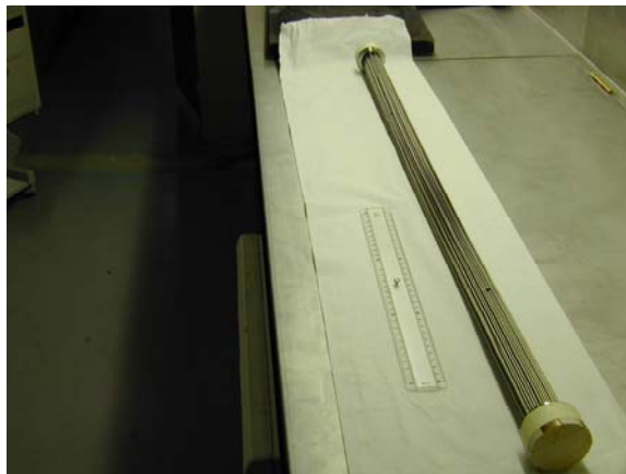
c. A unit of the gas cooler.
