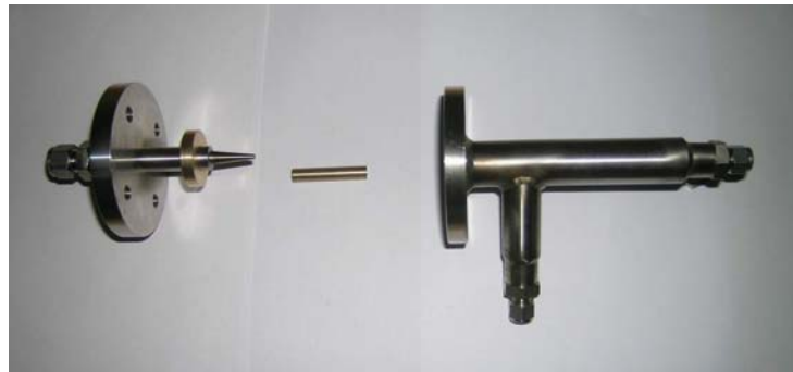
Assembly scheme of the ejector parts
