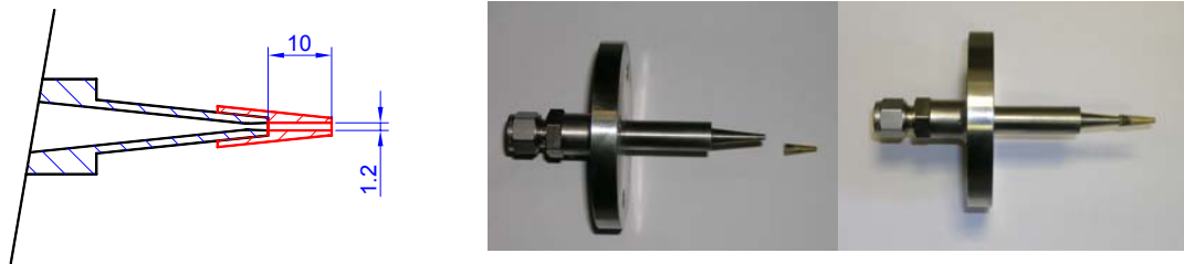
a. Scheme of the modified nozzle
