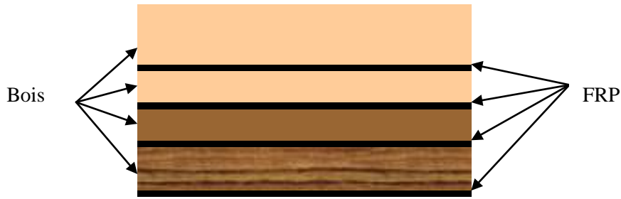
Figure 3.2. Renforcement multi lamé
