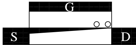
Figure 2.1: Interface traps in MOS structure under HCI degradation: illustration.
