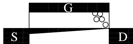
Figure 2.3: Aligned defaults in post-breakdown MOS structure: illustration.
