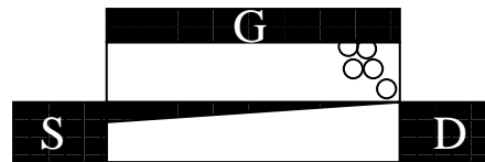
Figure 2.3: Aligned defaults in post-breakdown MOS structure: illustration.
