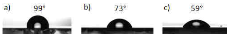
Figure 39 – Static water contact angle of a) pristine, b) spontaneously grafted and c) \text{H}_3\text{PO}_2 -induced grafted with NBDT gold substrates.
