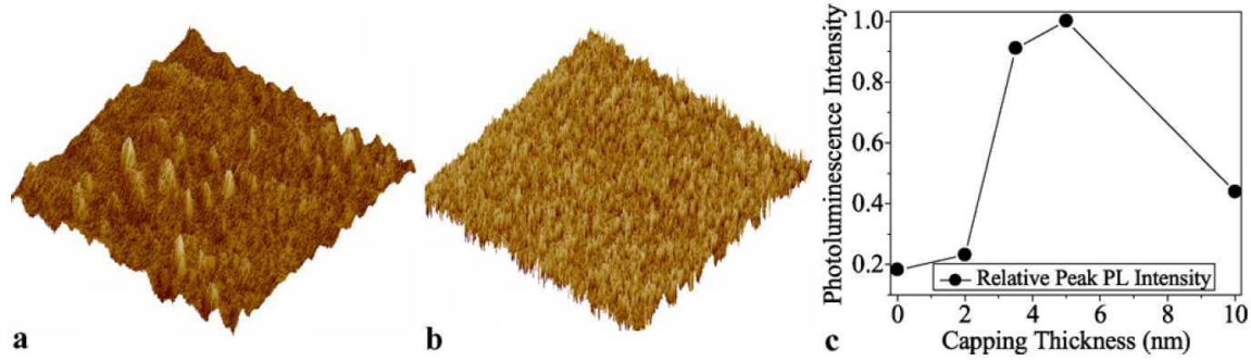
Figure 52. AFM Surface Plot for (a) 2 nm capped ( 1 \mu\text{m} \times 1 \mu\text{m} ), (b) 5 nm capped ( 5 \mu\text{m} \times 5 \mu\text{m} ) 4.4 ML InGaN QDs. (c) Peak photoluminescence intensity dependence on capping thickness.
