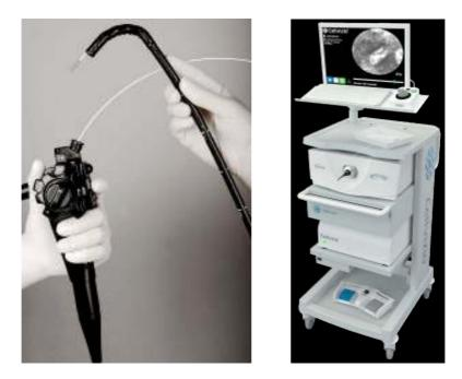
Figure 1.1: Left: pCLE miniprobe inserted through the working channel of a standard endoscope. Right: Setup of pCLE imaging system (Cellvizio, Mauna Kea Technologies).
