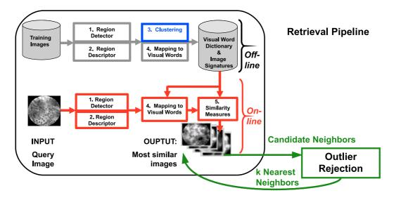
Figure 2.11: Overview of the retrieval pipeline followed by a the geometrical verification process performing outlier rejection.
