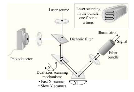
Figure 2.3: Physics of acquisition for pCLE imaging.
