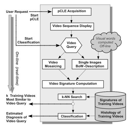
Figure 3.4: Pipeline of the pCLE retrieval-based classification framework, from the acquisition of the pCLE video query by the Cellvizio system to the online automated diagnosis estimation.
