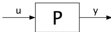
Figure 2.1: A linear time invariant system P with input \mathbf{u} and output \mathbf{y} .
