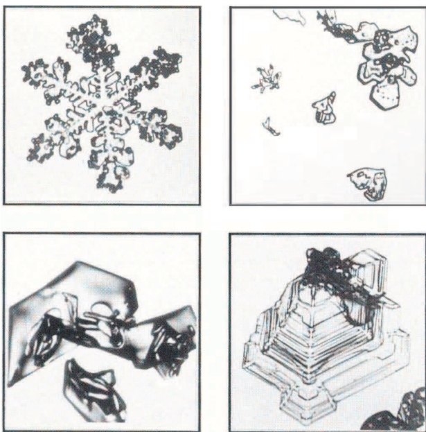
Fig. 2. Examples of grains collected from natural snowpacks and observed after several weeks' storage in cold iso-octane.
