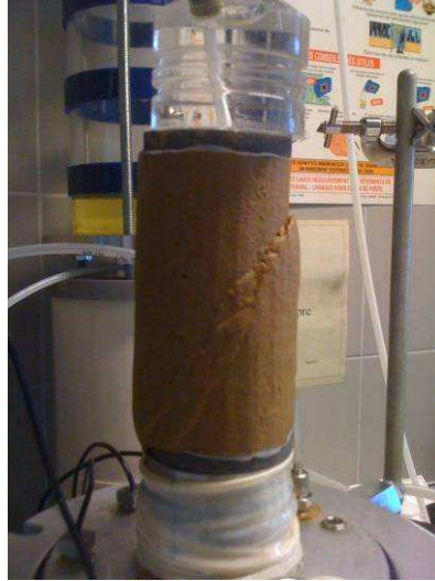
Figure 8. Shear plane in the shear triaxial test at water content of 10.6%
