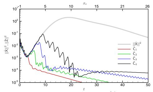
FIGURE 6. Temporal evolution of the energy of the error vector  $\|\hat{Z}\|^2$  for four different sensor locations  $\hat{C}_{1,2,3,4}$ , and energy of the (uncontrolled) state  $\|\hat{X}\|^2$  (in gray).
