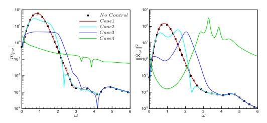
FIGURE 11. (a) Magnitude of the transfer function  $|m_{pw}|$  for four different (G/W, l)-parameter settings, as well as the uncontrolled case. (b) Transfer function between noise and global energy for the same four parameter settings.
