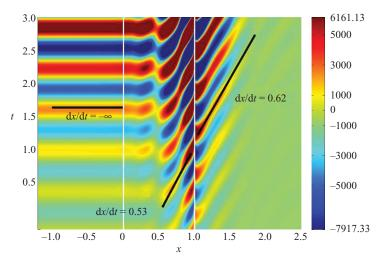
FIGURE 3. Spatio-temporal x-t diagram of pressure p(x, y=0, t) contours with no control applied. The initial condition corresponds to the most unstable global mode. The two vertical white lines indicate the cavity walls. See also movie I in the online version of the paper.
