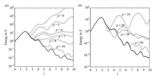
FIGURE 16. Performance of partial-state controller measured as the perturbation kinetic energy versus time for different reduced-order models. (a) The number of included BPOD modes (in addition to the unstable global modes) is denoted by p. (b) The number of included POD modes (in addition to the unstable global modes) is denoted by p.
