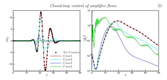
FIGURE 12. (a) Measurement signal at  $\hat{C}_p$  for four selected (G/W, l)-parameter settings. (b) Temporal evolution of the global perturbation energy for the same parameters.
