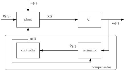
FIGURE 3. Sketch of a typical LQG-control setup.
