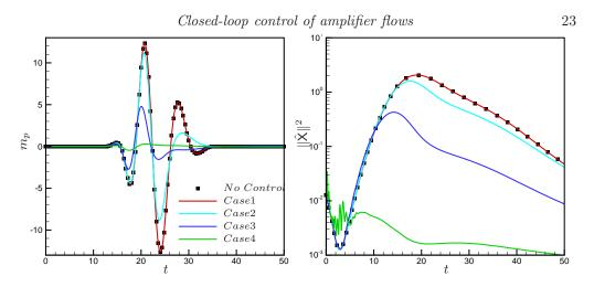
FIGURE 15. (a) Measurement signal at  $\hat{C}_p$  for four selected (G/W, l)-parameter settings. (b) Temporal evolution of the global perturbation energy for the same parameters.
