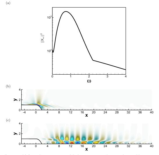
FIGURE 2. (a) Optimal energy response of the linear system to a harmonic forcing of frequency  $\omega$ . (b) Optimal forcing visualized by contours of the streamwise velocity. (c) Optimal response visualized by contours of the streamwise velocity.
