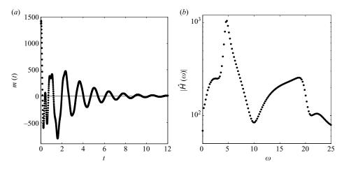
FIGURE 4. Impulse response (a) as a function of time and transfer function (b) as a function of frequency for the stable part of the flow over an open cavity at Re = 7500.
