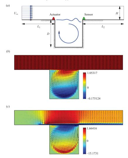
FIGURE 1. (a) Sketch of the geometry for flow over a square cavity. (b) Base flow, visualized by streamwise velocity contours and velocity vectors, for a Reynolds number of Re = 7500. (c) Inhomogeneous solution **C** with a unit force at the actuator location, visualized by streamwise velocity contours and velocity vectors.
