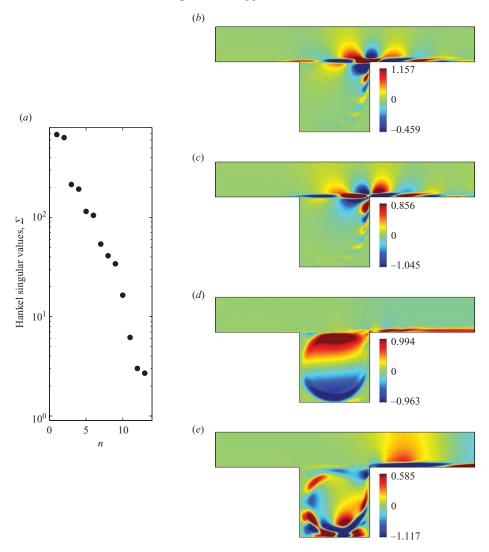
FIGURE 8. (a) Hankel singular values for flow over a square cavity for Re = 7500. (b-e) Balanced proper orthogonal decomposition (BPOD) modes. (b) First, (c) second, (d) ninth and (e) thirteenth mode, visualized by the streamwise velocity.
