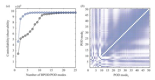
FIGURE 13. (a) Controllability/observability of a BPOD (blue) and POD (black) projection basis. (b) Observability measure of a POD basis according to criterion (5.27).
