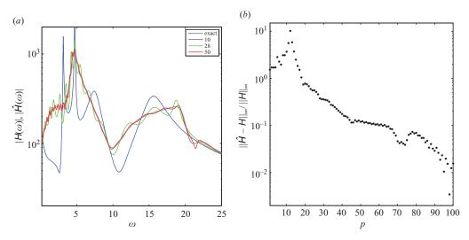
FIGURE 12. (a) Comparison of transfer function of the reduced-order model to the exact transfer function for a projection basis consisting of p = 10, 28, 50 POD modes. (b) Relative  $\mathscr{H}_{\infty}$ -error norm as a function of the number p of included POD modes.
