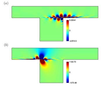
FIGURE 4. Selected direct and adjoint global modes for flow over an open cavity at Re = 7500. (a) Most unstable direct global mode, (b) adjoint global mode associated with the most unstable direct global mode in (a). Both modes are visualized by contours of the streamwise velocity component.
