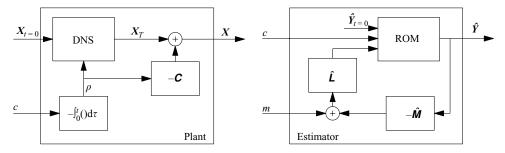
FIGURE 14. Block diagrams for the DNS module (plant) based on (2.8) and the estimator module based on a reduced-order model (ROM) described by (6.4).
