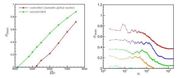
FIGURE 2.6 – left : growth rate  $\sigma_{max}$  of the least stable mode of the compensated system versus the Reynolds number. The ROM is only composed of unstable global modes. Right : growth rate  $\sigma_{max}$  of the least stable mode of the compensated system versus the number of stable global modes included in the ROM. The modes are ranked according to the criterion  $\Gamma$ . The different curves correspond from top to bottom to Re=7500, Re=7000, Re=6500, Re=6000 and Re=5500.
