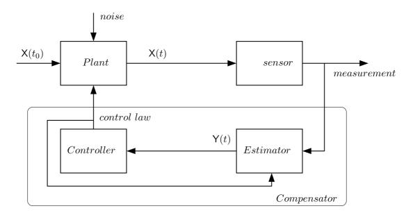
FIGURE 1.5 – Sketch of a typical Linear Quadratic Gaussian control setup.
