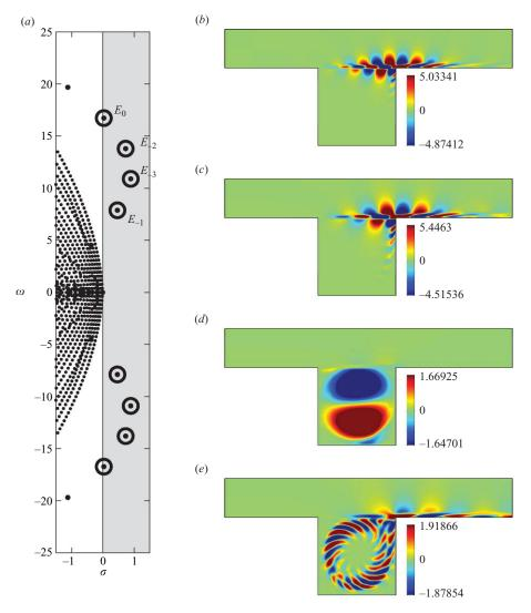
FIGURE 2. (a) Part of the global spectrum for flow over a square cavity at Re = 7500, showing four unstable global modes (marked by circles and labelled  $E_{-3}$ ,  $E_{-2}$ ,  $E_{-1}$ ,  $E_0$ ) and their symmetric counterparts. (b-e) Direct global modes corresponding to  $E_{-3}$  (b),  $E_{-1}$  (c),  $E_1$  (d) and  $E_2$  (e). The global modes are visualized by their streamwise velocity component.
