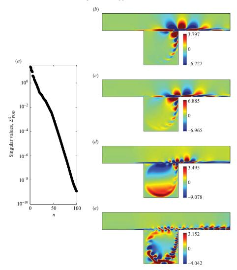
FIGURE 11. (a) Singular values for POD modes. (b-e) POD modes for flow over an open square cavity at Reynolds number Re = 7500. The (b) first, (c) second, (d) third and (e) twenty-eighth POD modes are visualized by their streamwise velocity component.
