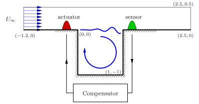
FIGURE 1. Sketch of flow over an open cavity.
