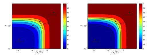
FIGURE 13. (a) Contours of the performance measure  $P_m$  based on the measurement energy as a function of noise-to-signal ratio G/W and control cost parameter l for sensor  $\hat{C}_1$ . (b) Contours of the performance measure  $P_e$  based on the global perturbation energy as a function of noise-to-signal ratio G/W and control cost parameter l for sensor  $\hat{C}_1$ .
