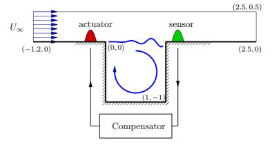
FIGURE 2.1 – Sketch of flow over an open cavity.
