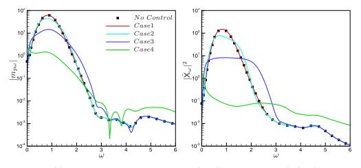
FIGURE 14. (a) Magnitude of the transfer function  $|m_{pw}|$  for four different (G/W, l)-parameter settings, as well as the uncontrolled case. (b) Transfer function between noise and global energy for the same four parameter settings.
