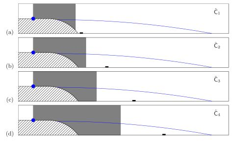
FIGURE 8. Sketch of regions of the flow domain where disturbances cannot be detected by the sensor: (a) for sensor  $\hat{C}_1$ , (b) for sensor  $\hat{C}_2$ , (c) for sensor  $\hat{C}_3$ , and (d) for sensor  $\hat{C}_4$ . The location of  $\hat{B}_1$  is indicated by a blue symbol; the respective sensor location is shown as a black rectangle.
