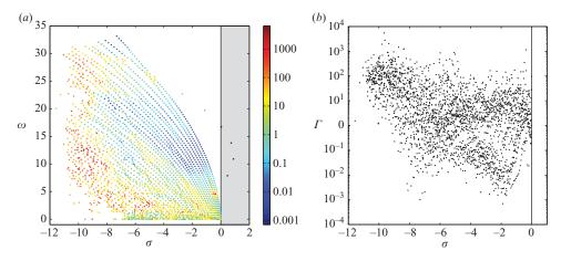
FIGURE 6. (a) Global spectrum of flow over an open square cavity at Re = 7500 colour-coded by  $\Gamma_i$ , a measure of each global mode's contribution to the input–output relation (see (5.8) and text for explanation). (b) Criterion  $\Gamma_i$  versus the each mode's amplification rate.
