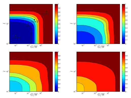
FIGURE 9. Contours of the performance measure  $P_m$  based on the measurement energy as a function of noise-to-signal ratio G/W and control cost parameter l. Top left: sensor  $\hat{C}_1$ , top right: sensor  $\hat{C}_2$ , bottom left: sensor  $\hat{C}_3$ , bottom right: sensor  $\hat{C}_4$ .
