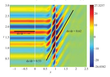
FIGURE 17. Spatio-temporal x-t diagram of pressure p(x, y = 0, t) contours with "best control strategy" applied. The initial condition consists of the most unstable global mode. The two vertical white lines indicate the cavity walls. See also movie II in the online version of the paper.
