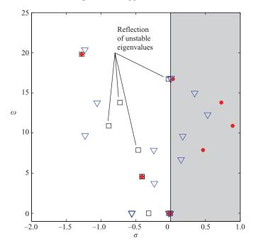
FIGURE 19. Global spectrum of the compensated system for p = 0 (triangles) and p = 13 (squares). Red dots correspond to the uncontrolled plant, i.e. eigenvalues of  $\hat{A}_{n,\tilde{n}}$ .
