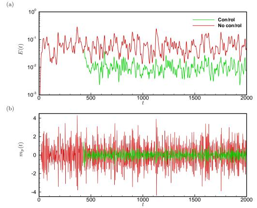
FIGURE 19. Temporal evolution of the energy based on a linearized numerical simulation continuously forced by random noise. The compensator has been designed under linear assumptions based on the  $ROM_{150}$  model (case 3). (a) Perturbation energy for the uncontrolled (red) and controlled (green) case, (b) measurement energy for the uncontrolled (red) and controlled (green) case.
