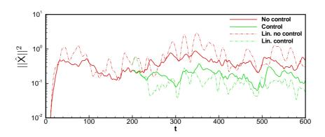
$\label{eq:Figure 2.10-Energy of the perturbations versus time. Thick curves : strongly non-linear simulations, dashed curves : linear simulations (same random sequence).$
