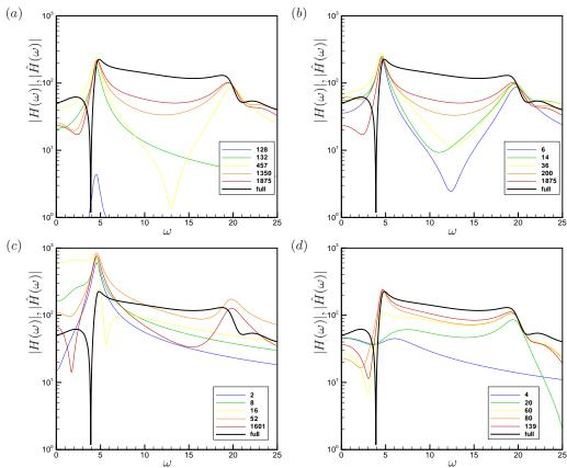
FIGURE 7. Approximation of the modulus of the exact transfer function (in black) as global modes are added to the reduction basis V according to the four selection criteria; (a) adding modes based on damping rate, (b) adding modes according to their contribution to the input-output behavior, (c) adding modes using orthogonal projections, (d) adding modes based on the "quasi-optimal" stability ranking. The Reynolds number is Re = 7500.
