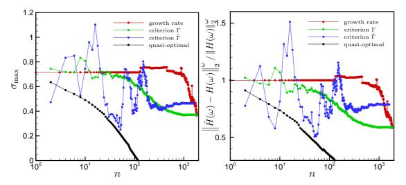
FIGURE 2.5 – left : growth rate  $\sigma_{max}$  of the least stable mode of the compensated system versus the number n of stable global modes included in the ROM. Right : relative frequency-restricted  $\mathcal{H}_2$  norm of the error between the full system and the ROM versus the number n of stable global modes included in the ROM.
