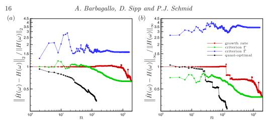
FIGURE 8. Relative approximation error of the full transfer function as global modes are added to the reduction basis V according to the four criteria (see text). (a) Relative error measure in the  $\mathcal{H}_2$ -norm, (b) relative error measured in the  $\mathcal{H}_\infty$ -norm. The Reynolds number is Re = 7500.
