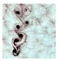
FIGURE 1.1 – Left : cigarette smoke subject to buoyancy effects. After Perry & Lim [75]. Right : Von Karmann vortex street in the atmosphere triggered by the flow over an island. (NASA picture).
