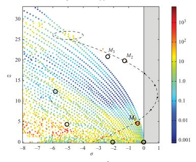
FIGURE 10. Eigenvalues of the reduced matrix  $\hat{A}_{\tilde{p},\tilde{p}}$  superimposed on the global spectrum of the cavity. Eight unstable global modes and 13 BPOD modes have been included in the reduced model. The global spectrum is coloured according to the criterion  $\Gamma_i$ .
