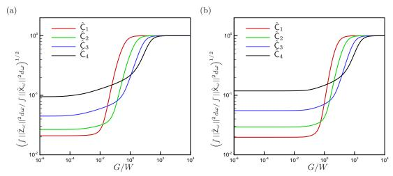
FIGURE 5. Normalized performance of the estimator, integrated over all frequencies, versus the estimation parameter G/W for four different sensor locations; (a) measuring shear-stress, (b) measuring pressure.
