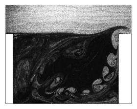
FIGURE 1.3 – Supercritical flow over an open cavity at  $Re_L = 11\,150$  (aspect ratio H/L = 1.5). After Basley et al. [13].
