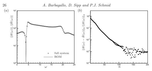
FIGURE 15. (a) Magnitude of the transfer function of the full system (symbols) and the reduced-order mode based on POD modes (solid line). (b) Relative  $\mathcal{H}_2$ -error of the transfer function of the reduced-order plant model based on n POD modes.
