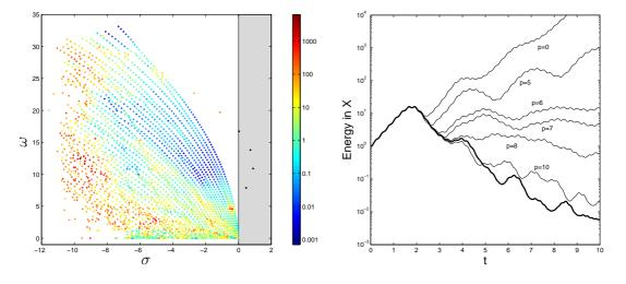
FIGURE 2.2 – left : global spectrum of the cavity flow at Re = 7500,  $\sigma$  is the damping rate and  $\omega$  the frequency. Right : energy of the perturbations in the compensated system for ROMs based on the unstable global modes and p BPOD modes (thin curves) and "best control strategy" (thick curve).
