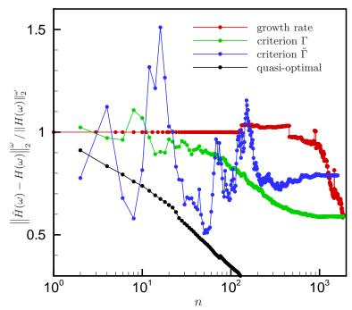
FIGURE 10. Relative approximation error of the reduced-model transfer function as global modes are added to the reduction basis V according to the four criteria (see text). The relative error is measure in the frequency-restriced norm  $\mathcal{H}_{2}^{\omega}$ . The Reynolds number is Re = 7500.
