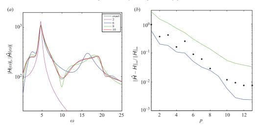
FIGURE 9. (a) Comparison of transfer function of the reduced-order model to the exact transfer function for a projection basis consisting of p = 2, 6, 8, 10 balanced modes. (b) Relative  $\mathscr{H}_{\infty}$ -error norm as a function of the number p of included balanced modes, together with an upper (green line) and lower bound (blue line) on the error.
