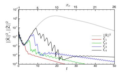
FIGURE 2.8 – Energy of the error vector  $||\hat{Z}||^2$  versus time color coded by the sensor considered, energy of the (uncontrolled) state  $||\hat{X}||^2$  (in gray).
