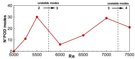
FIGURE 14. Minimum number of proper orthogonal decomposition (POD) modes to stabilize the compensated system consisting of a reduced model based on unstable global modes and POD modes. At critical values of the Reynolds number (indicated by dashed lines) additional global modes become unstable.
