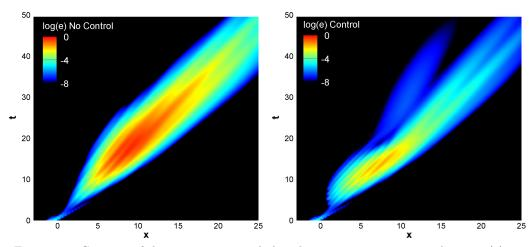
FIGURE 18. Contours of the energy integrated along lines x = const. in an *x*-*t*-diagram. (a) Uncontrolled linearized simulation; (b) compensated linearized simulation (case 3).
