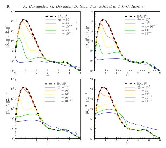
FIGURE 4. Performance of the estimator versus frequency using four different sensors and selected values of the estimation (noise-to-signal) parameter G/W. Top left: sensor  $\hat{C}_1$ , top right: sensor  $\hat{C}_2$ , bottom left: sensor  $\hat{C}_3$ , bottom right: sensor  $\hat{C}_4$ .
