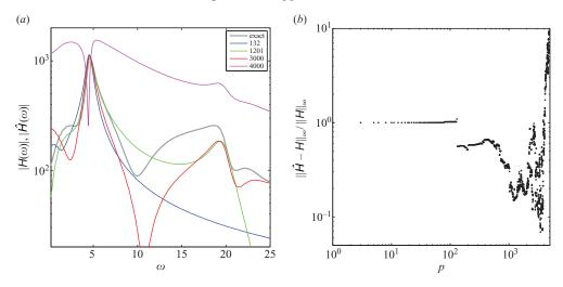
FIGURE 5. (a) Comparison of transfer function of the reduced-order model to the exact transfer function for a projection basis consisting of p = 132, 1201, 3000, 4000 stable global modes. (b) Relative  $\mathscr{H}_{\infty}$ -error norm as a function of the number p of included stable global modes.
