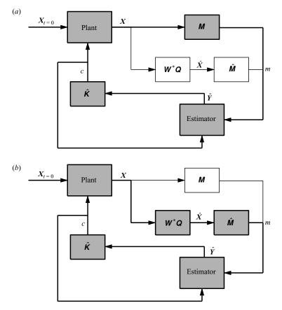
FIGURE 15. Block diagrams demonstrating (a) partial-state information control and (b) 'best control strategy'. Only the shaded blocks and the thick lines are active in each diagram. The details of the plant and estimator blocks are given in figure 14.
