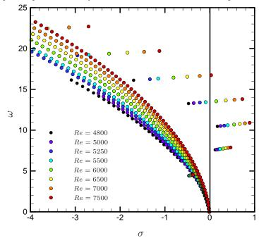
FIGURE 11. Changes in the global spectrum of flow over an open cavity as the Reynolds number is varied from Re = 4800 to Re = 7500.
