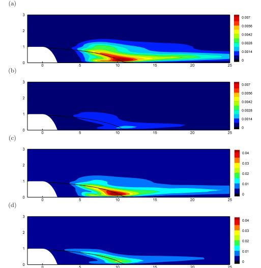
FIGURE 23. Pointwise mean perturbation energy of simulations with random forcing. (a) Uncontrolled direct numerical simulation for W = 1. (b) Compensated direct numerical simulation for W = 1 (case 3). (c) Uncontrolled direct numerical simulation for  $W = \sqrt{10}$ . (d) Compensated direct numerical simulation for  $W = \sqrt{10}$  (case 3).
