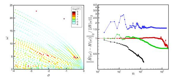
FIGURE 2.4 – left : global spectrum colored by criterion  $\Gamma$ . Right : relative  $\mathcal{H}_2$  norm of the error between the full system and the ROM versus the number n of stable global modes included in the ROM (see legend on figure 2.5(left)).
