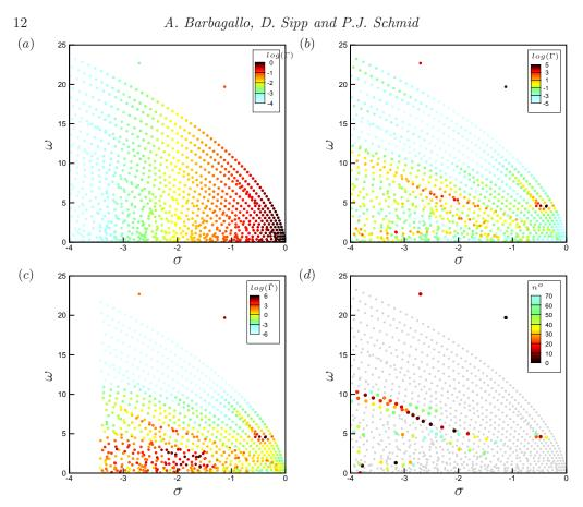
FIGURE 6. Identification of global modes by color-coding according to the four respective criteria (see text): (a) growth rate, (b) contribution to input-output behavior, (c) orthogonal projection, and (d) "quasi-optimal" stability ranking. Only the stable part of the spectrum is displayed; the Reynolds number is Re = 7500.
