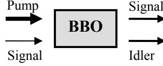
Figure 2.4 Principle of optical parametric amplification.
