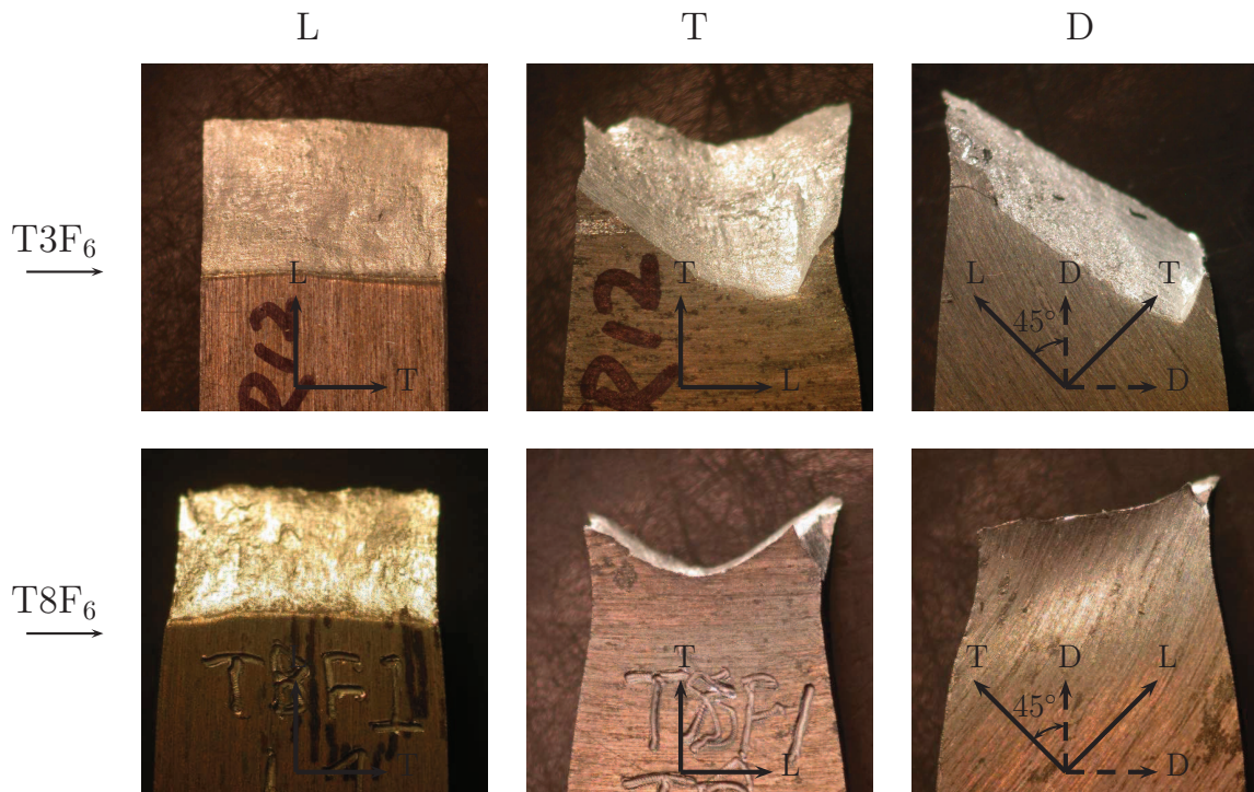
Figure 3.14: Post-test specimens of smooth flat tensile tests along L-, T- and D-loading for 6 mm thick fibrous materials.
