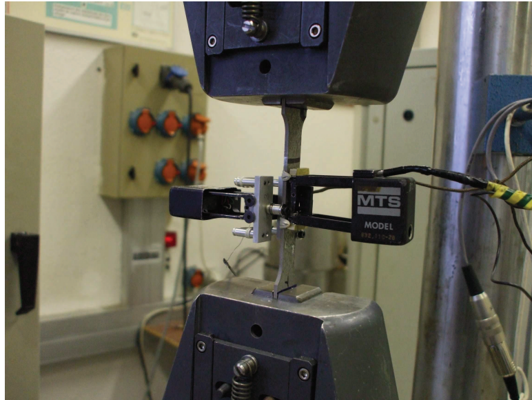
Figure 3.2: Smooth flat tensile specimen ST 12 setup with longitudinal and transverse gages during test.
