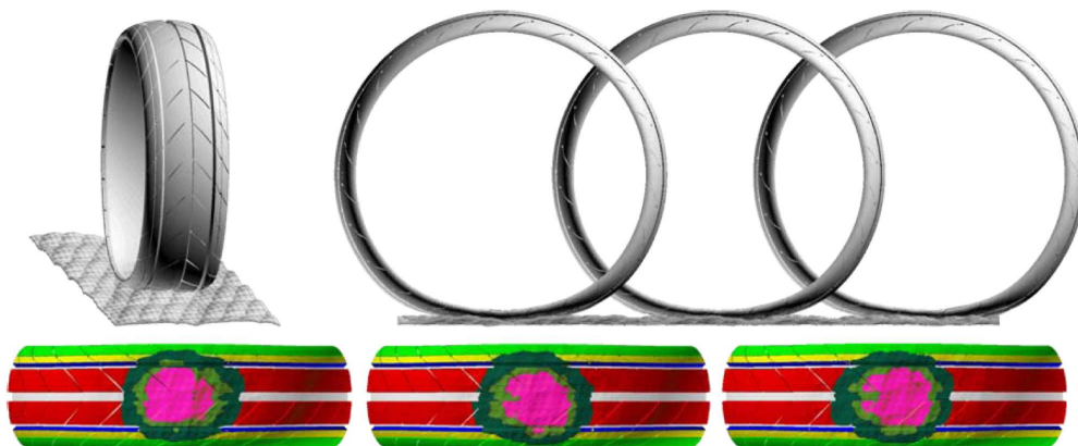
Figure 3.14: Tire-road contact problem: general view, three tire-road dispositions and corresponding contact elements on the bottom of the tire for different imprint configurations.
