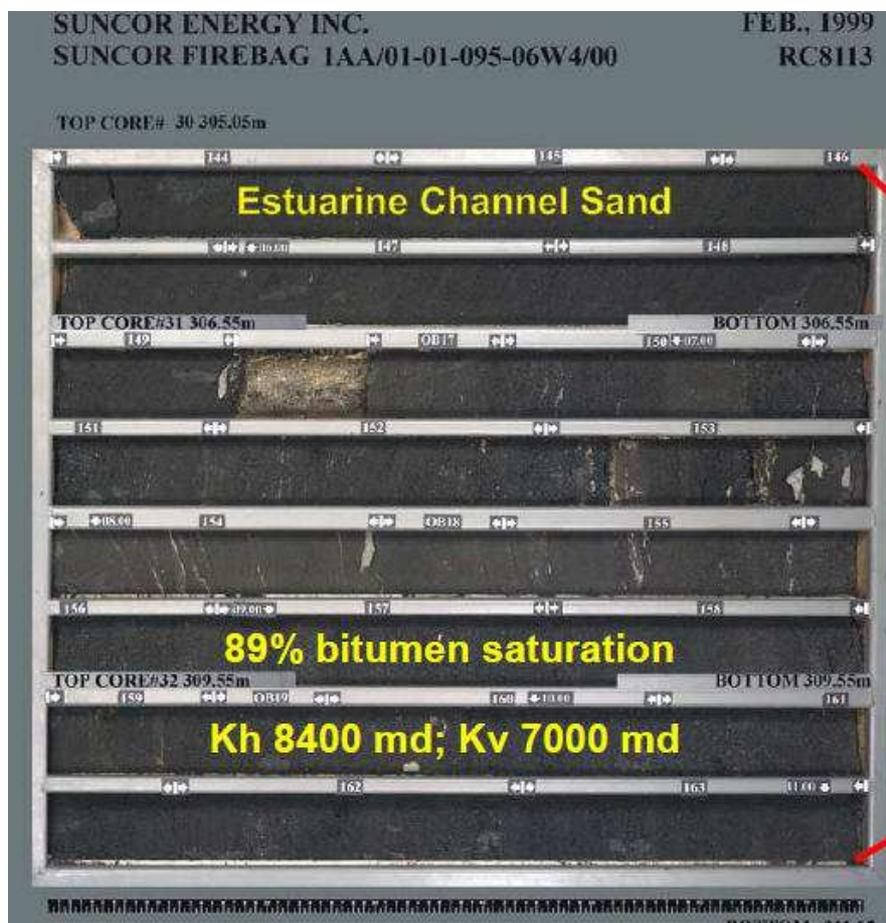
Figure I-4. Sable bitumineux de formation McMurray (Suncor, projet de Firebag) ([www.ercb.ca/docs/products/.../2005AthabascaSuncorFirebagSAGD8870.pdf](http://www.ercb.ca/docs/products/.../2005AthabascaSuncorFirebagSAGD8870.pdf)).
