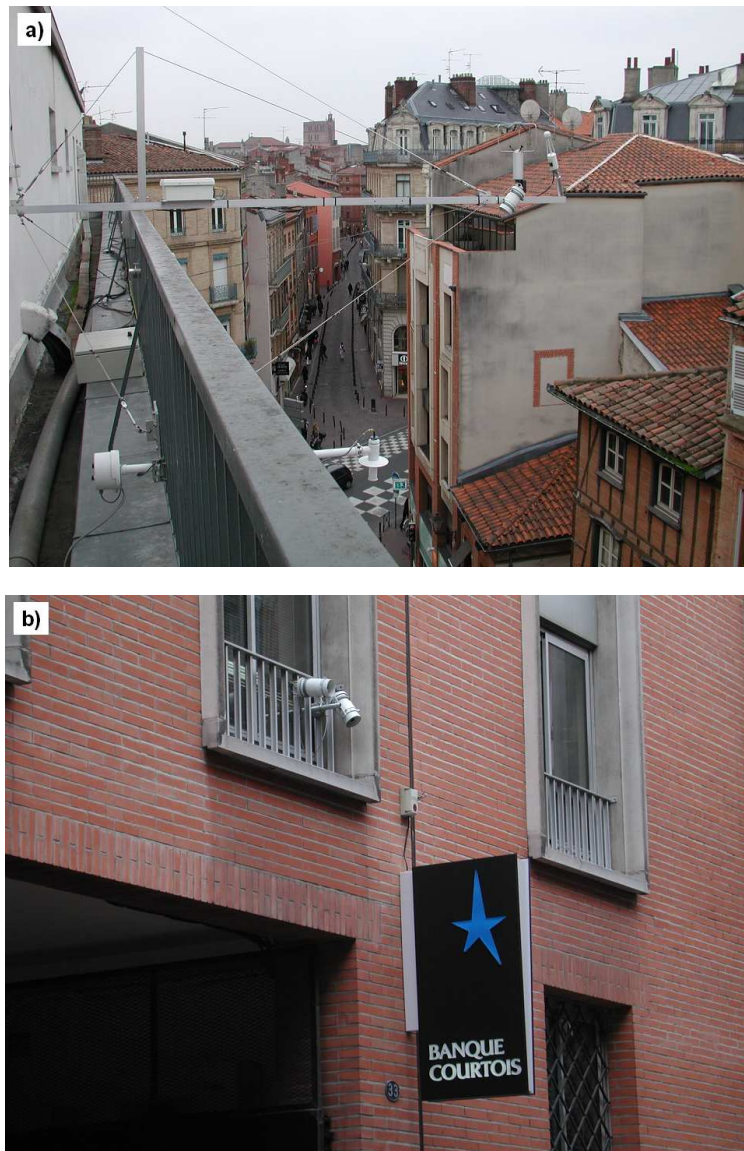
Figure 6.2: Photo of the affixed IRTs: a) an IRT mounted on a boom in the Alsace canyon; b) IRTs mounted on a railing in the Remusat canyon, one is directed toward the wall across the street and the other to the road below. Source Pigeon (2004).
