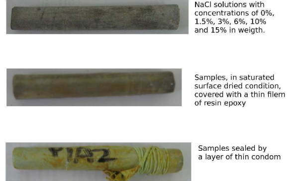
Figure 9.2: Preparation procedures of saturated cylindrical samples to obtain an undrained condition during freeze-thaw tests.
