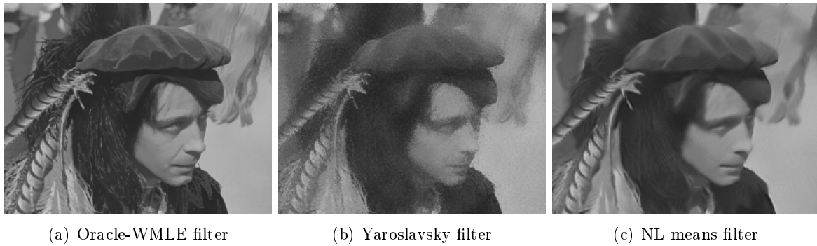
Figure 5.3: Denoising results obtained by (a) the oracle-WMLE, (b) the Yaroslavsky filter and (c) the NL means filter on a noisy image damaged by additive white Gaussian noise. The result obtained by the Yaroslavsky suffers from a strong residual noise which has been reduced properly by NL means. The NL means filter reaches performance challenging the oracle-WMLE.
