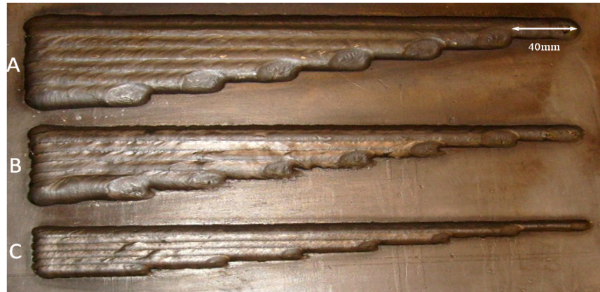
Figure 3.32: Single layer clad strategy for selected parameters at 40% overlapping
