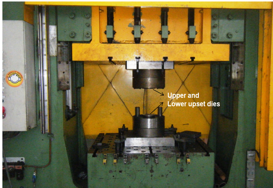
Figure 4.64: Setup for the experimental upsetting test
