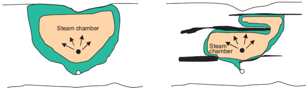
Fig. 3.11: Left: steam chamber development in a homogeneous reservoir. Right: steam chamber development in a reservoir with shale baffles of limited extent.
